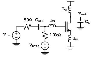
c) Assume this amplifier is loaded by an identical FET, therefore  $C_L = C_{gs}$ . Calculate the value of  $L_D$  required to resonate out this capacitance at 1GHz. Is this a reasonable value?
