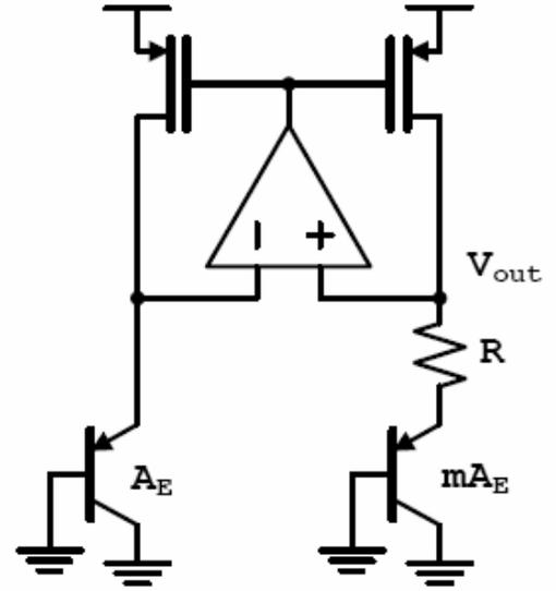
$$V_{BE1} = V_{BE2} + I_C R$$
