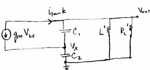
$$V_{be} = -V_x = -V_{out} \left( \frac{C_1}{C_1 + C_2} \right)$$
