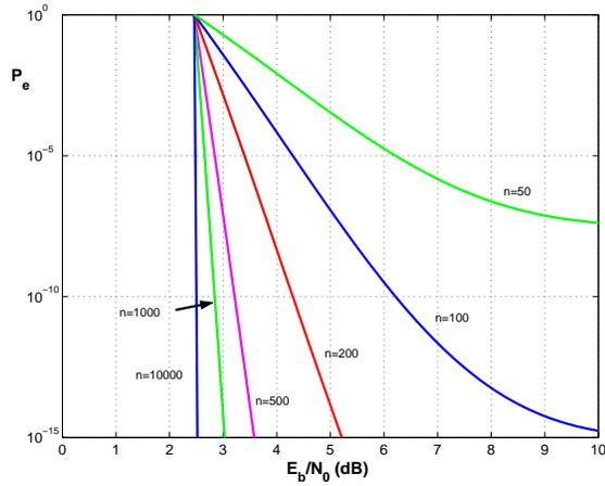
Figure 11: Error Probabilities Based on Cutoff Rate for Binary Input-Continuous Output Channel for Rate 1/2 codes
