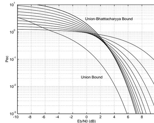
Figure 15: Comparison of Gallager Bound, Union Bound and Union Bhattacharyya Bound for the Hamming Code with BPSK Modulation
