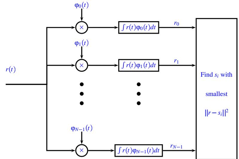
Figure 9: Optimum Receiver in Additive White Gaussian Noise
