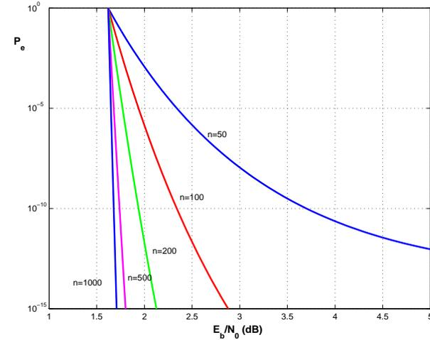
Figure 12: Error Probabilities Based on Cutoff Rate for Binary Input-Continuous Output Channel for Rate 1/8 codes
