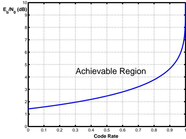
Figure 14: Cutoff Rate for Binary Input-Continuous Output Channel
