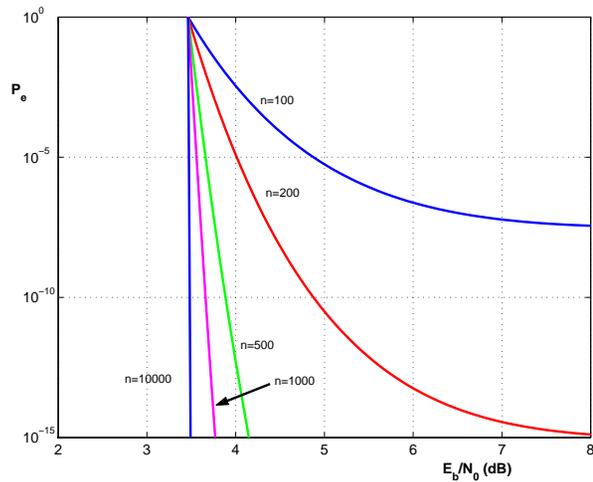
Figure 13: Error Probabilities Based on Cutoff Rate for Binary Input-Continuous Output Channel for Rate 3/4 codes
