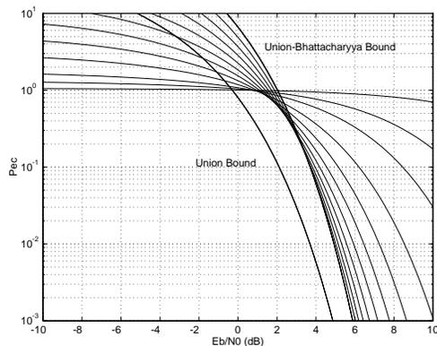
Figure 16: Comparison of Gallager Bound, Union Bound and Union Bhattacharyya Bound for the Nordstrom-Robinson code with BPSK Modulation
