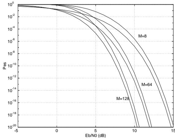
Figure 10: Comparison of Gallager Bound and exact error probability for orthogonal signals. In each group the upper signal is the bound and the lower signal is the exact error probability
