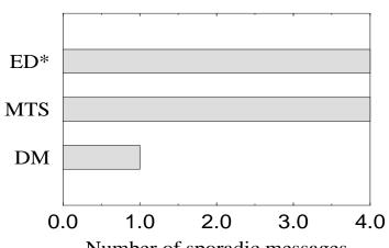
Number of sporadic messages Vary deadlines of high-speed sporadics with number fixed at 2: DM fails at 104.1 $\mu$ s or less; MTS and ED\* can handle even 17.3 $\mu$ s (min. possible).
