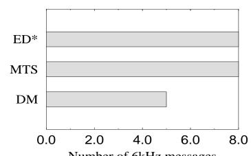
Number of 6kHz messages Vary deadlines of high-speed periodics (with six 6kHz messages and DM fails at 99.9 $\mu$ s or less; MTS and ED\* can handle even 56.8 $\mu$ s (min. possible).
