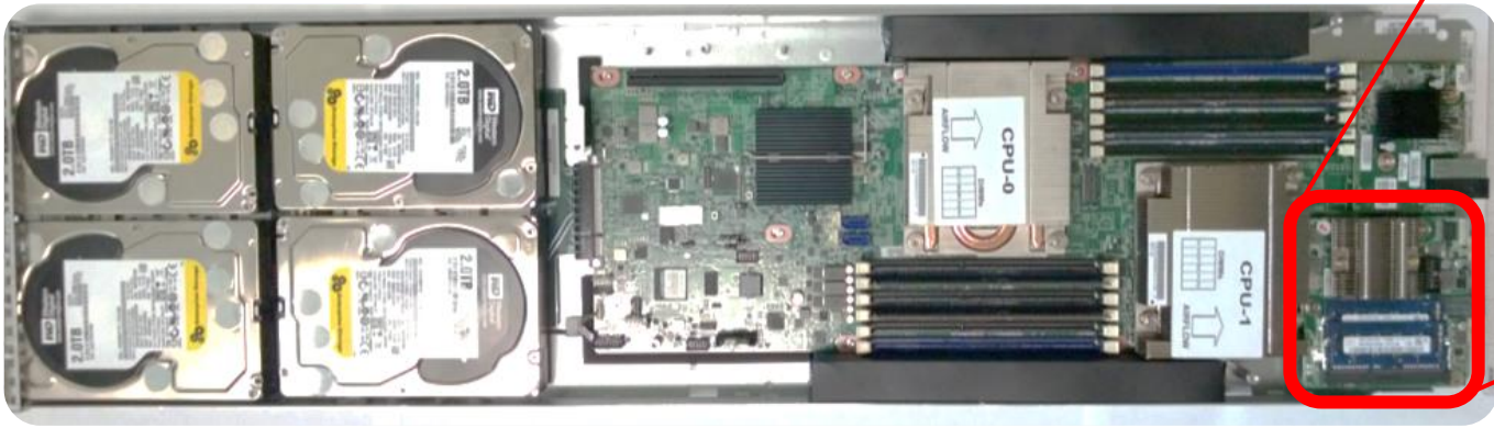
Data Center Server (1U, ½ width)
