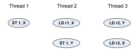
where X and Y are memory locations and "ST 1, X" means "write 1 to memory location X", while "LD r1, X" means "load the contents of memory location X to register r1".
