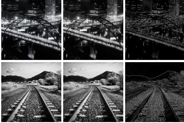
(a) Original (b) Low-Pass (c) High-Pass Fig 2. Example Images after Filter Processing
