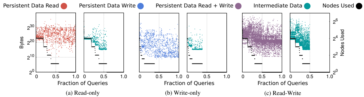
Figure 6: Persistent data read / write and intermediate data exchange characteristics of queries sorted by the number of nodes used. Each plot uses the same axis for bytes (left axis) and nodes used (right axis). Persistent Read and write bytes vary by three orders of magnitude across each node count.
