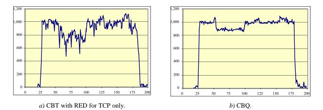
**Figure 6:** Aggregate TCP throughput under "CBT with RED for TCP only" and CBQ (TCP throughput in kilobytes/second versus elapsed time in seconds.)
