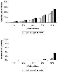
This figure shows the percent of lost replicas and objects when chain lengths are capped using aggressive claims transfer. An object is lost only when all of its replicas are.
