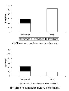
This figure shows the time to transfer both the tree and archive loads for samsarad and the copying utility scp. The Samsara prototype requires three phases to complete the transfer—storing the data at a
