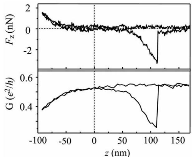
FIG. 3. Deflection force and conductance as a function of tip height for a NT with  $d = 6.5$  nm and  $L_0 = 1.9$   $\mu$ m at  $V_{\text{tip}} = 0$  V. The tip was first moved toward the surface (toward negative  $z$ ) and then away from the surface.
