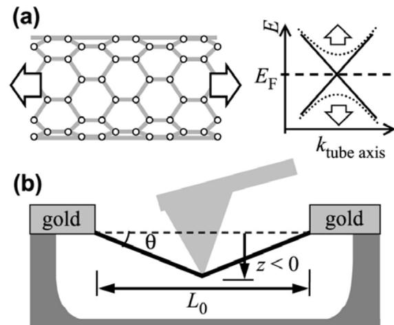
FIG. 1. (a) Real space representation of a zigzag NT and the dispersion relation near  $E_F$ . Solid lines and dashed lines show  $E(k)$  before and after stretching, respectively. (b) Experimental geometry for applying strain and gate voltage with an AFM tip, and measuring conductance with gold contacts.  $L_0$  is distance between anchoring points;  $z$  is the distance the center of the NT is displaced from the plane of the anchoring points.
