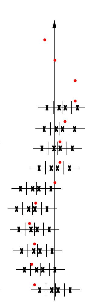
DPCM is a kind of backward adaptive quantizer. The quantizer to use on  $X_i$  is determined by the reconstructions of past  $X$ 's.
