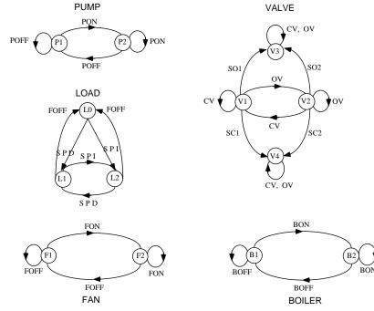
Models of the Components of the HVAC System:
