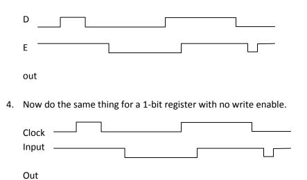
5. Design a one-bit register with a write enable using standard gates (AND, OR, NOT). \$\$
