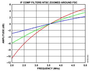
Figure 28. NTSC IF Filter Compensation
