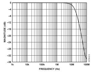
Figure 12. Antialiasing Filter Magnitude Response
