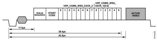
Figure 42. WSS Waveform
