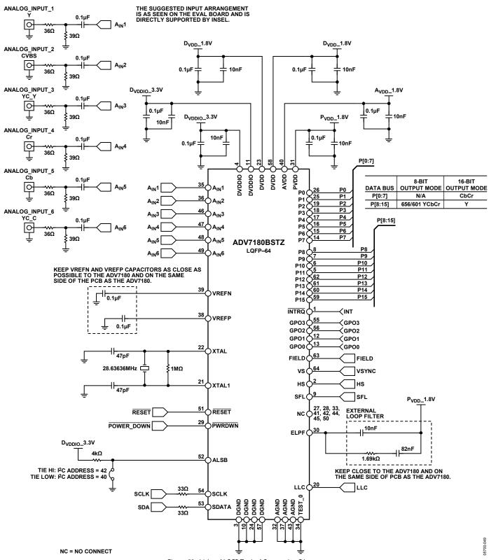
Figure 53. 64-Lead LQFP Typical Connection Diagram
