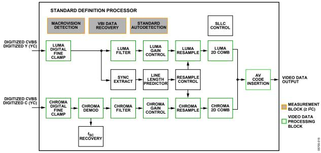
Figure 14. Block Diagram of the Video Processor
