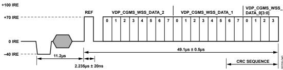
Figure 43. CGMS Waveform
