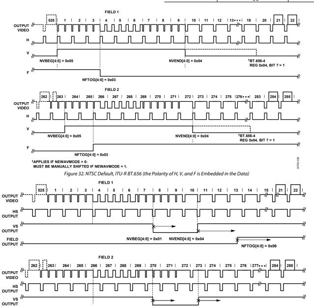
Figure 33. NTSC Typical VSYNC/FIELD Positions Using Register Writes in Table 62 Rev. D | Page 44 of 112
