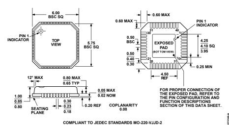
Figure 54. 40-Lead Lead Frame Chip Scale Package [LFCSP\_VQ] 6 mm × 6 mm Body, Very Thin Quad (CP-40-1) Dimensions shown in millimeters
