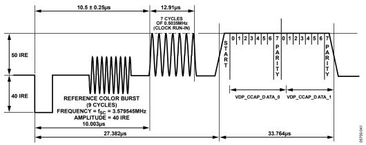
Figure 44. CCAP Waveform and Decoded Data Correlation
