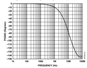
Figure 13. Antialiasing Filter Phase Response
