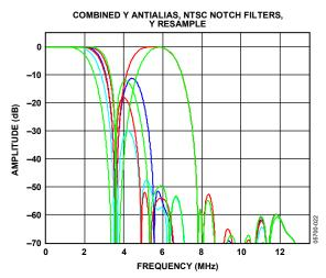
Figure 21. Combined Y Antialias Filter, NTSC Notch Filters
