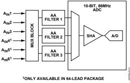
Figure 11. Antialias Filter Configuration
