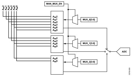
Figure 8. 64-Lead LQFP Internal Pin Connections
