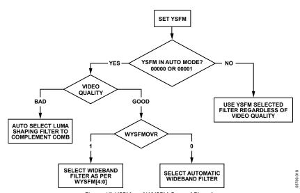
Figure 17. YSFM and WYSFM Control Flowchart
