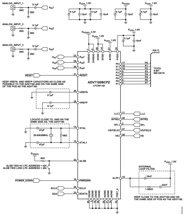
Figure 52. 40-Lead LFCSP Typical Connection Diagram
