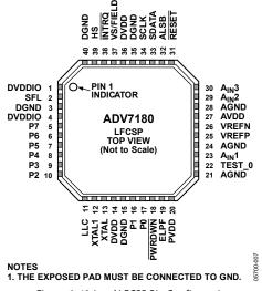
Figure 6. 40-Lead LFCSP Pin Configuration
