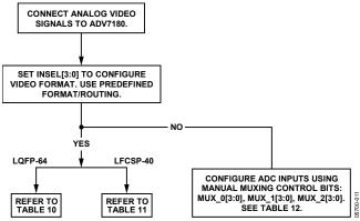
Figure 10. Signal Routing Options
