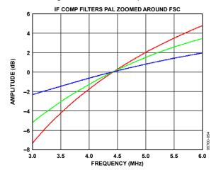
Figure 29. PAL IF Filter Compensation
