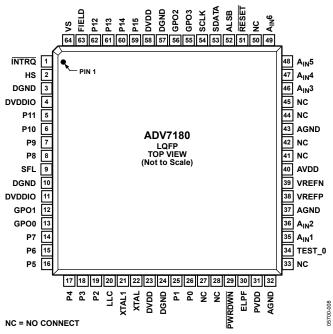
Figure 7. 64-Lead LQFP Pin Configuration
