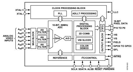
Figure 2. 64-Lead LQFP Functional Block Diagram
