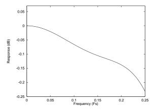
Figure 41 DAC Digital Filter Frequency Response -Type 3
