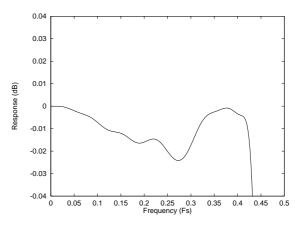
Figure 37 DAC Digital Filter Frequency Response -Type 1
