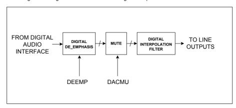
Figure 17 DAC Filter Schematic
