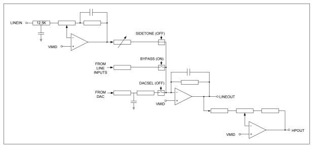
Figure 23 Signal Routing in Bypass Mode
