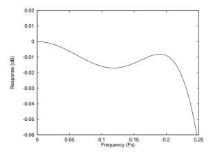
Figure 49 ADC Digital Filter Frequency Response -Type 3
