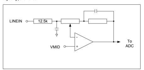
Figure 10 Line Input Schematic
