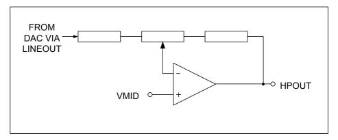
Figure 21 Headphone Amplifier Schematic
