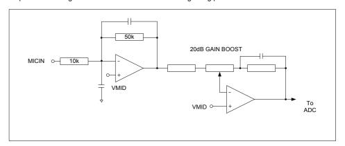
Figure 12 Microphone Input Schematic
