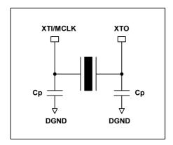
Figure 25 Crystal Oscillator Application Circuit
