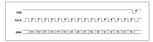
Figure 33 3-Wire Serial Interface
