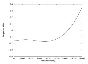
Figure 51 De-Emphasis Frequency Response (32kHz)
