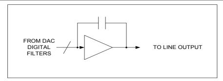
Figure 18 Multi-Bit Oversampling Sigma Delta Schematic
