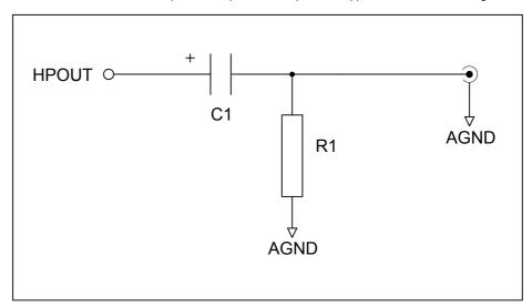
Figure 22 Headphone Output Application Drawing
