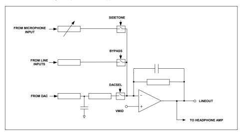
Figure 19 Line Output Schematic
