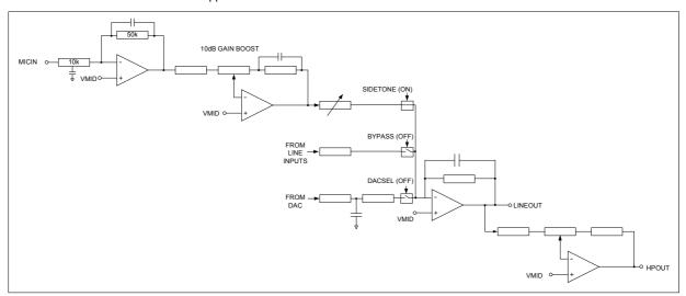
Figure 24 Side Tone Mode Schematic
