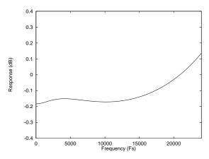
Figure 55 De-Emphasis Frequency Response (48kHz)
