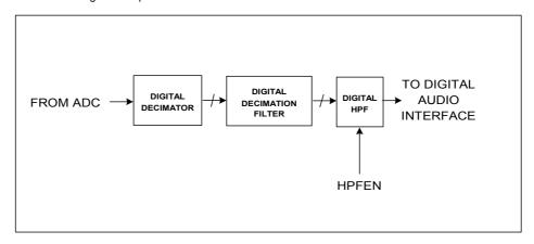
Figure 16 ADC Digital Filter
