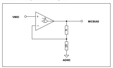
Figure 14 Microphone Bias Schematic
