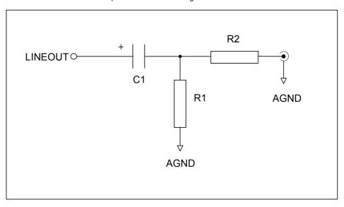
Figure 20 Line Outputs Application Drawing
