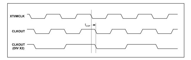
Figure 2 Clock Out Timing Requirements
