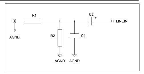
Figure 11 Line Input Application Drawing
