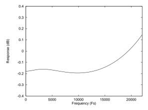
Figure 53 De-Emphasis Frequency Response (44.1kHz)
