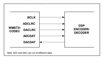
Figure 3 Master Mode Connection
