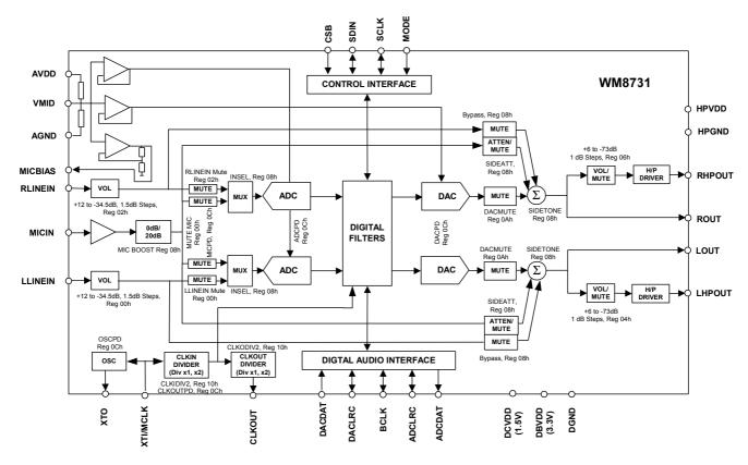
Figure 9 Functional Block Diagram
