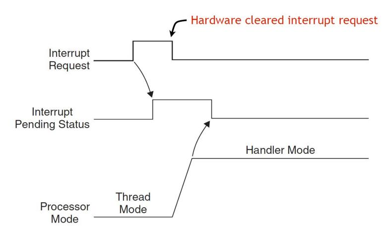
The normal case. Once Interrupt request is seen, processor puts it in "pending" state even if hardware drops the request. IPS is cleared by the hardware once we jump to the ISR.
