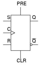
Traditionally, CLR is used to indicate async reset. "R" or "reset" for sync. reset.
