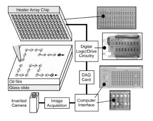
Schematic of the programmable system for noncontact droplet actuation based on Marangoni flows. The system includes a 128-pixel array of resistive heaters suspended above the oil layer, control circuitry, and a graphical user interface.
