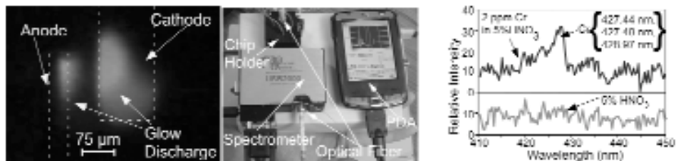
Left – The microglow discharge at 1atm pressure, Middle – The handheld system for chemical analysis, Right – Spectrum showing 427.5nm Cr line in 2ppm Cr solution.
