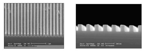
120nm linewidth dense grating imprinted in epoxy-based SSQ resin, and pattern transferred into oxide by using the imprinted SSQ template as a dry etching mask.
