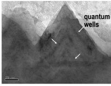
Photoluminescence shows a much improved light output intensity compared to conventional devices with planar quantum wells. Cross-sectional transmission electron micrograph confirms the formation of quantum wells on semipolar planes.
