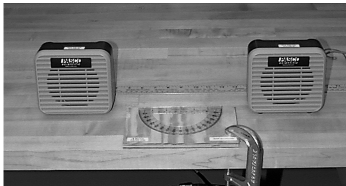
Figure 1-4: Configuration for finding the standing wave pattern in front of the two speakers.
