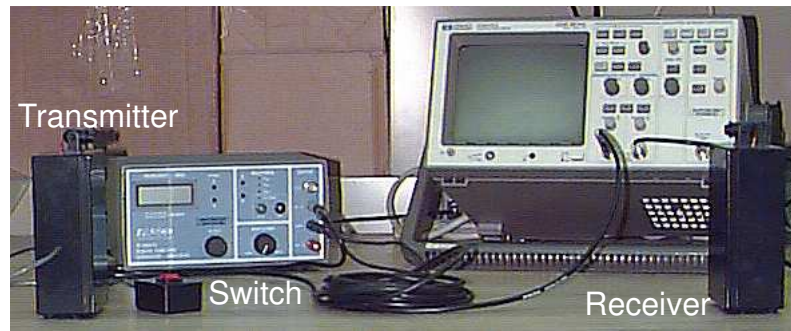
Figure 1-7: Setup for the speed of sound experiment.
