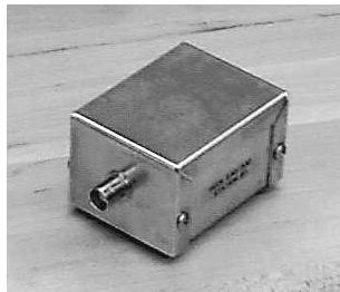
Figure 5-3: The lossy line simulator.
