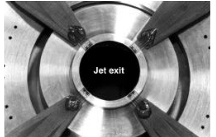
Figure 7: Actuator chips mounted on a PC board, which is attached to the front surface of the nozzle. This device has been tested on a high-speed jet facility.
