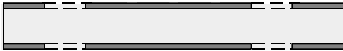
(a) Shallow boron diffusion to define beams, proofmass, and supporting rim. Nitride deposition and definition for electrode anchors and isolation dielectric underneath electrode dimples.
