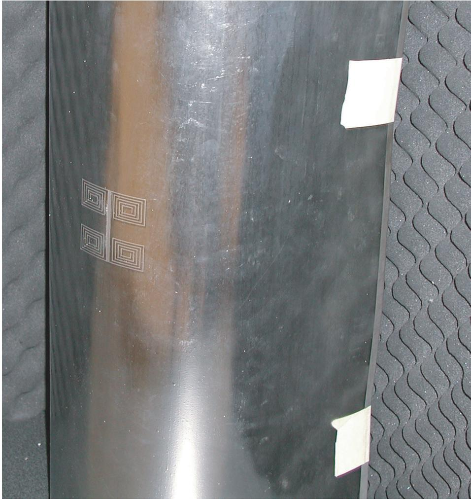
Figure 3.16: A photograph of the miniaturized slot antenna conformed into a curved surface along the E-plane.
