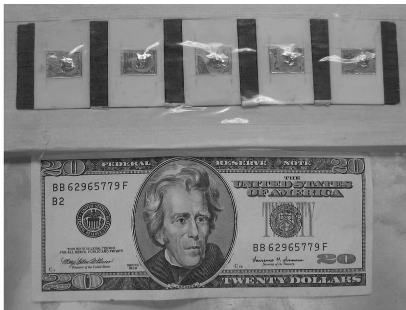
Figure 8.8:  $1.18\lambda_0$  five-element metamaterial enabled patch array for 2GHz operation
