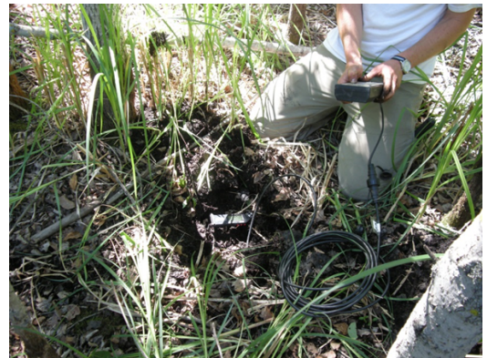
Figure A.5: Soil moisture sampling location (left) with inserted soil moisture probe (right).
