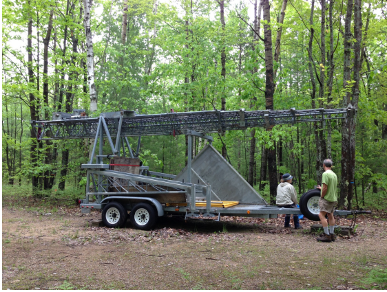
Figure 2.28: Field work in May 2013 at UMBS. Figure on left: folded tower radar with view on radar footprint (behind radar). Figure on right: measurement in the radar footprint.
