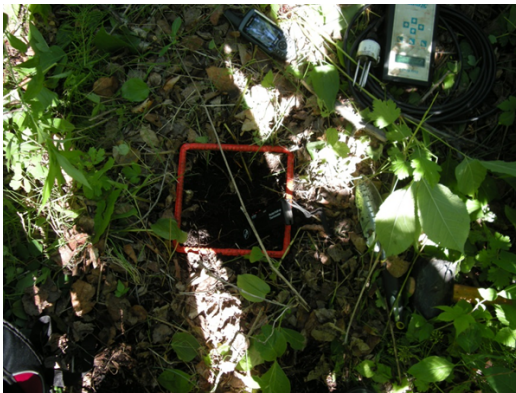
Figure A.5: Soil moisture sampling location (left) with inserted soil moisture probe (right).
