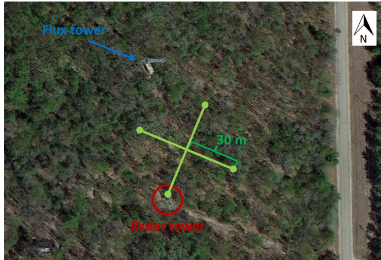
Figure 2.26: Google Earth image of the UMBS site with radar tower, two transects of May 2013 field work and flux tower location.
