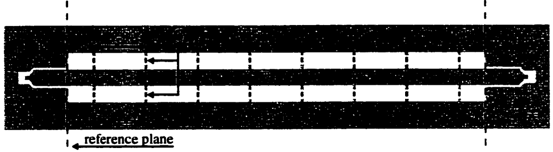
Figure 3.3: Typical test structure used in conjunction with the distributed technique.
