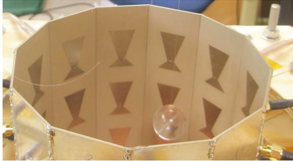
Figure 7.22: Second cavity with antennas designed to operate at 915 MHz of Experiment 2. Three acrylic sphere are suspended (one visible). Cavity is filled with fluid for imaging.
