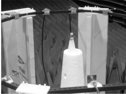
Figure 6.7: Setup to test the antenna model by measuring the scattered field from a conducting sphere. The sphere has a diameter of 2 inches, and was centered in the setup.
