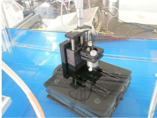
Figure 8.11: Photo of micropositioner with transducer to measure the speed of sound of the water bath.
