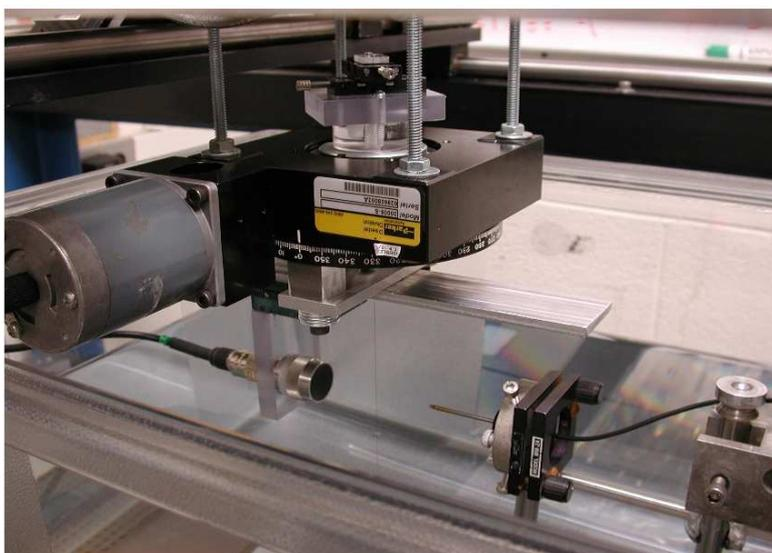
Figure 8.1: Photo of an early hydrophone characterization experiment. A transducer is gimbaled and mounted on a translator. The focus of the transducer is positioned at the center of rotation of the rotational stage. A hydrophone is also gimbaled and positioned with a 3-axis micropositioner.
