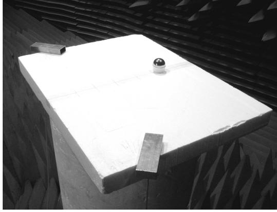
Figure 4.9: Example of anechoic chamber measurements of  $S_{21}$  for a scatterer. The scatterer is a 2 inch diameter conducting sphere. Waveguide apertures in photo are separated by 0.85 m and rotated 40 degrees. The sphere is positioned near the boresights of the waveguide apertures.
