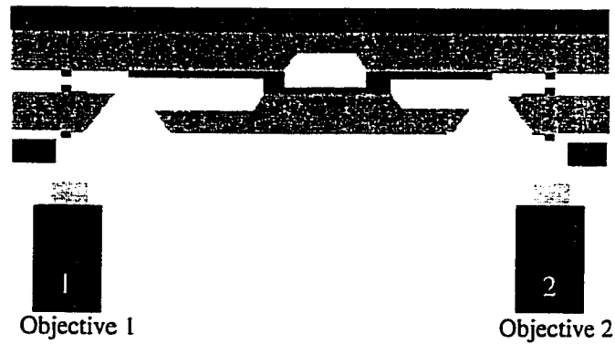
(d) Upper bonding chuck is lowered to form contact between upper and lower wafers. Alignment is complete.
