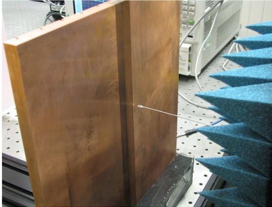
(b) Small loop measuring the pattern created by OC
