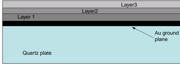
Figure 3.13: Cross section of samples with optical polymers.
