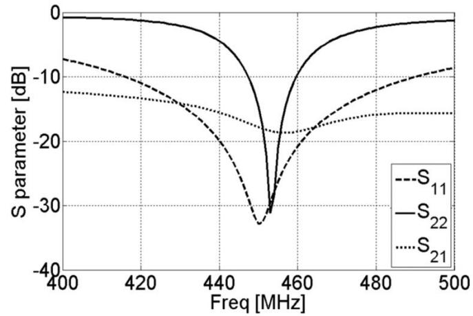
Figure 5.18: Simulated  $S_{11}$ ,  $S_{21}$  and  $S_{22}$  of the proposed pattern diversity antenna.
