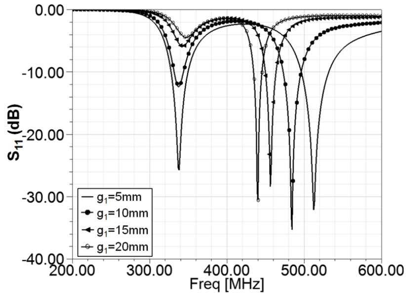
Figure 5.7: Simulated  $S_{11}$  of the proposed bow-tie microstrip antenna versus  $g_1$ .
