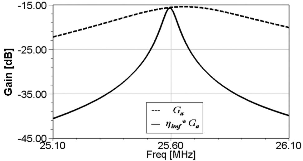
Figure 6.1: Antenna gain with and without considering impedance mismatch factor to a feed ( $\eta_{inf}$ ).
