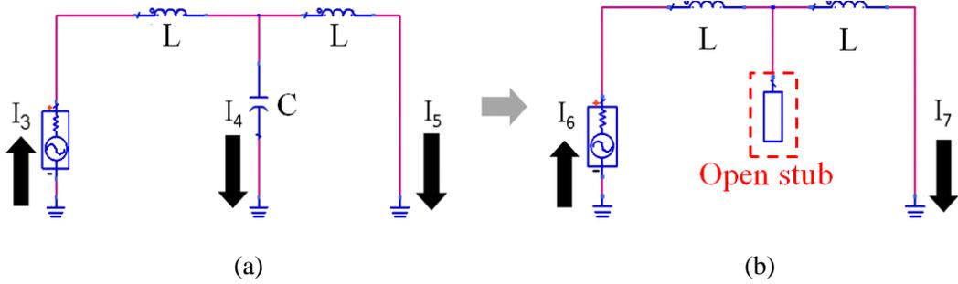
Figure 2.17: (a) Circuit model for a T-type 180 degree phase shifter and (b) circuit model employing an open stub instead of a grounded capacitor in (a).
