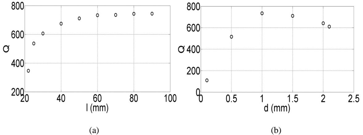
Figure 2.30: Calculated  $Q$  versus (a)  $l$  (=coil length) where  $d = 1$  mm, and (b)  $d$  (=wire diameter) where  $l = 70$ mm.
