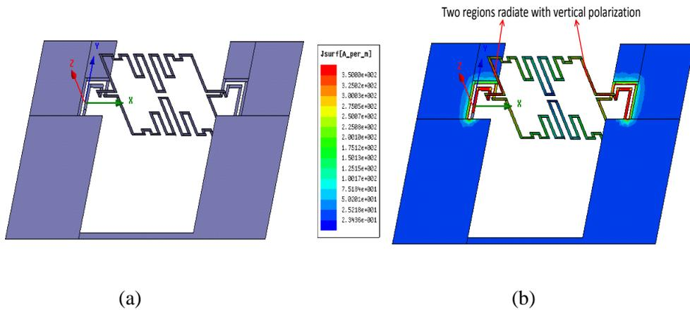
Figure 3.11: (a) The proposed antenna and (b) its surface current distribution.
