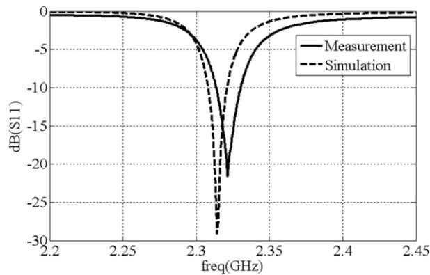
Figure 2.13: Measured and simulated  $S_{11}$  of a miniaturized single-layer ICCLMA on a large ground plane.
