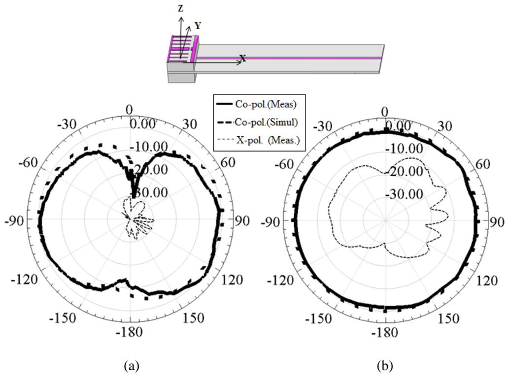
Figure 3.6: Measured and simulated (a) E-Plane (=XZ-Plane) and (b) H-Plane (=XY-Plane) radiation patterns of the proposed balanced architecture.
