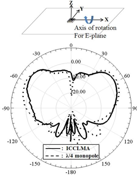
Figure 2.14: Measured E-Plane radiation patterns of a ICCLMA and  $\lambda_0/4$  monopole antenna.
