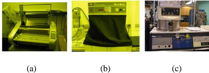
Figure 3.15: (a) Photoresist laminator, (b) exposure machine, and (c) sputtering system.
