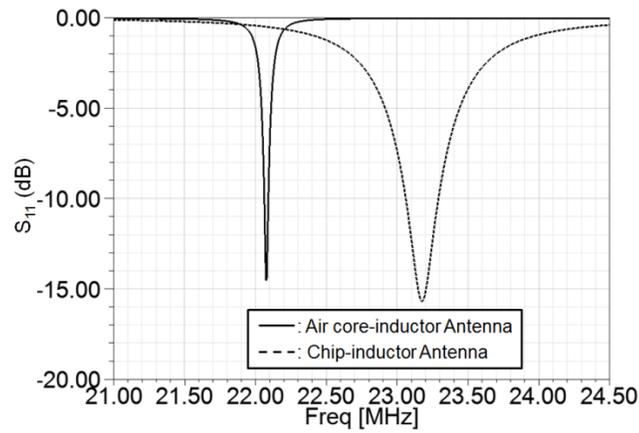
Figure 2.33: Simulated  $S_{11}$  of the proposed antenna with air-core inductors, compared to that of the antenna with chip inductors. Narrower bandwidth indicates higher radiation efficiency because the antenna volume is fixed.
