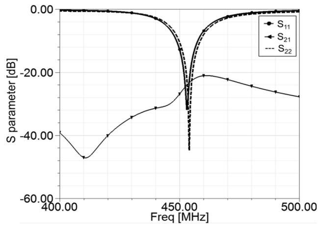
Figure 5.10: Simulated  $S_{11}$ ,  $S_{21}$  and  $S_{22}$  of the proposed polarization diversity antenna.
