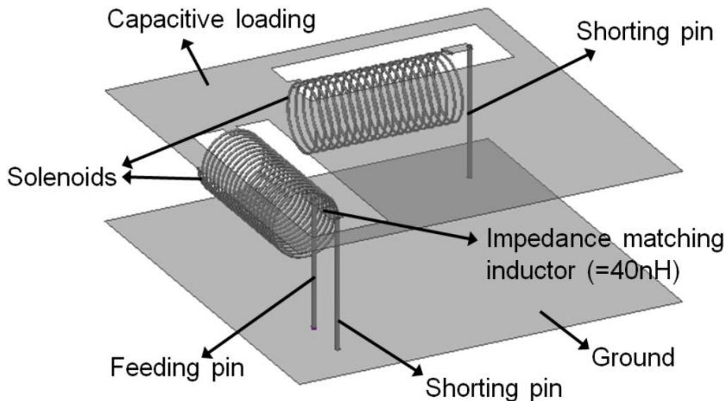
Figure 2.31: Geometry of the proposed antenna with air-core inductors having the dimensions of 150mm X 150mm X 50mm.
