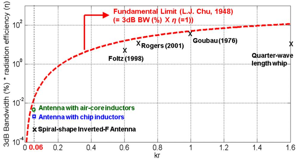
Figure 2.36: Performance comparison among the electrically small antennas shown in this work.
