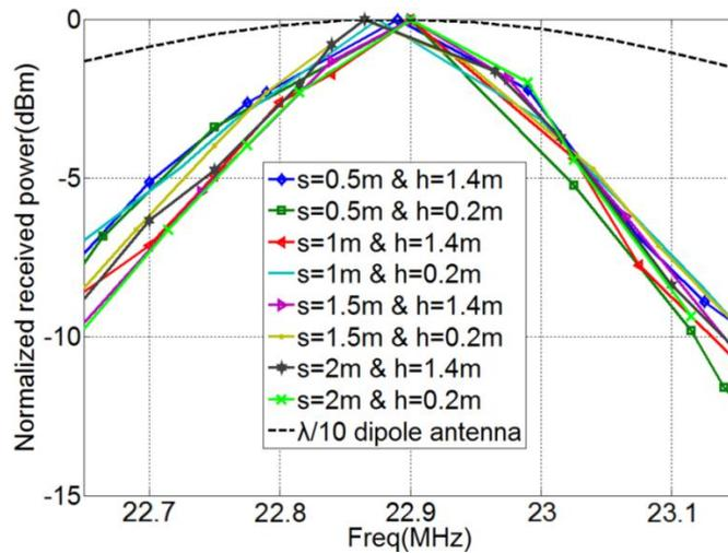
Figure 2.38: Measured received normalized power corresponding to various positions of the transmitting (=proposed) antenna shown in Fig. 2.37.
