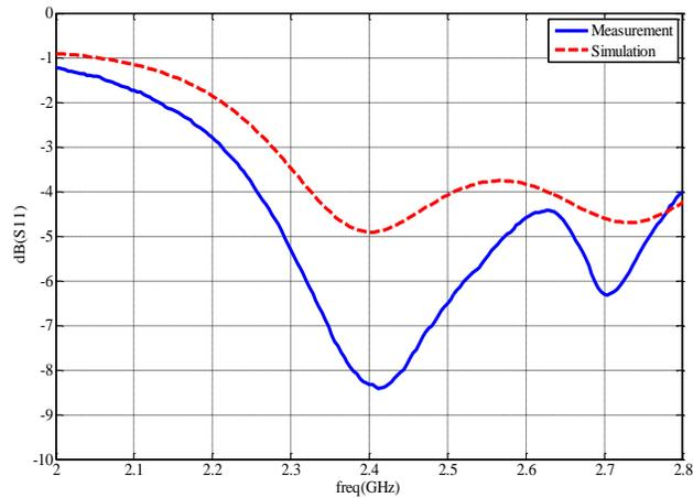
Figure 3.19: Measured and simulated return loss ( $S_{11}$ ).
