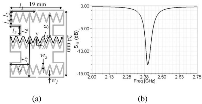
Figure 4.10: (a) Topology, design parameters and (b) simulated  $S_{11}$  of the proposed CP antenna exhibiting 72% size reduction as compared to the conventional corner-truncated square microstrip antenna.
