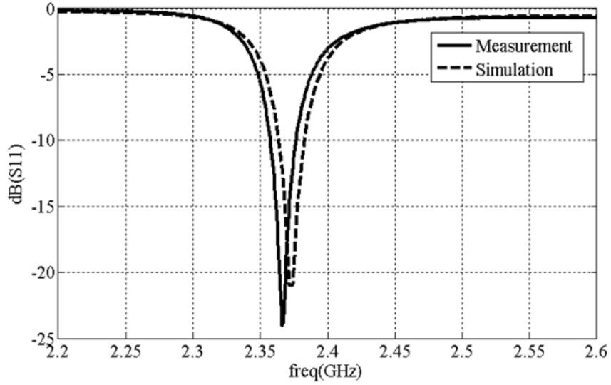
Figure 3.5: Measured and simulated  $S_{11}$  of the proposed balanced architecture.
