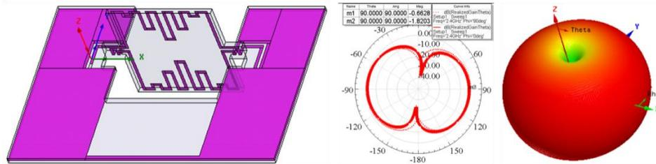
Figure 3.13: Embedded antenna inside paper and its 2D/3D radiation patterns.
