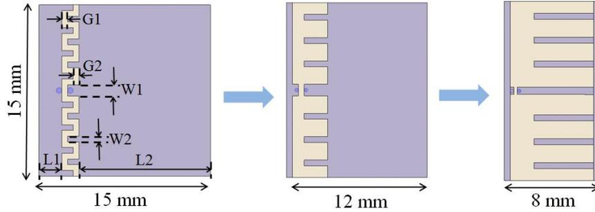
Figure 2.11: Design procedure for additional size reduction of single-layer ICCLMA.
