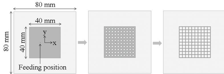
Figure 4.1: Conversion of a  $\lambda_g/2$  microstrip antenna to an array of thin wires.
