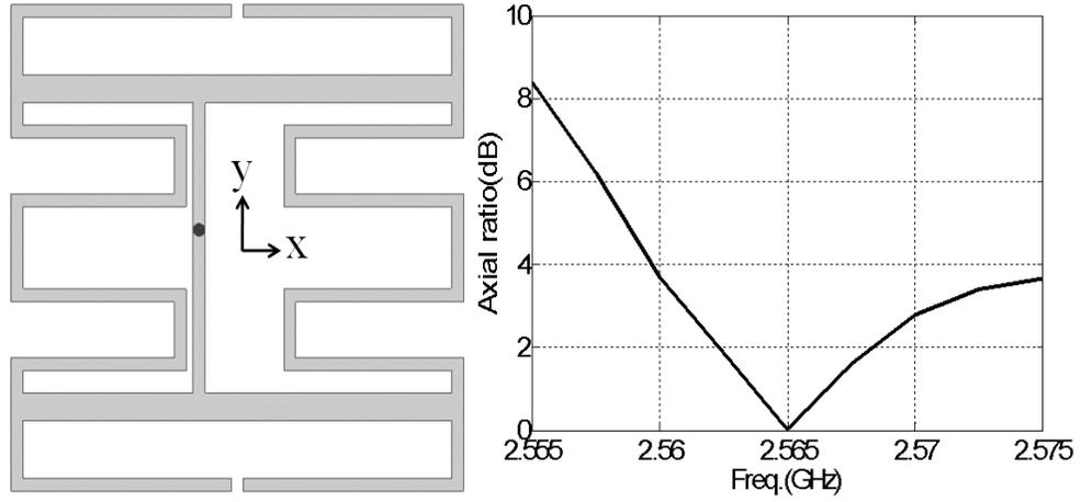
Figure 4.17. Measured axial ratio in the broadside direction for the antenna shown in Fig. 4.16(a).
