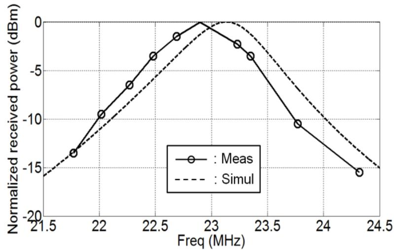
Figure 2.22: Measured and simulated power received at the reference  $\lambda_0/10$  dipole antenna and normalized by the peak value of each response versus frequency when the proposed antenna with chip inductors is used as a transmitting antenna.
