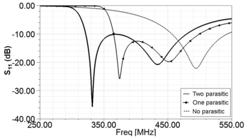
Figure 3.35: Simulated  $S_{11}$  of the proposed antenna corresponding to three cases: *i*. Antenna without any parasitic element ('no parasitic'), *ii*. Antenna with one parasitic element ('one parasitic') and *iii*. Antenna with two parasitic elements (denoted by 'two parasitic').
