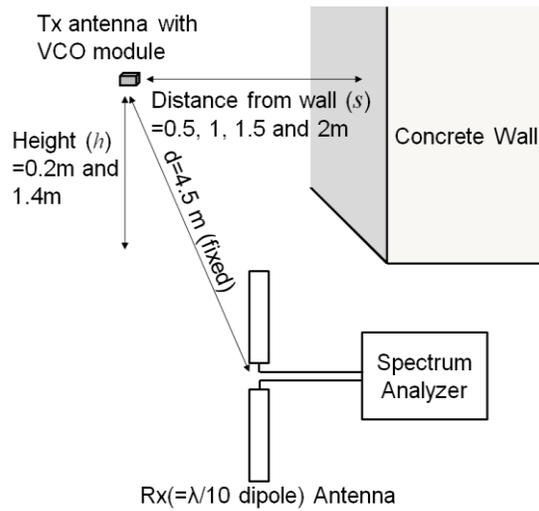
Figure 2.37: Measurement set up for examining the proximity effect of nearby objects on the resonant frequency of the proposed narrow band antenna.
