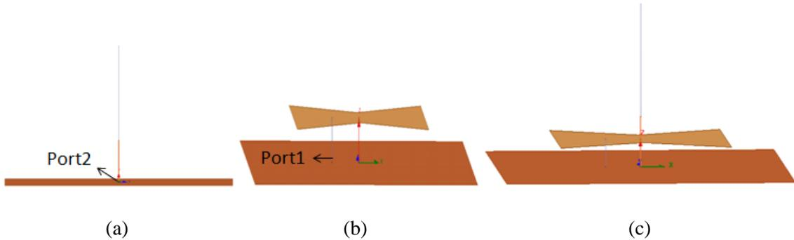
Figure A.3: (a) Quarter-wave monopole antenna, (b) bow-tie patch antenna, and (c) proposed radiation pattern diversity antenna.
