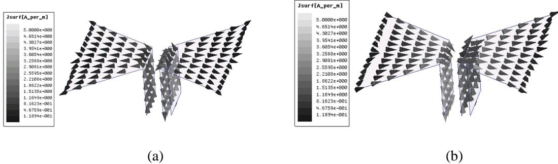
Figure 5.5: Current distributions of the proposed antenna in Fig. 5.3 at (a) 342MHz and (b) 456MHz.
