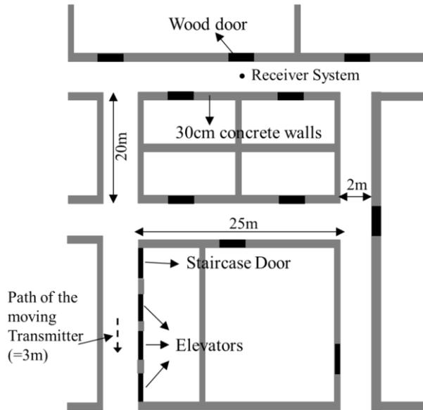
Figure A.12: Measurement set up on 3rd floor in EECS building in the University of Michigan.
