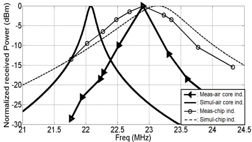
Figure 2.34: Measured and simulated power received at the reference  $\lambda_0/10$  antenna and normalized by the peak value of each response versus frequency when the proposed antenna with air-core inductors is used as a transmitting antenna, compared to those of the antenna with chip inductors.
