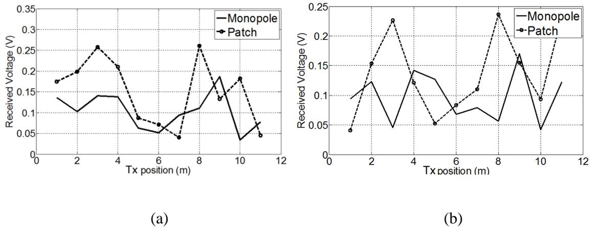
Figure A.13: Two output signals from the two receiving antennas (a) when monopole antenna is ‘ON’ and patch antenna is ‘OFF’ and (b) when monopole antenna is ‘OFF’ and patch antenna is ‘ON’.
