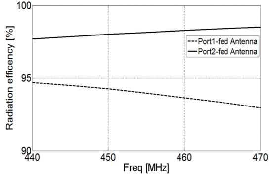
Figure 5.13: Simulated radiation efficiency of two antenna elements in the proposed polarization diversity antenna.
