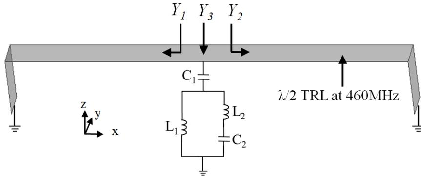
Figure 3.27: Input admittances toward two shorting sheets and parasitic element in the middle of a shorted  $\lambda/2$  TRL.
