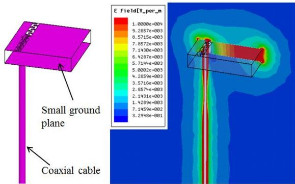
Figure 3.1: Electric field distribution in the proposed antenna fed by coaxial cable.
