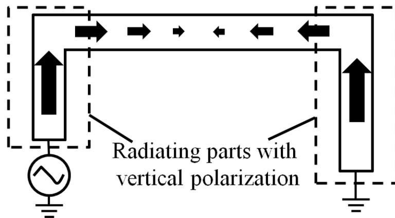
Figure 3.23: Directions and amplitudes of electric currents on  $\lambda/2$  folded monopole antenna.
