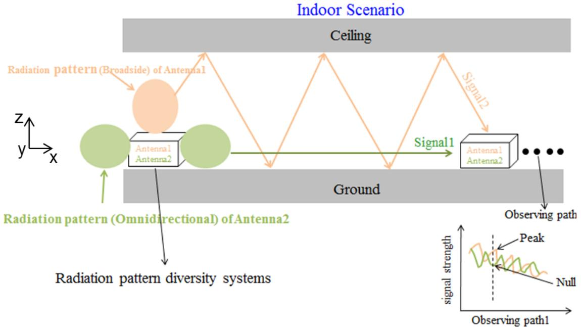
Figure A.2: Indoor scenario utilizing radiation pattern diversity antenna system.
