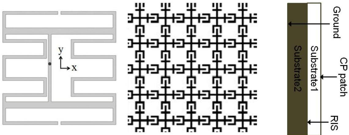
Figure 6.3: Proposed miniaturized CP patch antenna further reduced by being mounted on the RIS.
