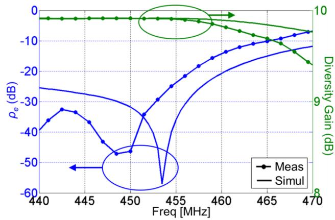
Figure 5.14: Envelop correlation ( $\rho_e$ ) between radiation patterns of two antenna elements in the proposed polarization diversity antenna and diversity gain.
