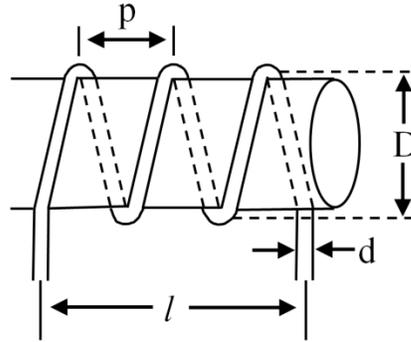
Figure 2.29: Design parameters of the air-core coil.
