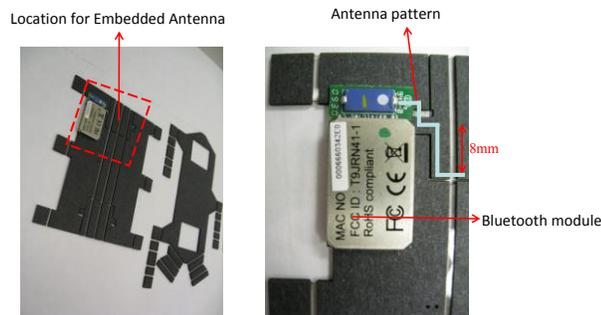
Figure 3.8: Integration of an embedded antenna with Bluetooth module.
