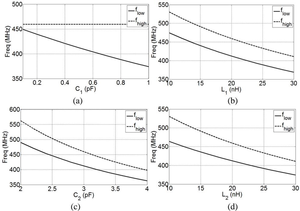
Figure 3.28:  $f_{low}$  and  $f_{high}$  versus (a)  $C_1$ , (b)  $L_1$ , (c)  $C_2$  and (d)  $L_2$  in the equivalent circuit model of the parasitic element in Fig. 3.27. Each plot shows the fixed values of other parameters.
