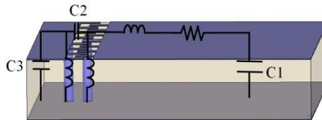
Figure 2.10: Equivalent circuit model of single-layer ICCLMA.
