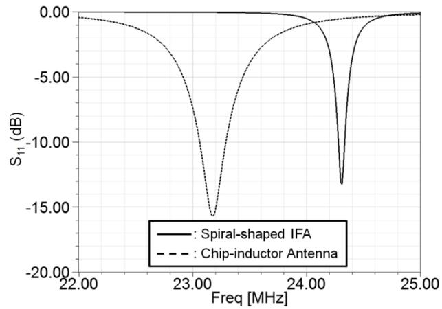
Figure 2.25: Simulated  $S_{11}$  of spiral-shaped inverted-F antenna on the substrate with  $\epsilon_r = 10.2$ , compared to that of the proposed antenna with chip inductors.
