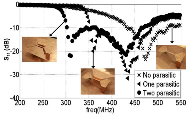
Figure 3.37: Measured  $S_{11}$  of the proposed antenna corresponding to the three cases: *i.* No parasitics, *ii.* One parasitic and *iii.* Two parasitics.
