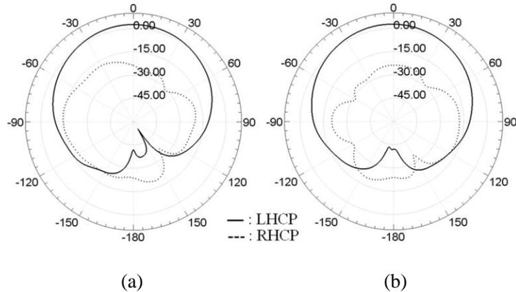
Figure 4.12: Simulated radiation patterns in two orthogonal planes of (a)  $xz$  and (b)  $yz$ -planes for the antenna shown in Fig. 4.10(a).
