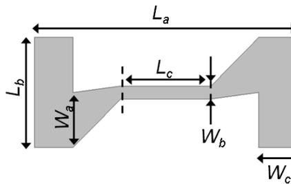
Figure 3.30: Design parameters of the meandered  $\lambda/2$  folded monopole antenna.
