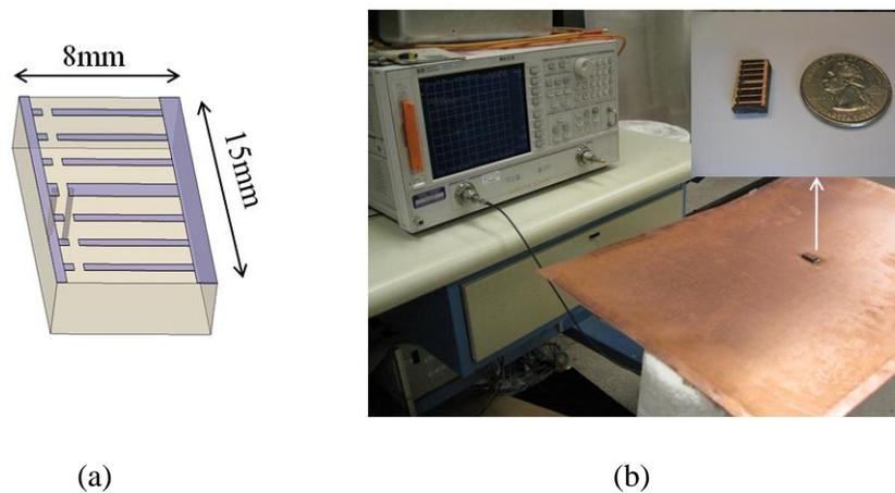
Figure 2.12: (a) Miniaturized single-layer ICCLMA and (b) measurement set up using a large ground plane ( $3\lambda_0 \times 3\lambda_0$ ).
