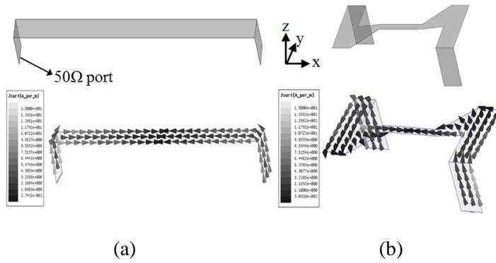
Figure 3.29: Geometries and electric current distributions of (a) the straight and (b) meandered  $\lambda/2$  folded monopole antenna.
