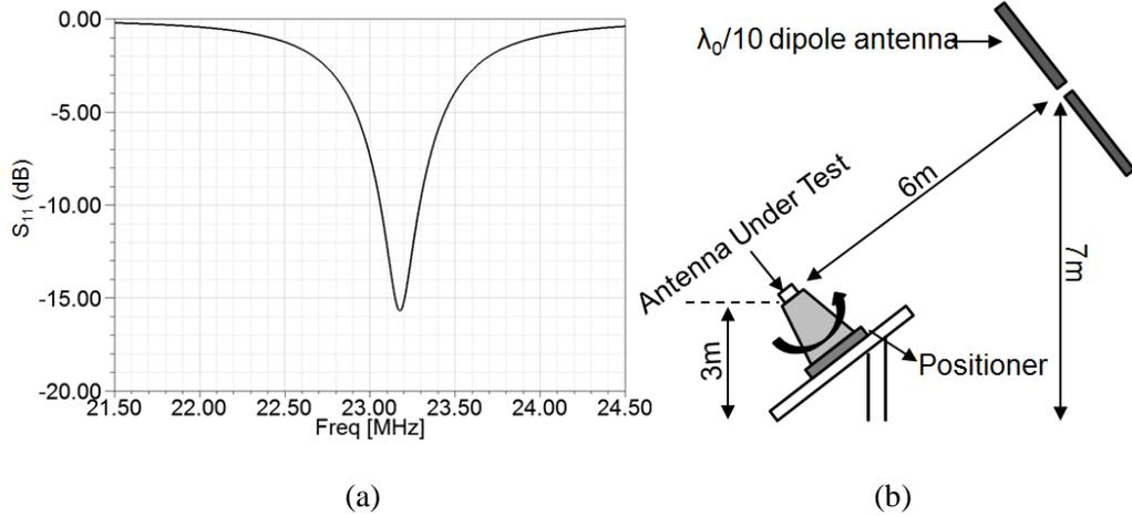
Figure 2.20: (a) Simulated  $S_{11}$  of the proposed antenna with chip inductors and (b) measurement setup in an elevated antenna range.
