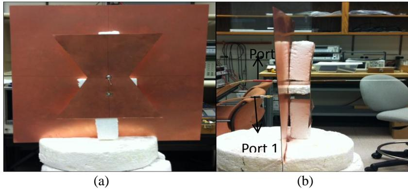
Figure A.7: (a) Top view and (b) side view of the fabricated pattern diversity antenna.
