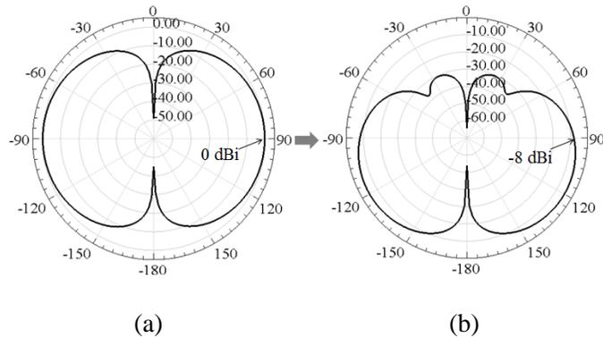
Figure 3.2: Simulated E-Plane radiation pattern of single-layer ICCLMA (a) without and (b) with a coaxial cable.
