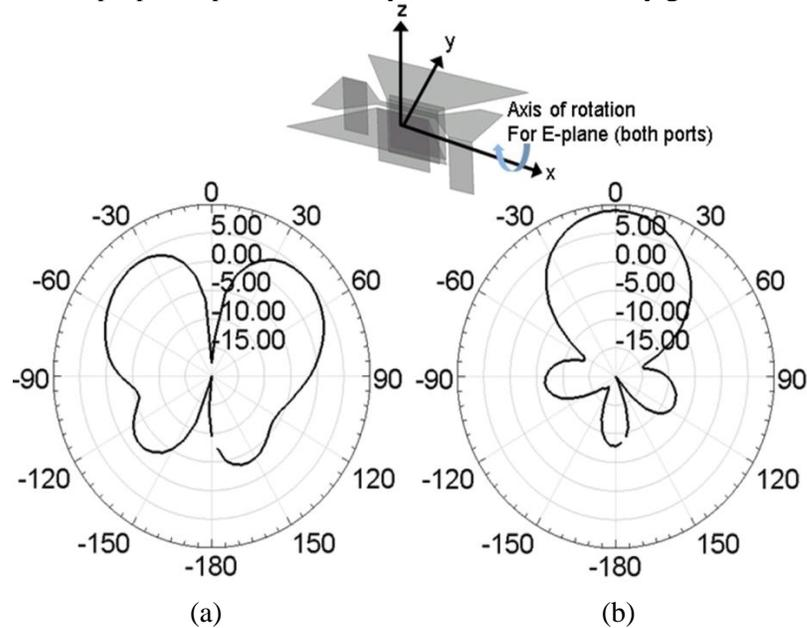
Figure 5.22: Measured radiation patterns on E-planes of the folded monopole antenna and proposed bow-tie microstrip antenna: (a) Port1: ON and Port2: OFF (50 $\Omega$  terminated) and (b) Port1: OFF (50 $\Omega$  terminated) and Port2: ON.
