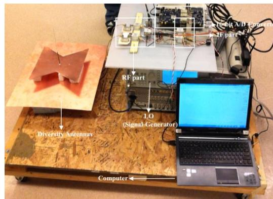
Figure A.11: Receiving system including diversity antennas and a computer.
