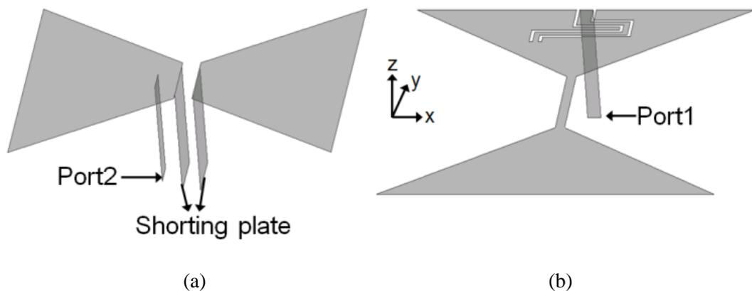
Figure 5.8: (a) Proposed bow-tie microstrip antenna with x-pol and (b) conventional bow-tie microstrip antenna with y-pol.
