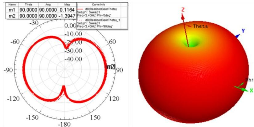
Figure 3.12: 2D and 3D radiation patterns of the proposed antenna.
