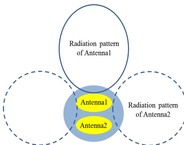
Figure A.1: Radiation pattern diversities using two antennas.
