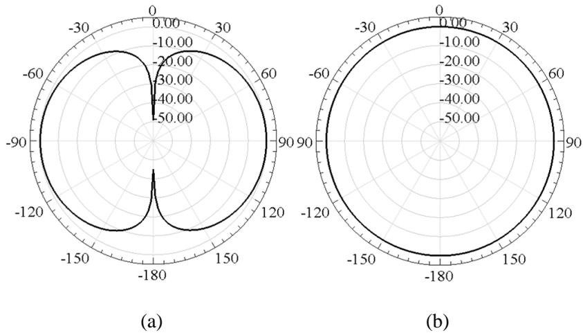
Figure 2.9: Simulated (a) E-Plane and (b) H-Plane radiation patterns of a single layer ICCLMA when  $L = \lambda_0/8$  and  $h = \lambda_0/40$ .
