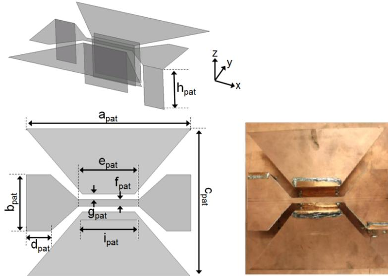
Figure 5.17: Geometry and design parameters of the proposed pattern diversity antenna.
