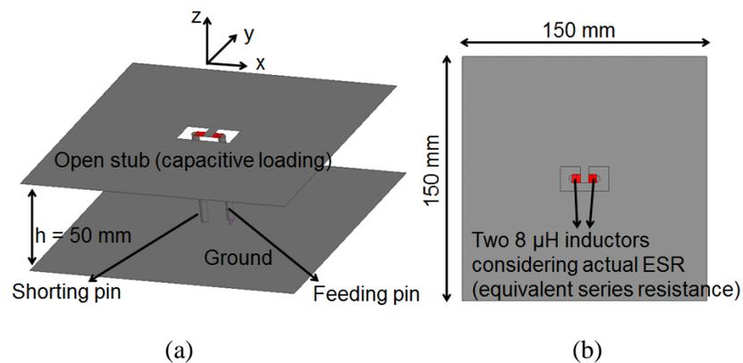
Figure 2.19: (a) Side view and (b) top view of the proposed antenna with chip inductors.
