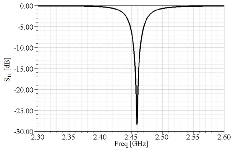
Figure 2.5: Simulated  $S_{11}$  when  $L = \lambda_0/8$  and  $h = \lambda_0/40$ .
