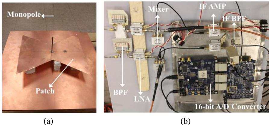
Figure A.10: (a) Fabricated diversity antennas and (b) receiving module.
