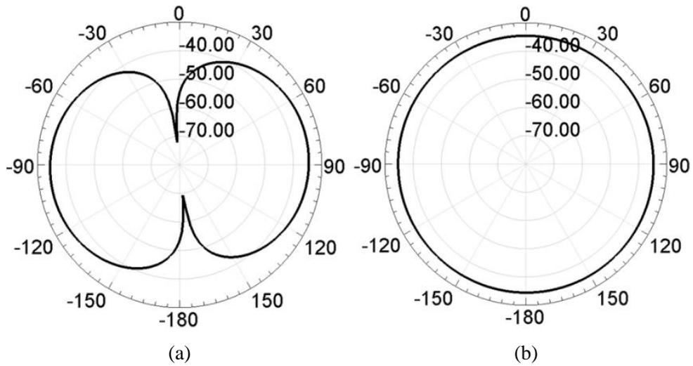
Figure 2.26: Simulated radiation patterns of spiral-shaped inverted-F antenna on the substrate with  $\epsilon_r = 10.2$  in the (a) E (=yz) plane and (b) H (=xy) plane.
