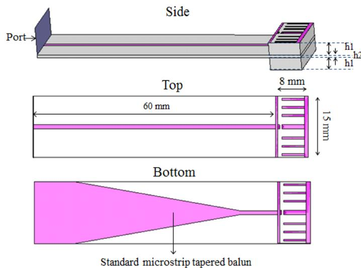
Figure 3.4: Side, top and bottom views of measurement set up of a balanced miniaturized antenna compatible with unbalanced measurement system.
