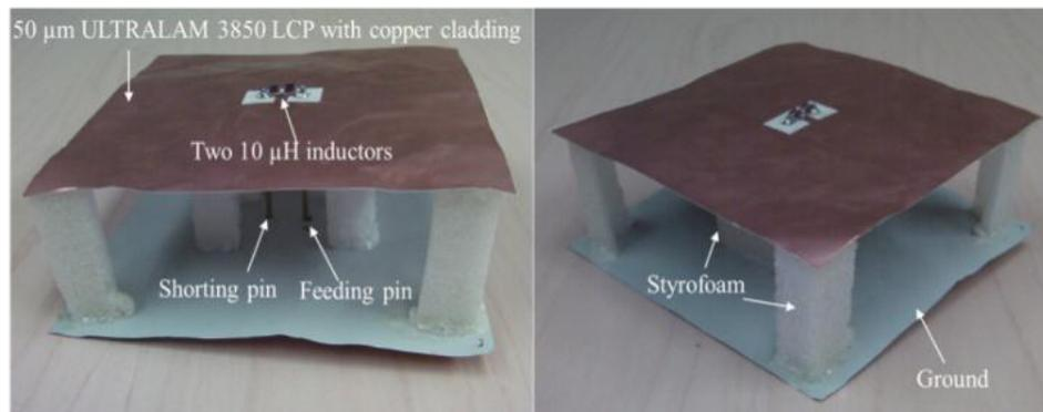
Figure 2.27: Proposed antenna fabricated using flexible thin substrates.
