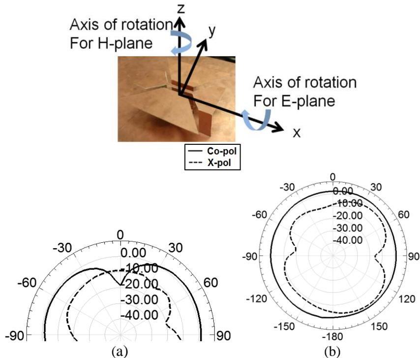
Figure 3.38: Measured radiation patterns of the proposed antenna at 310MHz: (a) E-Plane and (b) H-Plane.
