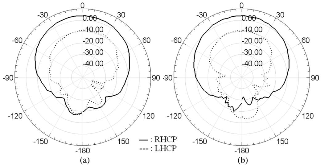
Figure 4.18: Measured radiation patterns in two orthogonal planes of (a) xz and (b) yz-planes for the antenna shown in Fig. 4.16(a).
