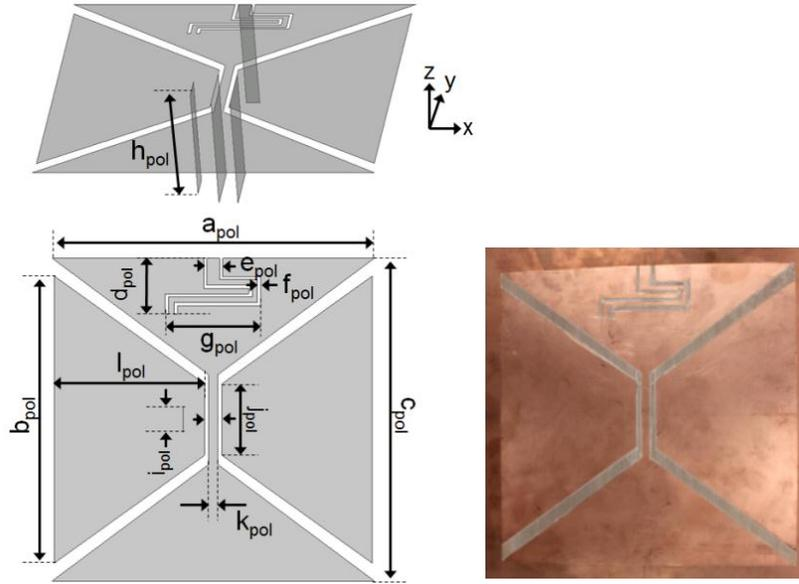
Figure 5.9: Geometry and design parameters of the proposed polarization diversity antenna.
