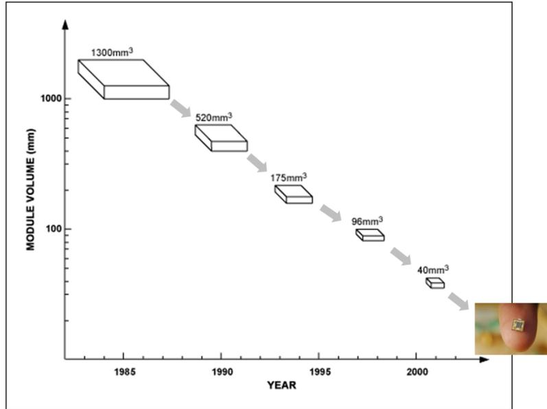
Figure 1.2: VCO module size scaling versus time [3].
