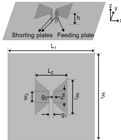
Figure 5.3: Geometry and design parameters of the bow-tie version of the proposed microstrip antenna with an open area in its middle.
