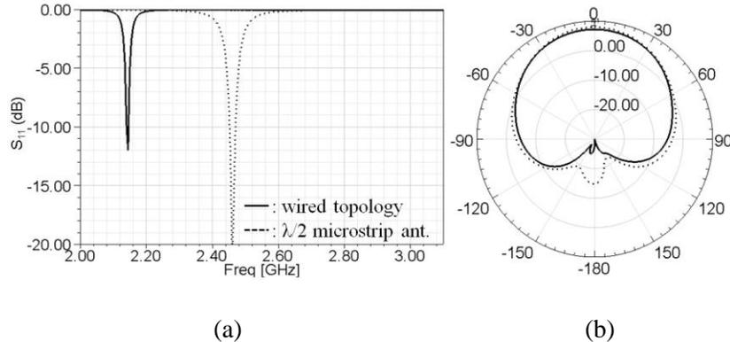
Figure 4.2: Simulated (a)  $S_{11}$  and (b) radiation pattern on xz-plane of a wire mesh patch antenna and a conventional  $\lambda_g/2$  microstrip antenna with the same sizes and substrate.
