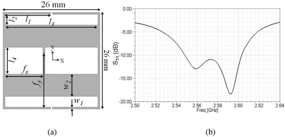
Figure 4.13: (a) Topology, design parameters and (b) measured  $S_{11}$  of the proposed CP antenna exhibiting 53% size reduction as compared to the conventional corner-truncated square microstrip antenna.
