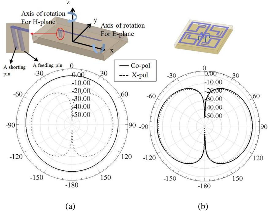
Figure 2.7: E-Plane radiation patterns of (a) a conventional inverted-F antenna and (b) multi-element monopole antenna with the same vertical profile as the height of the proposed antenna ( $=\lambda_0/40$ ).
