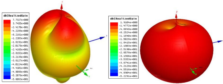
Figure A.6: 3D radiation patterns ( $E_{\theta}$ ) of the proposed radiation pattern diversity antenna: (a) when the bowtie patch antenna is ‘ON’ and the  $\lambda/4$  monopole antenna is ‘OFF’ (broadside radiation pattern), and (b) when the bowtie patch antenna is ‘OFF’ and the  $\lambda/4$  monopole antenna is ‘ON’ (omnidirectional radiation pattern).
