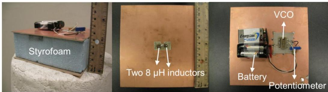
Figure 2.21: Fabricated antenna with chip inductors, integrated with the source module.
