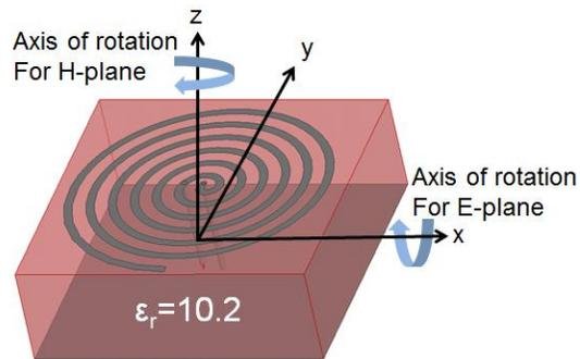
Figure 2.24: Spiral-shaped inverted-F antenna on the substrate with  $\epsilon_r = 10.2$ .
