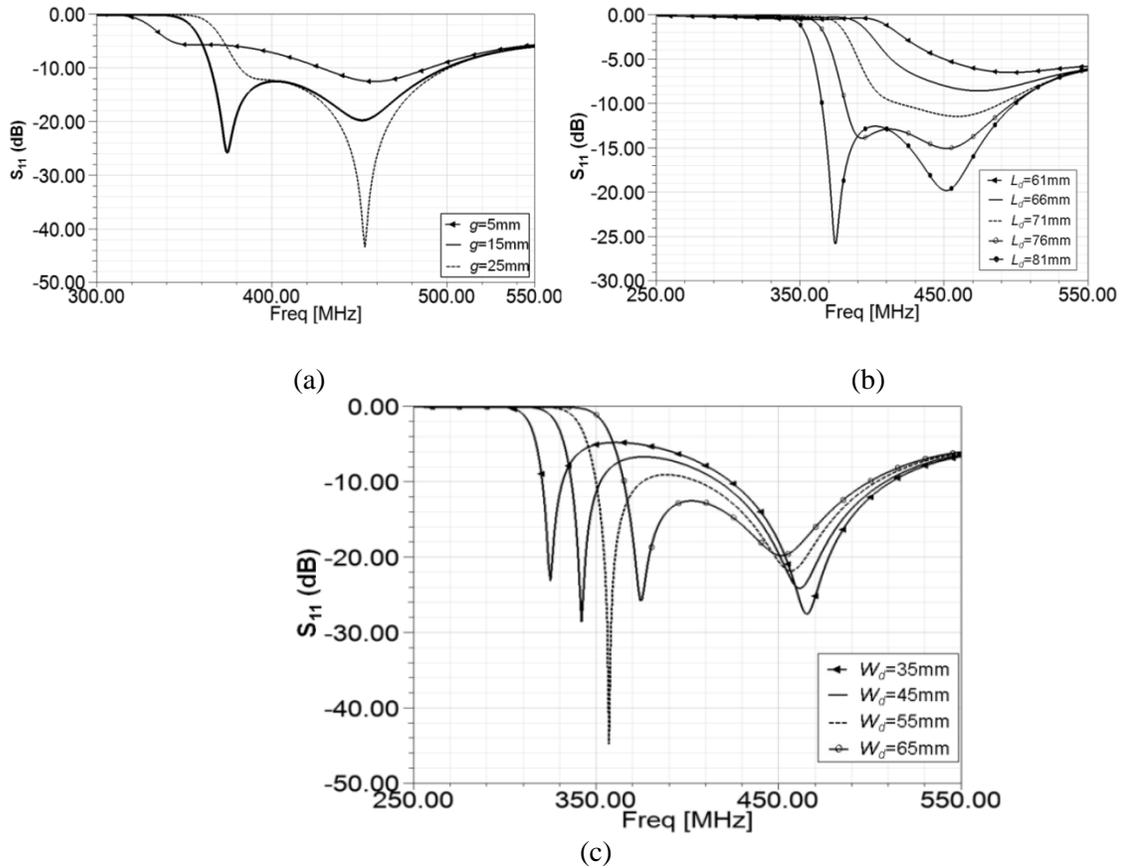
Figure 3.33: Simulated  $S_{11}$  as a function of (a)  $g$ , (b)  $L_d$  and (c)  $W_d$ .
