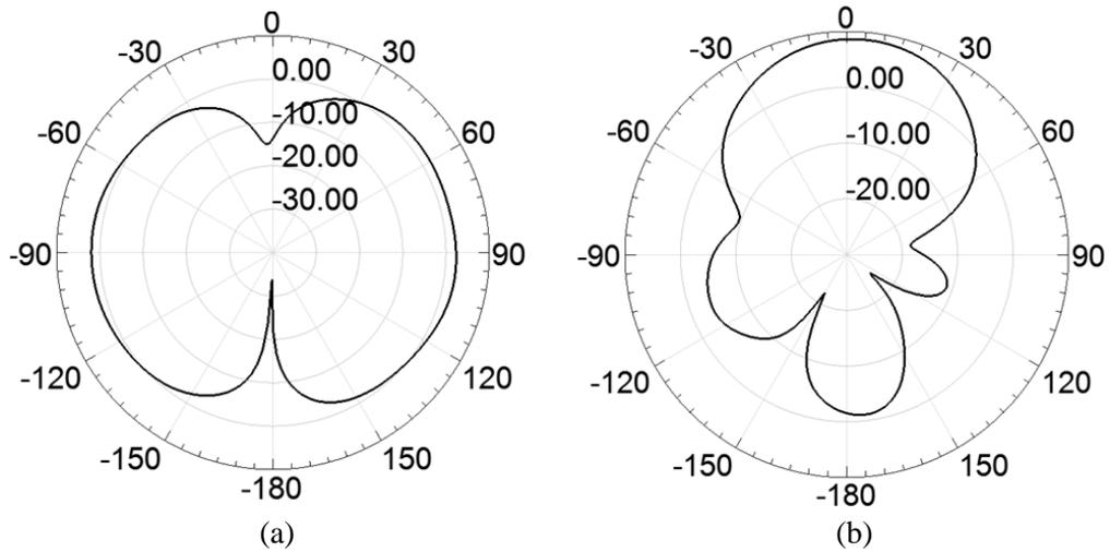
Figure 5.6: Simulated radiation patterns of the proposed bow-tie microstrip antenna on E-plane (xz-plane) at two resonant frequencies, corresponding to (a) PIFA and (b) patch operation shown Fig. 5.4.
