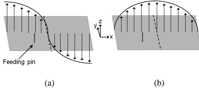
Figure 5.2: Distributions of (a) voltage and (b) current on the  $\lambda/2$  microstrip antenna with x-polarized radiation on the infinite ground plane.
