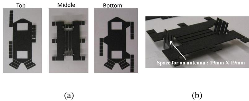
Figure 3.7: (a) Layout of Crawling Robot and (b) location and space for antenna.
