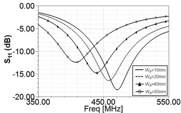
Figure 3.31: Simulated  $S_{11}$  of the modified folded monopole geometry as a function of width parameter  $W_b$  shown in Fig. 3.30.
