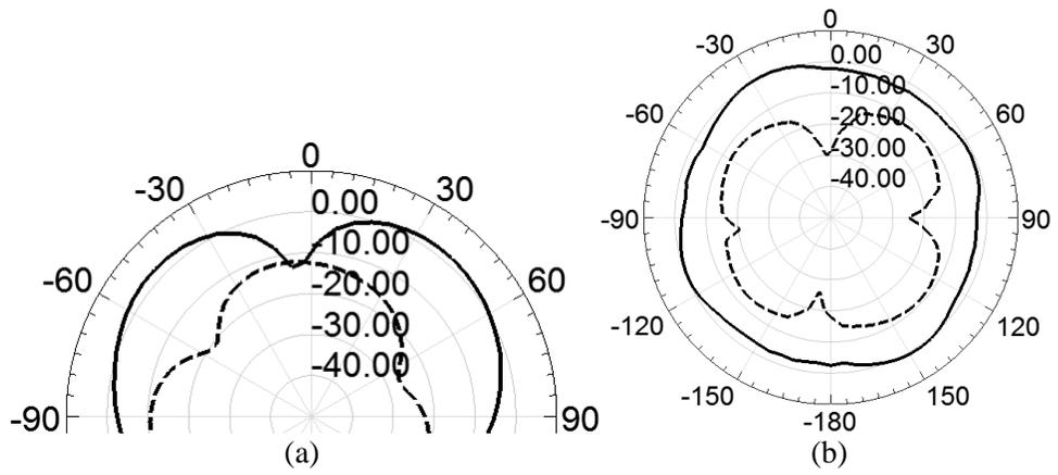
Figure 3.39: Measured radiation patterns of the proposed antenna at 430MHz: (a) E-Plane and (b) H-Plane.
