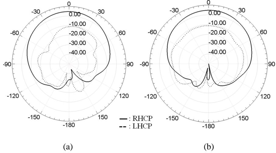
Figure 4.9: Simulated radiation patterns in two orthogonal planes of (a) xz and (b) yz-planes for the antenna shown in Fig. 4.7(a).
