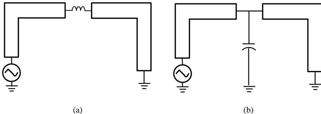
Figure 3.24: Folded monopole antennas with (a) a series inductor and (b) a shunt capacitor to excite the lower resonant frequency ( $f_{low}$ ).
