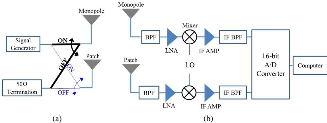
Figure A.9: Schematics of (a) the transmitter and (b) receiver utilizing the proposed diversity antennas.
