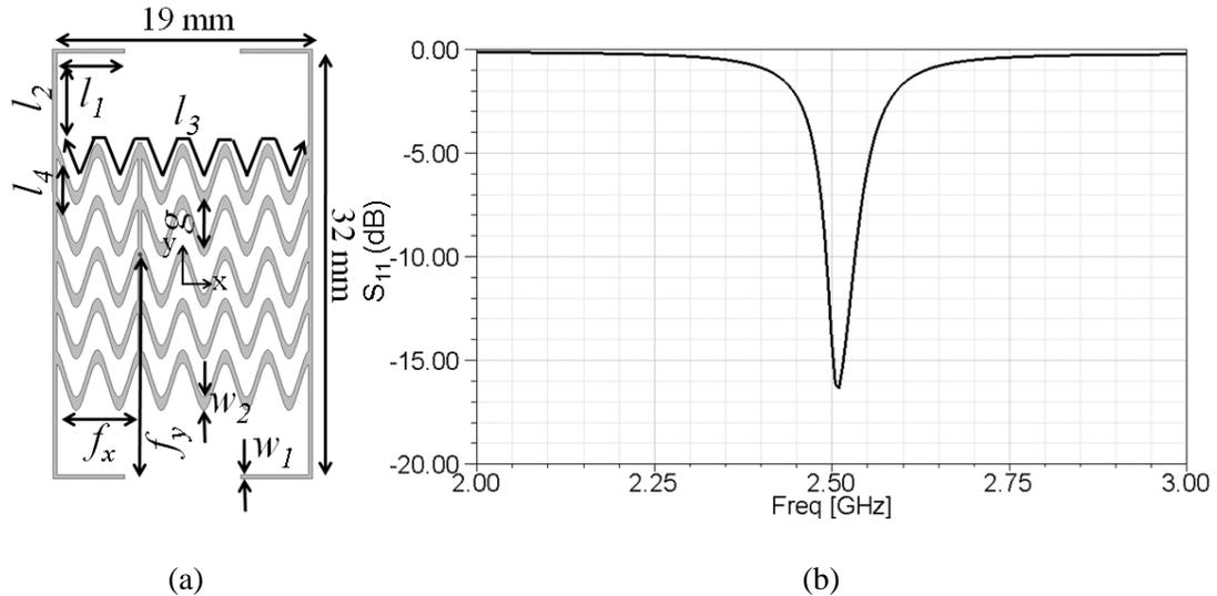
Figure 4.7: (a) Topology, design parameters and (b) simulated  $S_{11}$  of the proposed CP antenna exhibiting 59% size reduction as compared to the conventional corner-truncated square microstrip antenna.
