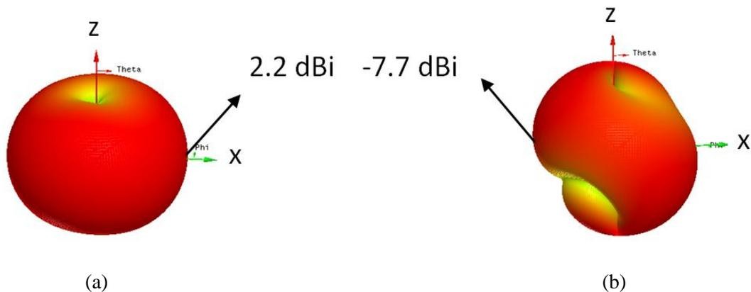
Figure 1.5: 3D radiation patterns corresponding to vertical polarization ( $E_\theta$ ) of (a) the straight  $\lambda/4$  monopole antenna and (b) meandered inverted-F antenna.
