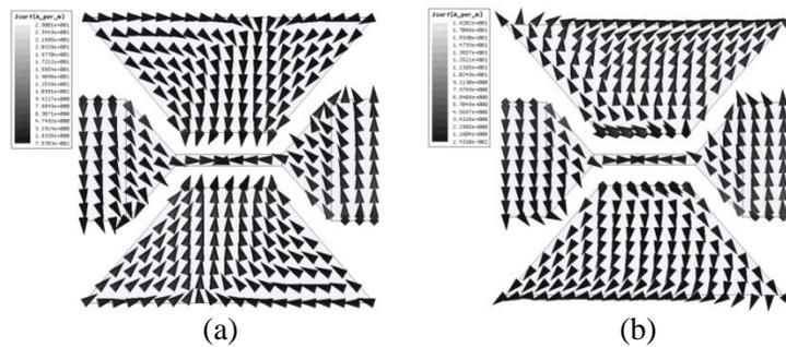
Figure 3.36: Horizontal electric current distributions at (a) 328MHz and (b) 419MHz.
