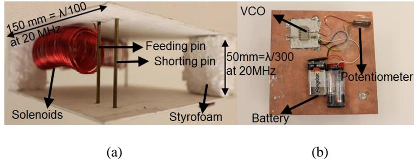
Figure 2.32: (a) Side view and (b) bottom view of the fabricated antenna incorporating air-core inductors, integrated with the source module.
