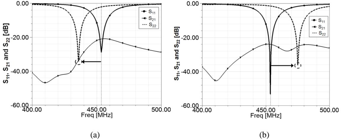
Figure 5.12: Simulated  $S_{11}$ ,  $S_{21}$  and  $S_{22}$  of the proposed polarization diversity antenna with 5mm
