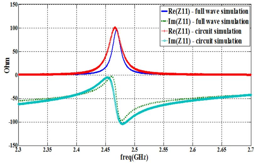
Figure 2.4: Real and imaginary parts of input impedance simulated by full wave and circuit simulators.
