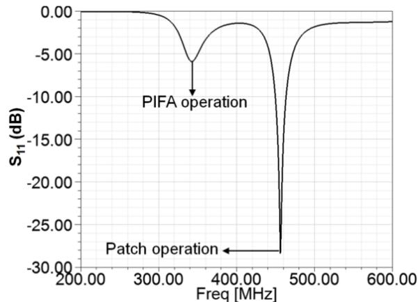
Figure 5.4: Simulated  $S_{11}$  of the proposed bow-tie microstrip antenna shown in Fig. 5.3.
