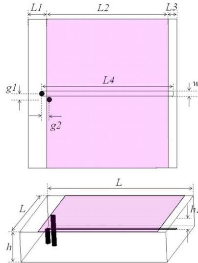
Figure 2.2: Design parameters of a multilayer ICCLMA.
