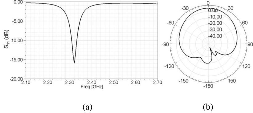
Figure 4.4: Simulated (a)  $S_{11}$  and (b) radiation pattern on xz-plane of the wired antenna depicted in Fig. 4.3(b).
