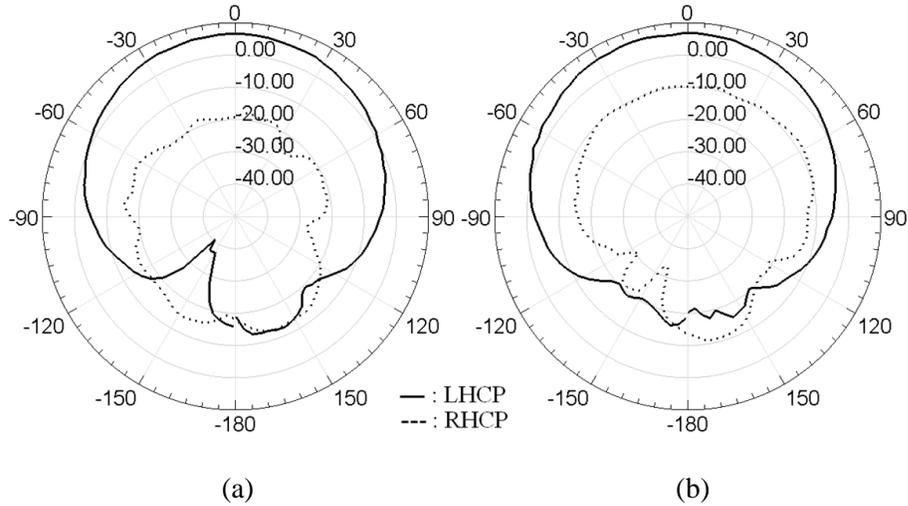
Figure 4.15: Measured radiation patterns in two orthogonal planes of (a) xz and (b) yz-planes for the antenna shown in Fig. 4.13(a).
