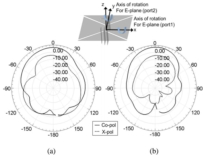
Figure 5.15: Measured radiation patterns on E-planes of two bow-tie microstrip antennas: (a) Port1: ON and Port2: OFF ( $50\Omega$  terminated) and (b) Port1: OFF ( $50\Omega$  terminated) and Port2: ON.
