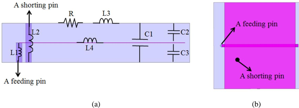
Figure 2.1: (a) Equivalent circuit model drawn in side view and (b) top view of a multilayer ICCLMA.
