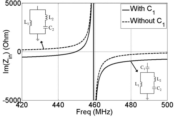
Figure 3.26: Imaginary part of  $Z_{in}$  in the equivalent circuit model of the capacitively coupled parasitic element shown in Fig. 3.25(b), compared to the same circuit model without  $C_1$ .
