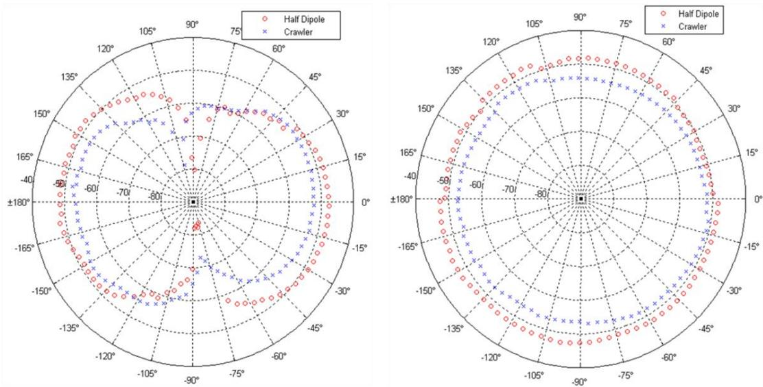
Figure 3.20. Measured (a) E-planes and (b) H-planes of  $\lambda/2$  dipole and proposed antennas.
