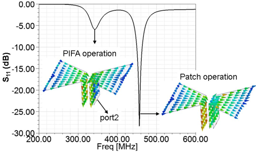
Figure 6.4:  $S_{11}$  and electric surface current distributions at two modes of the proposed microstrip antenna.
