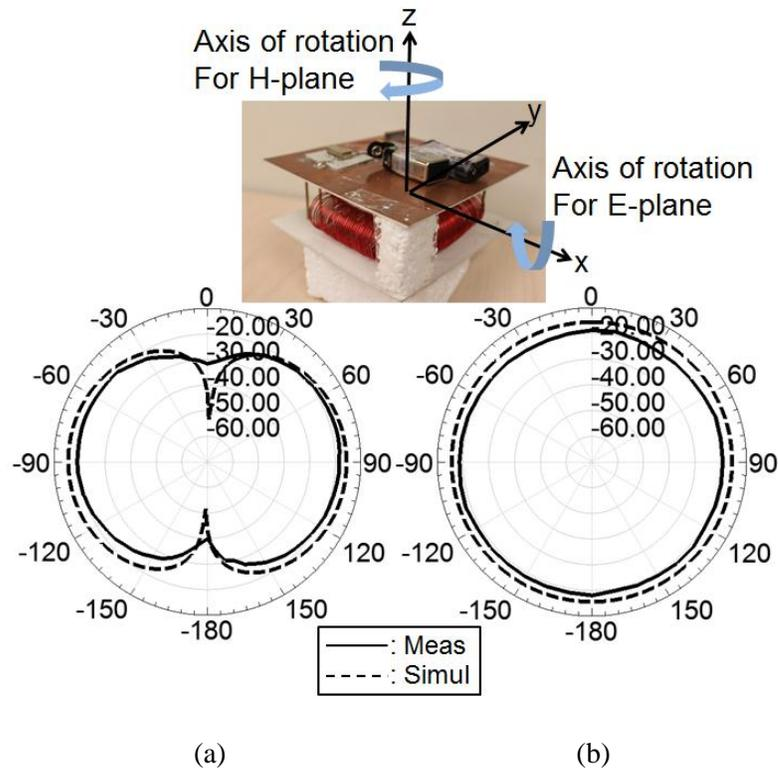
Figure 2.35: Measured and simulated radiation patterns of the proposed antenna with air-core inductors in the (a) E (=yz) plane and (b) H (=xy) plane.
