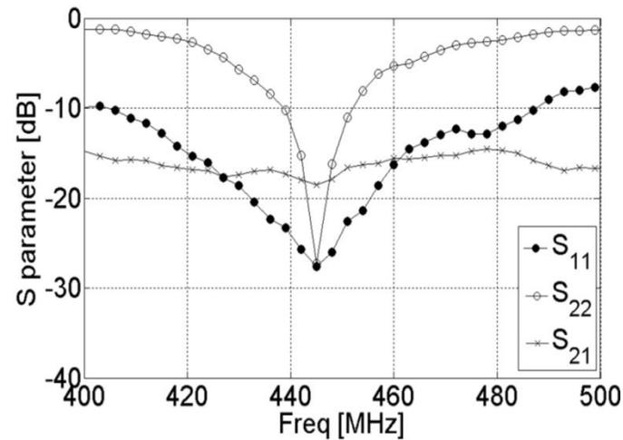
Figure 5.19: Measured  $S_{11}$ ,  $S_{21}$  and  $S_{22}$  of the proposed pattern diversity antenna.
