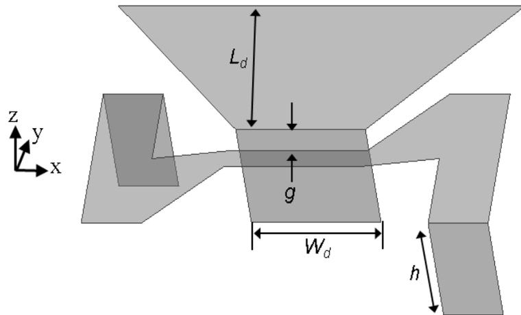
Figure 3.32: Geometry and design parameters of the meandered  $\lambda/2$  folded monopole antenna with the capacitively coupled parasitic element.
