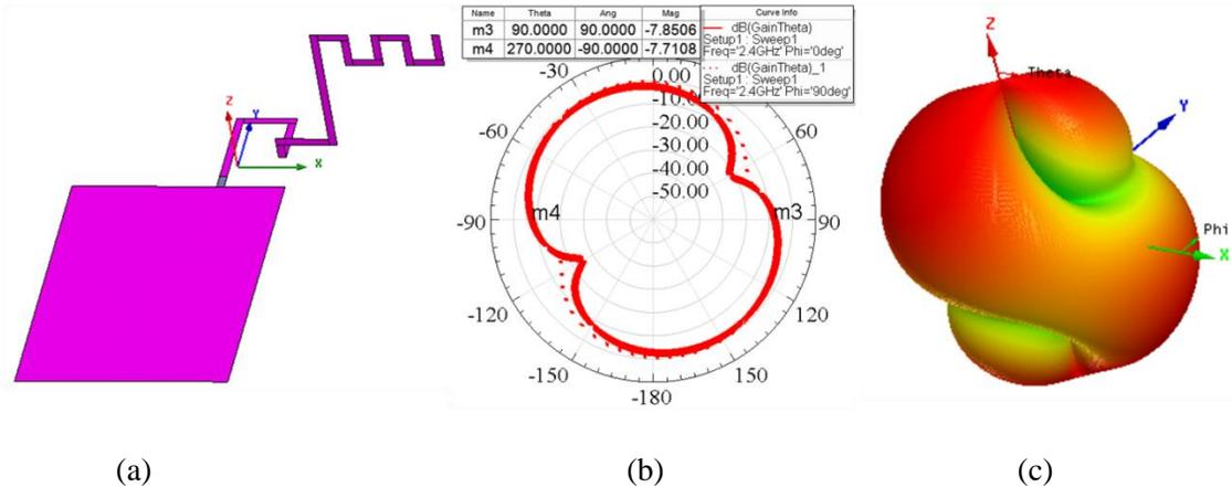
Figure 3.9: (a) Meandered monopole antenna, (b) 2D and (c) 3D radiation pattern of v-pol.
