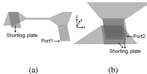
Figure 5.16: (a) Folded monopole antenna with omnidirectional radiation pattern and (b) proposed bow-tie microstrip antenna with broadside radiation pattern.
