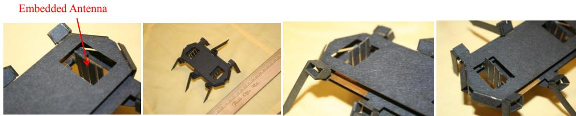
Figure 3.21: Embedded antenna inside a crawler robot.
