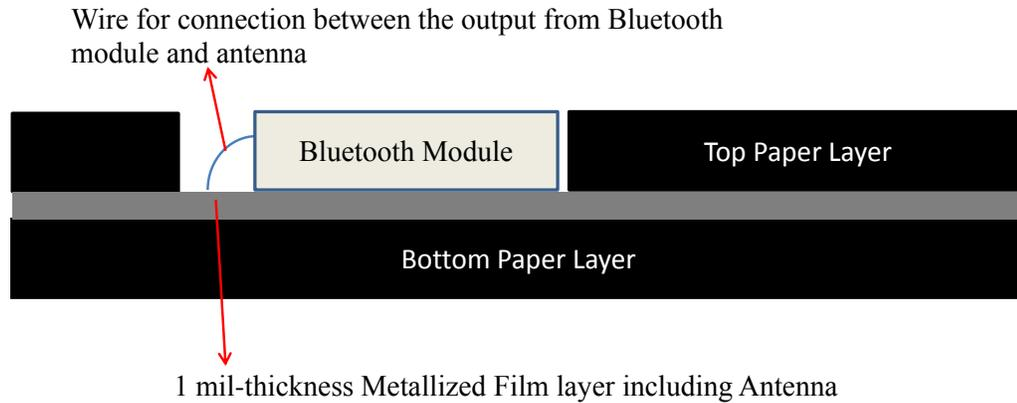
Figure 3.22: Integration of embedded antenna in thin paper with Bluetooth module.
