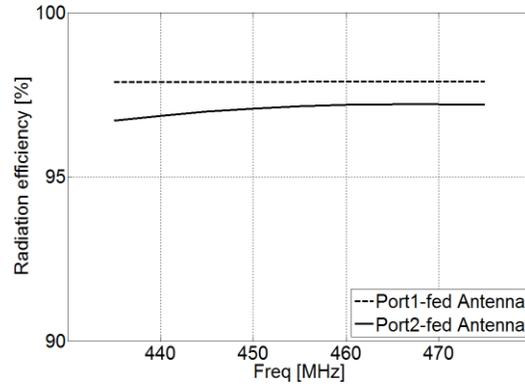
Figure 5.20: Simulated radiation efficiency of two antenna elements in the proposed pattern diversity antenna.
