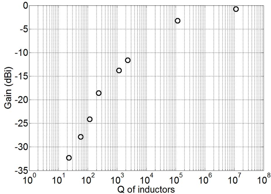
Figure 2.28: Simulated gains of the proposed antennas with chip inductors versus Q of the chip inductors.
