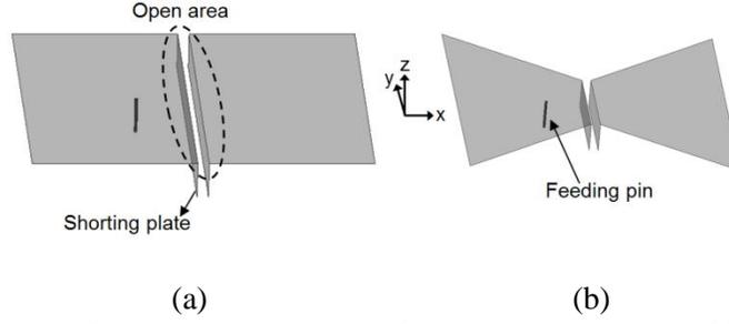
Figure 5.1: (a) Proposed microstrip antenna with an open area in its middle and (b) bow-tie version of the proposed microstrip antenna on the infinite ground plane.
