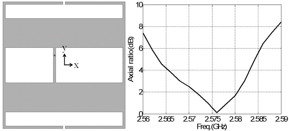
Figure 4.14: Measured axial ratio in the broadside direction for the antenna shown in Fig. 4.13(a).
