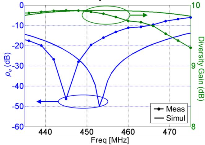
Figure 5.21: Envelop correlation ( $\rho_e$ ) between radiation patterns of two antenna elements in the proposed pattern diversity antenna and diversity gain.
