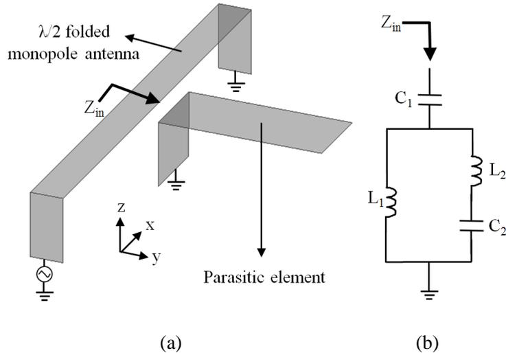
Figure 3.25: (a) Side view of  $\lambda/2$  folded monopole antenna with a capacitively coupled parasitic element and (b) equivalent circuit model of the parasitic element.
