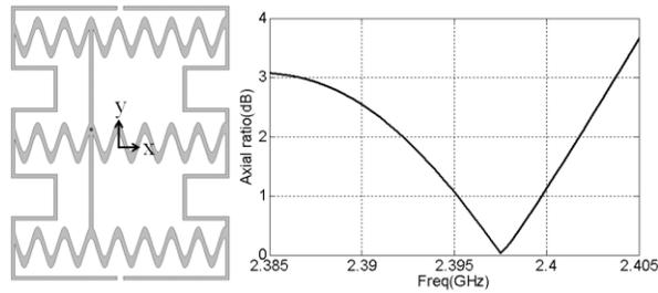
Figure 4.11: Simulated axial ratio in the broadside direction for the antenna shown in Fig. 4.10(a).
