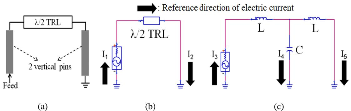
Figure 2.15: (a) Two vertical elements put  $\lambda_0/2$  away from each other, (b) its circuit model and (c) a circuit model for the conventional T-type 180 degree phase shifter.
