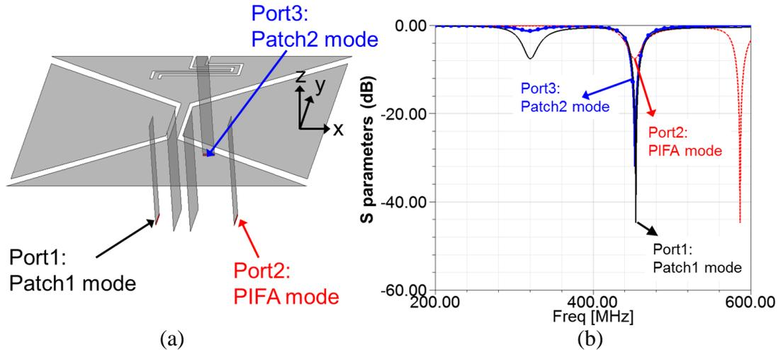
Figure 6.5: Expected (a) topology of the 3-element diversity antenna and (b)  $S_{11}$ ,  $S_{22}$  and  $S_{33}$ .
