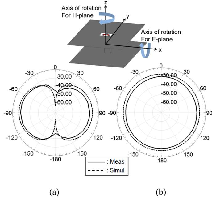
Figure 2.23: Measured and simulated radiation patterns of the proposed antenna with chip inductors in the (a) E (=yz) plane and (b) H (=xy) plane.
