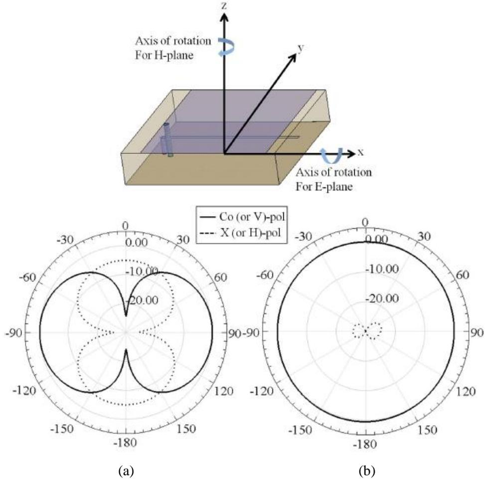
Figure 2.6: Simulated (a) E-Plane and (b) H-Plane radiation patterns when  $L = \lambda_0/8$  and  $h = \lambda_0/40$
