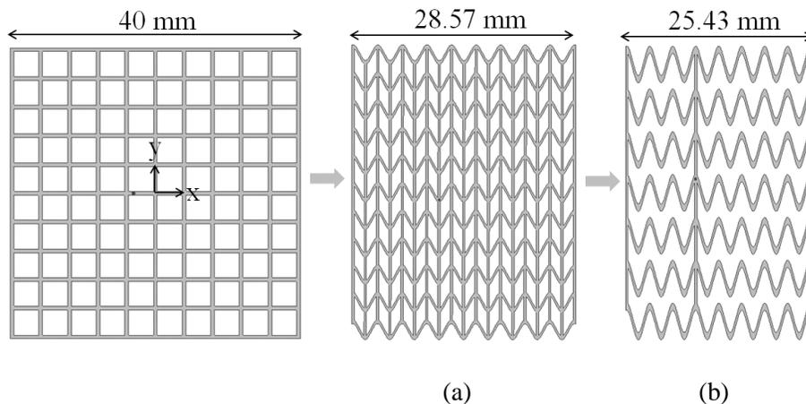
Figure 4.3: (a) Shrunken wires and (b) sinusoidal wires with the elimination of wires in parallel with y-axis.
