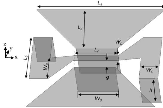
Figure 3.34: Geometry and design parameters of the omnidirectional antenna topology with two back-to-back parasitic elements.
