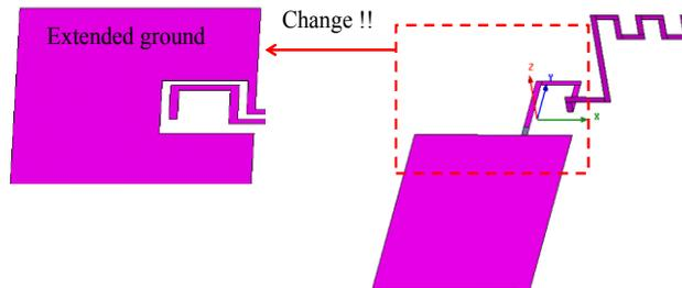
Figure 3.10: Suppression of radiation from horizontal current using extended ground.
