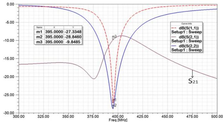
Figure A.5: Simulated S parameters of the proposed radiation pattern diversity antenna.
