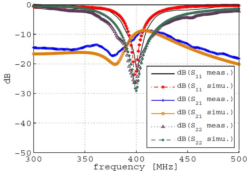
Figure A.8: Simulated and measured S parameters of the proposed pattern diversity antenna
