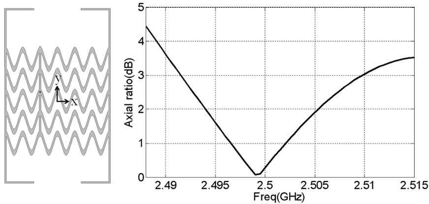
Figure 4.8: Simulated axial ratio in the broadside direction for the antenna shown in Fig. 4.7(a).
