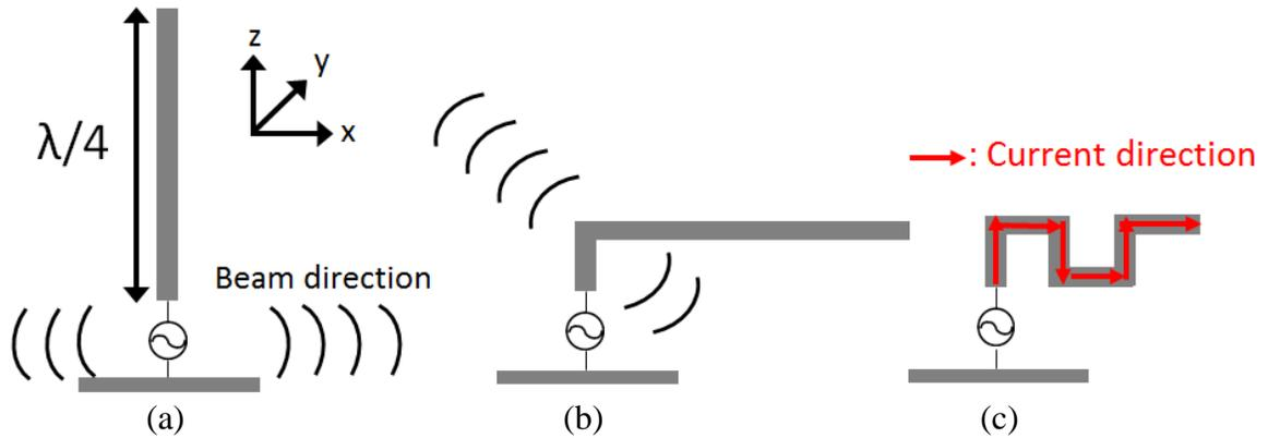
Figure 1.4: Side views of (a) straight  $\lambda/4$  monopole antenna, (b) inverted-F antenna and (c) meandered inverted-F antenna on small ground plane.
