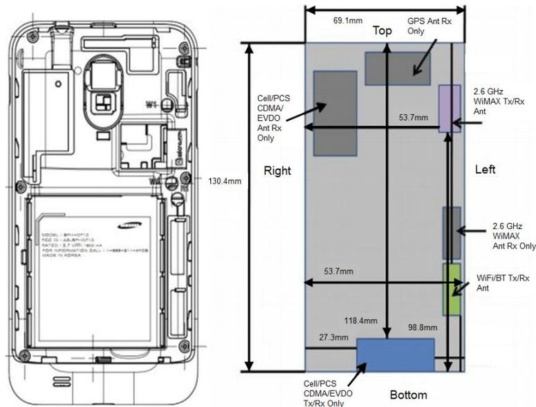
Figure 1.3: Antenna dimensions and locations on the Samsung Galaxy S [4].
