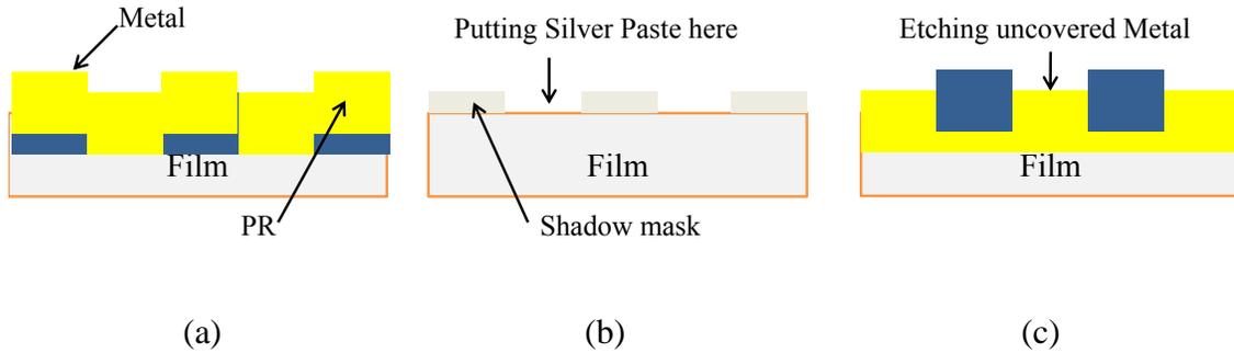
Figure 3.14: (a) Lift-off, (b) Shadow mask, and (c) Etch-back.
