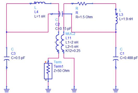
Figure 2.3: Equivalent circuit model of a multilayer ICCLMA.
