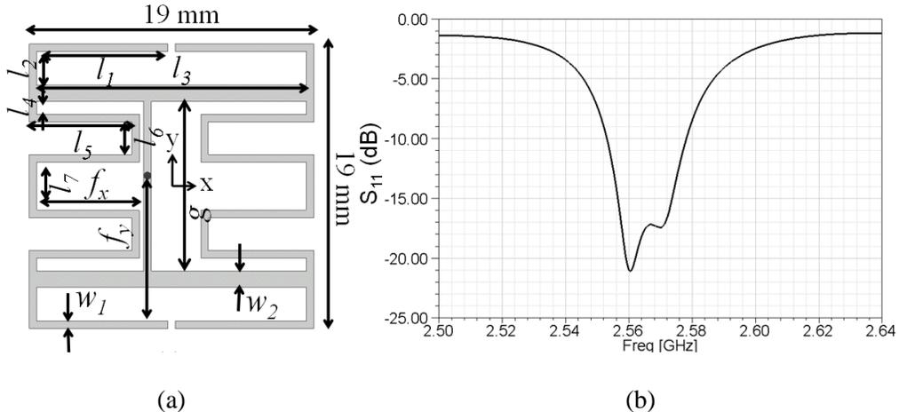
Figure 4.16: (a) Topology, design parameters and (b) measured  $S_{11}$  of the proposed CP antenna exhibiting 75% size reduction as compared to the conventional corner-truncated square microstrip antenna.
