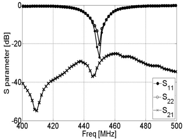
Figure 5.11: Measured  $S_{11}$ ,  $S_{21}$  and  $S_{22}$  of the proposed polarization diversity antenna.
