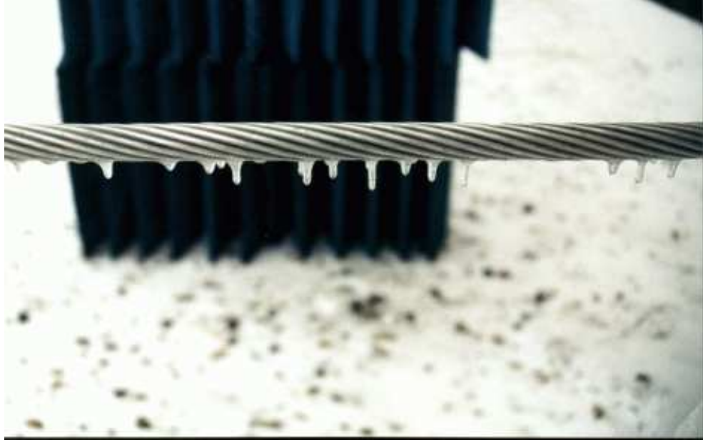
Figure 2.8: A picture of power line #2 covered with a layer of ice(thickness \approx 1 mm) during the backscatter measurements.
