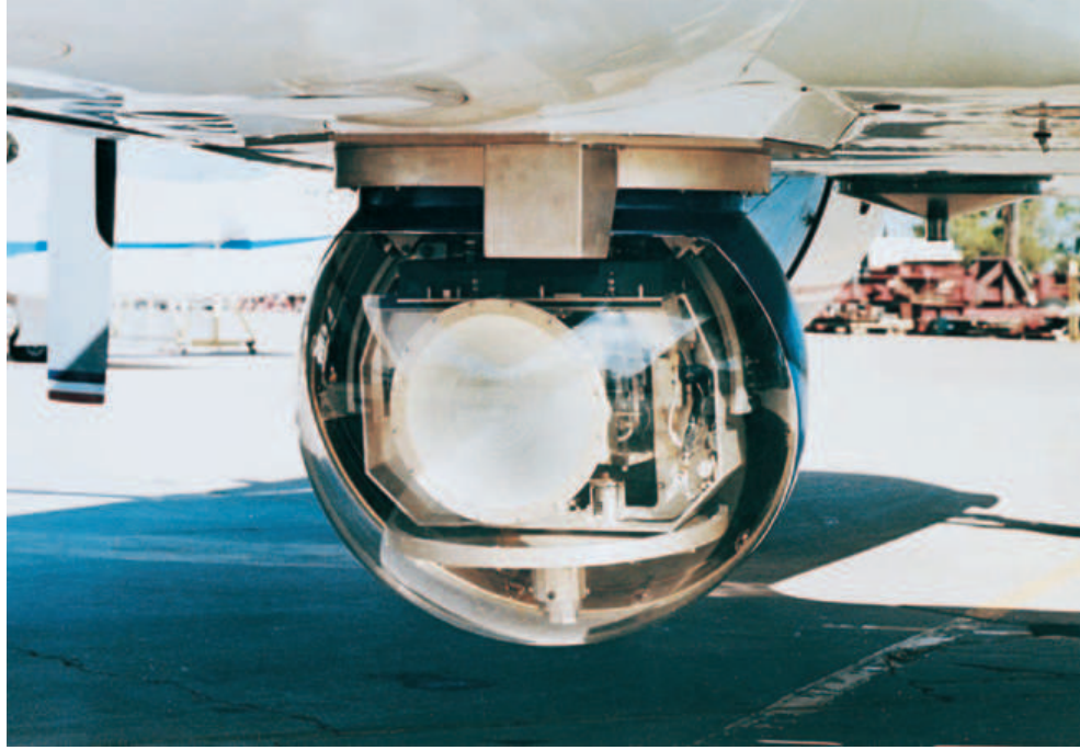
Figure 4.10: The Lincoln Laboratory's Ka-Band high-resolution fully polarimetric Synthetic Aperture Radar (SAR) used to collect the SAR imageries used in this work. The radar is mounted below a fuselage of a Gulfstream aircraft. System parameters: frequency 33 GHz, resolution (SAR) 1 \text{ ft} \times 1 \text{ ft} , beamwidth 2^\circ , polarization isolation 1000/1, sensitivity (SAR mode) (7 km range) S/N = 10 for 0.001 \text{ m}^2 RCS.
