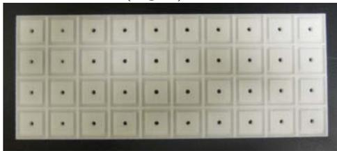
Figure 4.14: Top-view of one of the Rohacell trays.
