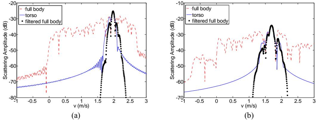
Figure 3.14. Temporal backscattering response of torso and the full body at two instances: (a) the limbs are spread out and the spectrum is narrow. (b) the limbs are aligned with the body and the spectrum is wide. The filtered response of the full body resembles that of the torso at both instances.
