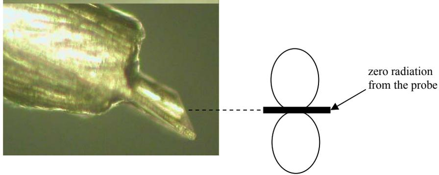
Figure 8.12. Radiation pattern of the GSG probe.
