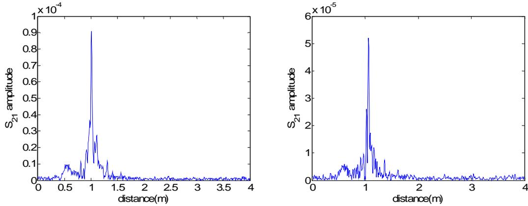
Figure 8.17. The time domain response at two different spots on top of the slots.
