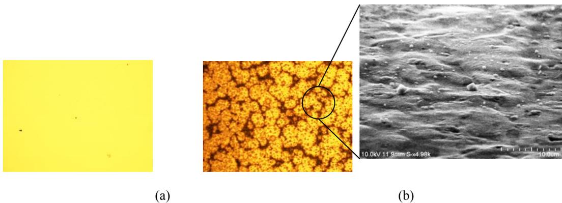
Figure 8.19. Etched area of the bottom wafer (a) before and (b) after bonding. The SEM photo in the inset shows around 5~10  $\mu\text{m}$  roughness.
