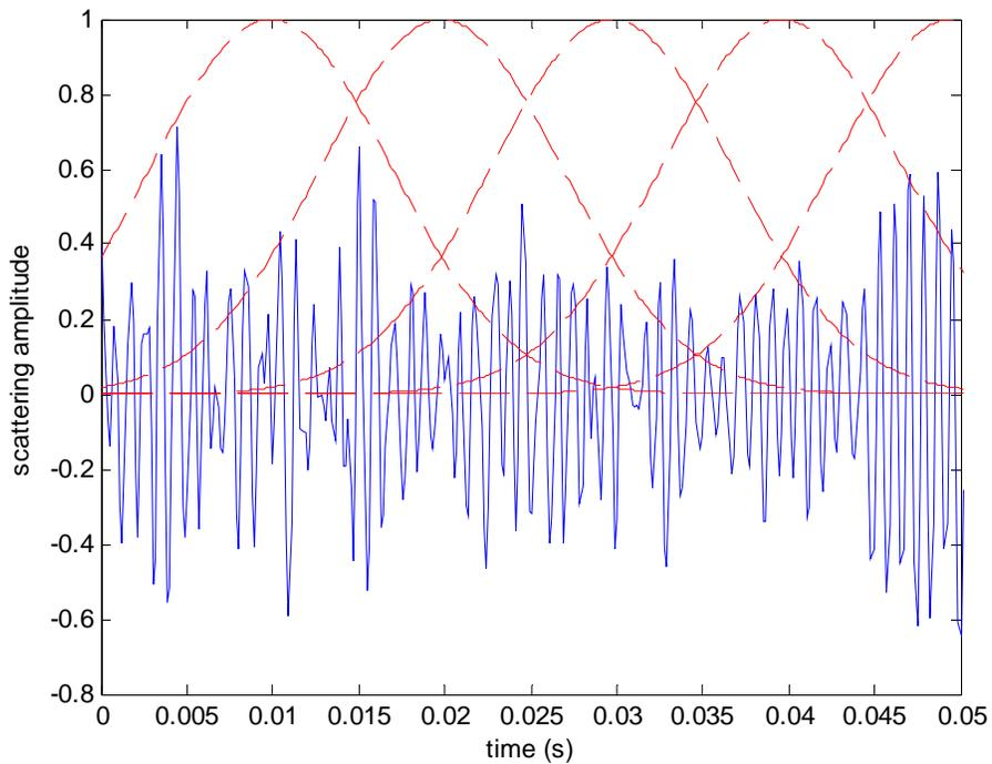
Figure 3.12. The signal is multiplied by a number of shifted Gaussian functions.
