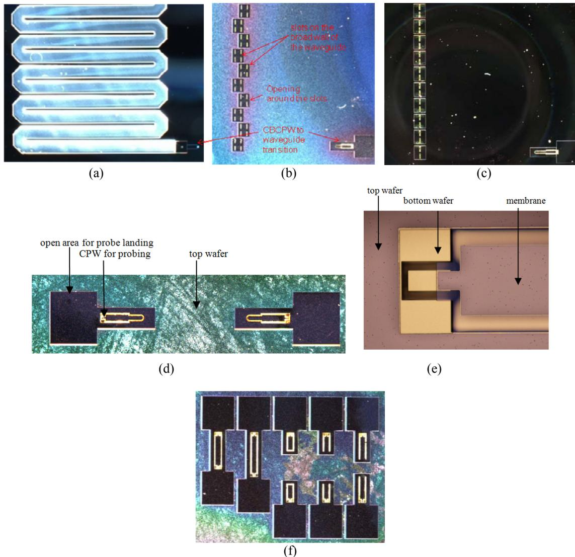
Figure 7.9. (a) First wafer before bonding. (b) the meander-line slot antenna after bonding, (c) the low-loss design (d) the CBCPW/waveguide transition, (e) the CPW/CBCPW transition, (f) calibration standards, from left to right: thru, line, open, short, offset short.
