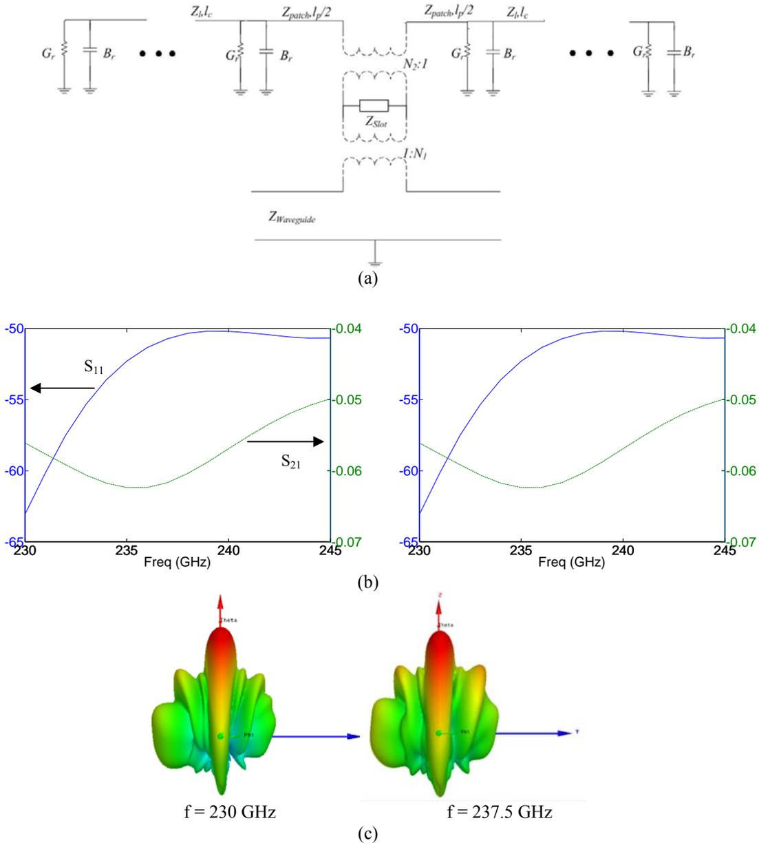
Figure 5.11. (a) equivalent circuit model of the hybrid-coupled patch array, (b) directivity of the hybrid-coupled patch array and the S-parameters of the waveguide for the center patch length of 380  $\mu\text{m}$ . The lengths of the center patch and connecting line to the series-fed array are optimized in such a way that the directivity is maximized and the S-parameters show resonance and (c) far-field radiation pattern of the antenna.
