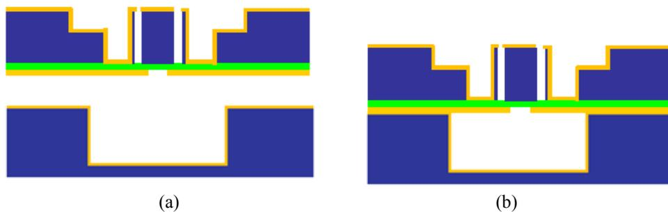
Figure 7.11. First and second wafers. (a) before gold-gold thermocompression bonding (b) after bonding
