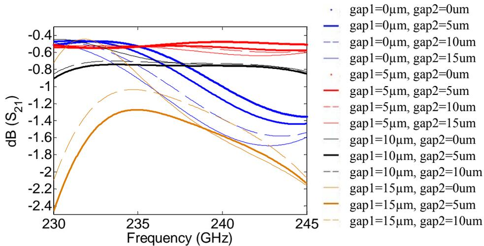
Figure 6.17. The transmission coefficient of the back-to-back transition in Figure 5 (a) for different gap values.
