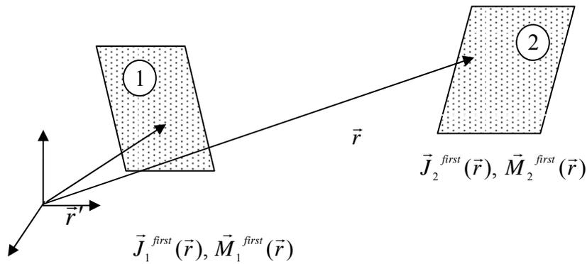
Figure 2.11. The interaction between two flat facets.
