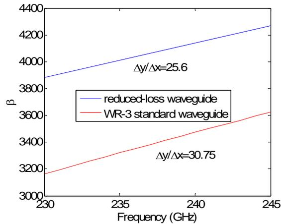
Figure 5.21. The dispersion diagram: propagation constant ( $\beta$ ) versus frequency. The slope is decreased for the reduced-loss waveguide
