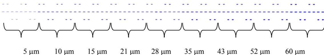
Figure 5.8. The slot width for each four turns so that nine different widths are used for the 36 turn waveguide. The length of the slots is 380  $\mu\text{m}$ .
