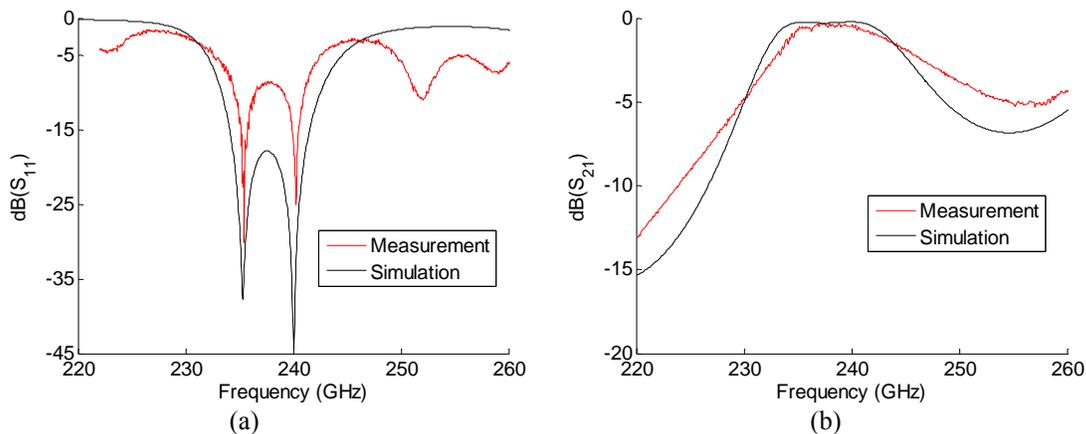
Figure 8.4. The measured (a) reflection and (b) transmission coefficient of the filter shown in Figure 6.19 compared to the full-wave simulation. The nulls of the filter are precisely detected and the results are in good agreement with the simulation.
