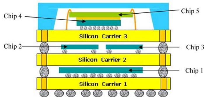
Figure 4.6. Schematic of 3-D silicon stacked carrier SiP [63]. Chips 1 to 4 are connected with the flip-chip method and chip 5 with wire bonding.
