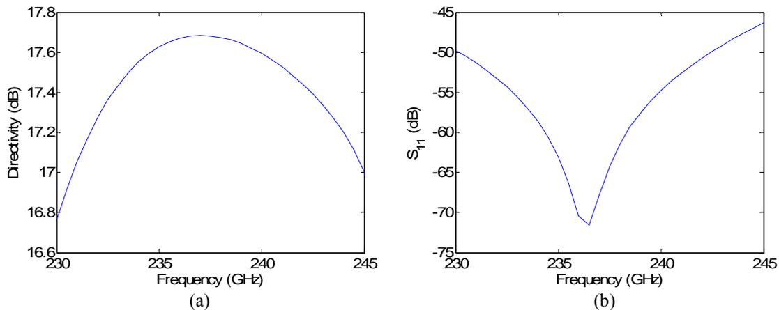
Figure 5.16. (a) The directivity and (b) return loss versus frequency of the patch array of Figure 5.15.  $l_r = 950 \mu\text{m}$
