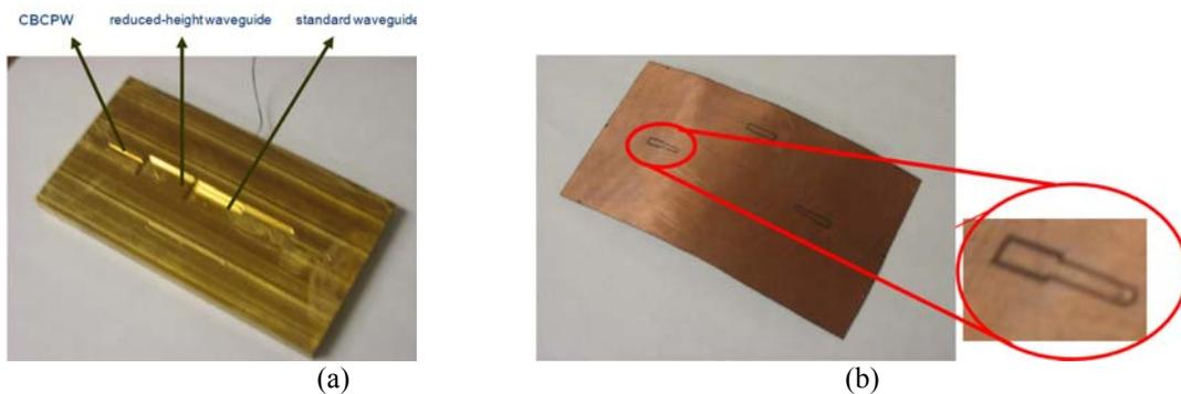
Figure 6.9. (a) The CBCPW trench, reduced-height waveguide and the standard waveguide are machined on a brass plate. (b) the top cover includes the lines is a substrate whose both sides are etched with CPW patterns.
