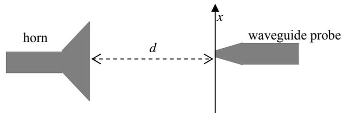
Figure 8.8. Measurement setup for the near-field measurement of the E-plane horn.
