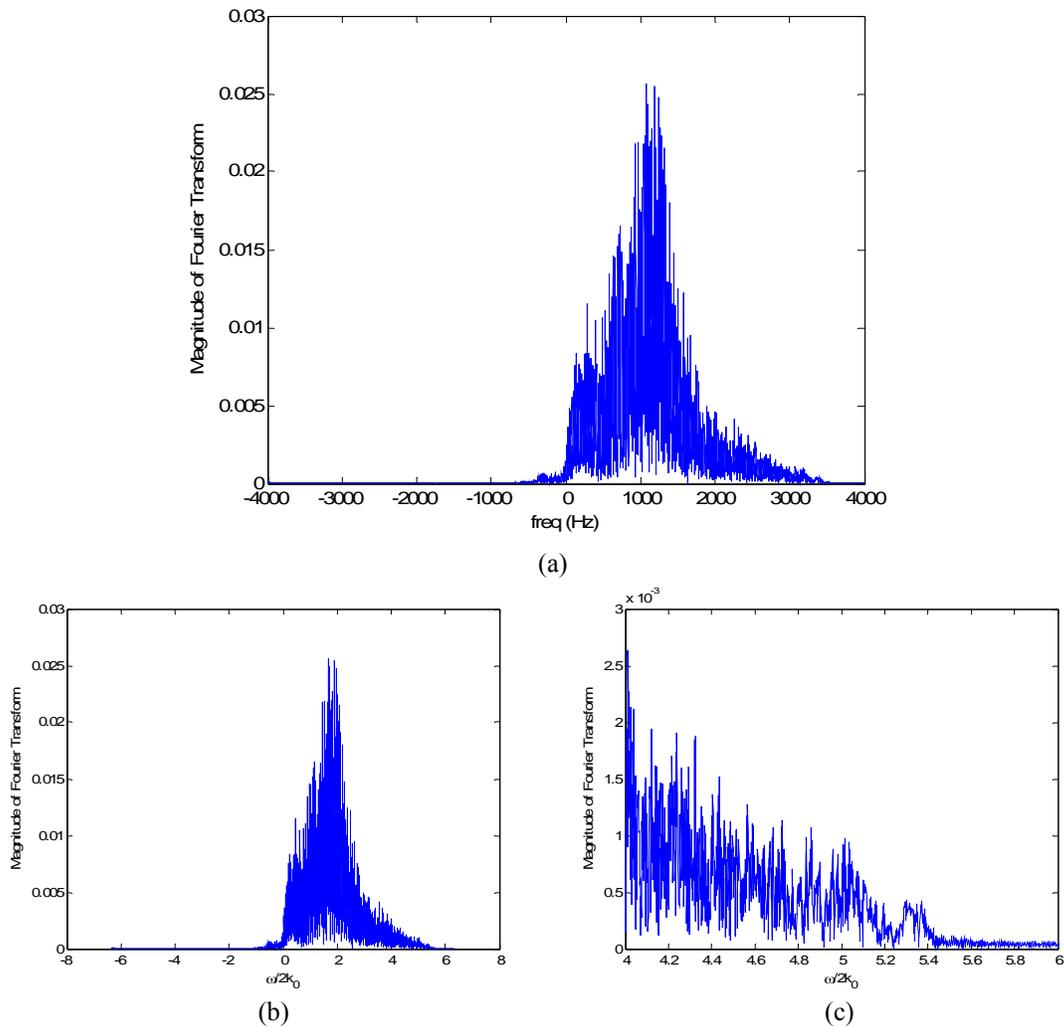
Figure 3.3. (a) Fourier transform of scattering amplitude of human walking. (b) Fourier transform of scattering amplitude of human walking versus  $\omega_0/(2k_0)$  to give the velocities. It can be seen that it has peaks around its average velocity ( $v=1.8$  m/s) from 1.4 to 2.1m/s. (c) the extended plot to find maximum velocity which is approximately 5.3m/s.
