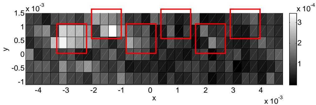
Figure 8.15. (a) The  $S_{21}$  intensity measured over the slot openings.
