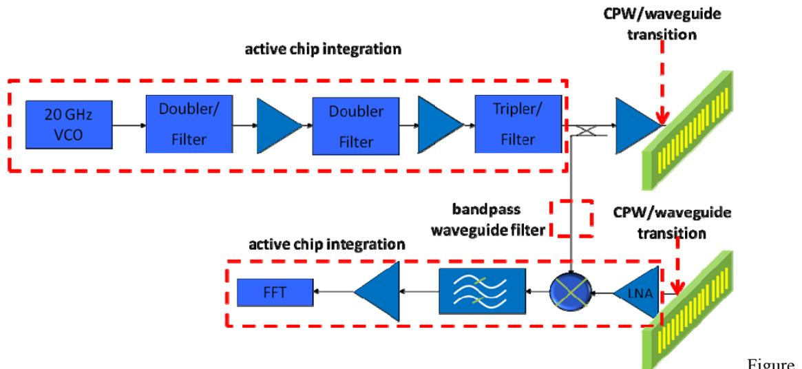
Figure 6.1. The passive components for radar integration are highlighted in the radar block diagram. These components include CPW/waveguide transition, bandpass waveguide filters and active chip packaging.
