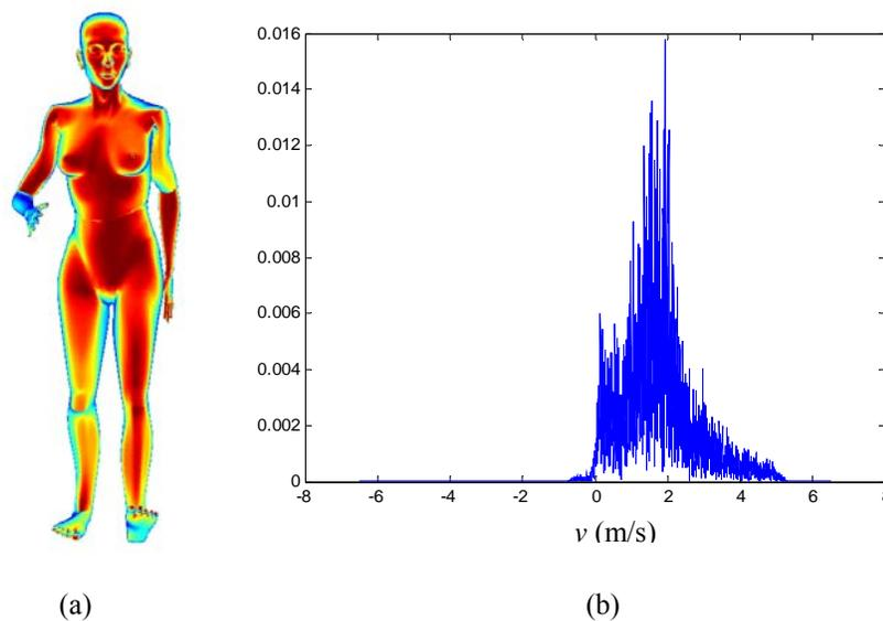
Figure 3.19. (a) The qualitative current distribution on human body and (b) the Doppler spectrum of walking at 240 GHz.
