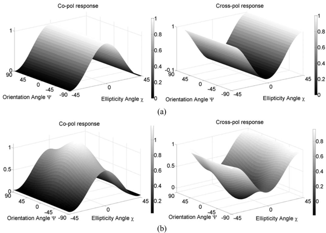
Figure 3.9. (a) Polarization response of sphere and (b) torso.
