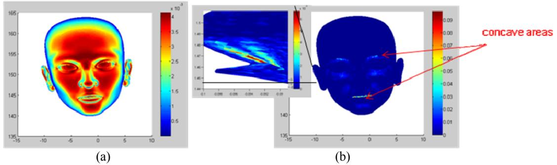
Figure 2.15. (a) first and (b) second order current distribution on human head. First order currents are distributed almost everywhere which is not shadowed and have larger amplitudes in the areas which are more perpendicular to the direction of propagation. Second order currents are concentrated on concave and irregular parts.
