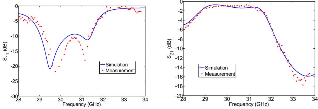
Figure 6.11. Simulation results of a structure with misalignments (300  $\mu\text{m}$  translational displacement) between the top substrate and the brass unit compared to the measured results. The transmission is decreased for frequencies lower than 29 GHz and the impedance match near 31 GHz is not as good as that of the optimized
