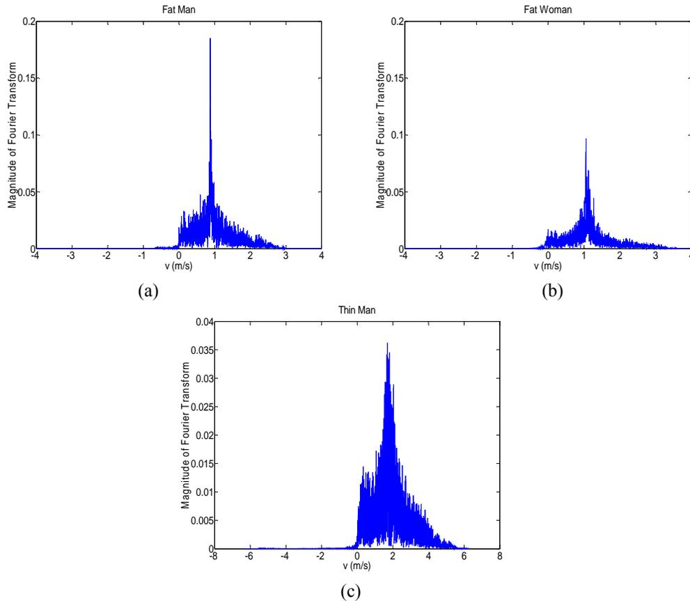
Figure 3.5. Doppler spectra of walking bodies with different sizes and genders. (a) oversized male body (b) oversized female body and (c) thin male body.
