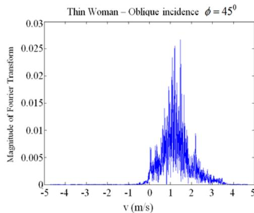
Figure 3.6. Doppler spectrum of a thin woman obliquely walking with respect to the radar with  $45^\circ$  angle. It is observable that the velocity content is lower, the maximum velocity is 3.8 (which is  $5.4/\sqrt{2}$ ) as expected). However, it is definitely not an oversized body since the energy is not highly concentrated around the average velocity.
