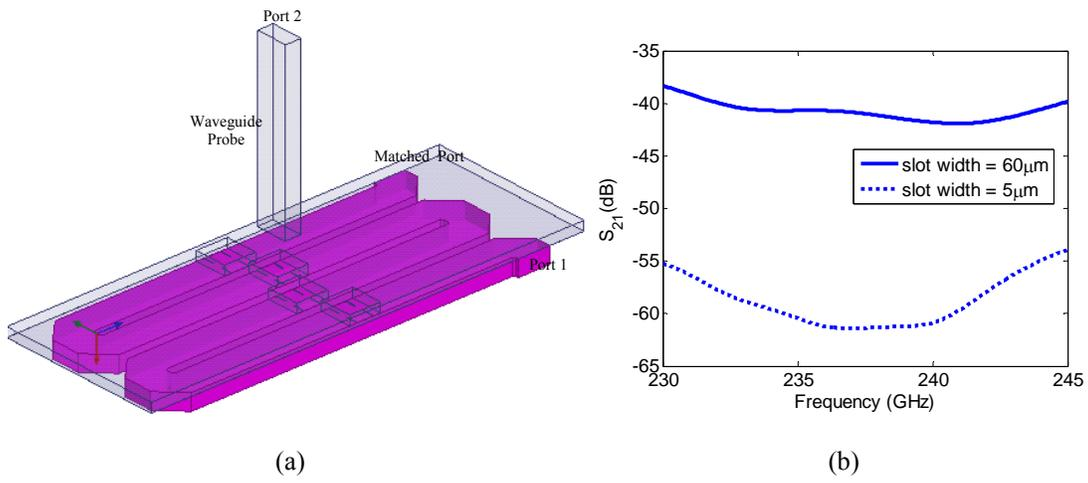
Figure 8.13. The structure simulated to calculate the power radiated from the slots
