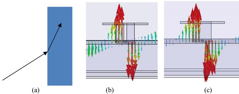
Figure 5.13. (a) Electric field at the boundary of two dielectric materials. The electric field distribution under a patch element excited from a very thin slot far from the patch element assisted by (b) high dielectric vertical walls (c) dielectric block.
