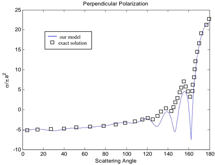
Figure 2.9. Normalized RCS of a lossy sphere with  $\epsilon_r = 5 + j10$  and  $a = 2\lambda$  for perpendicularly polarized incident wave compared with exact solution (Figure 3.21 in [29]).
