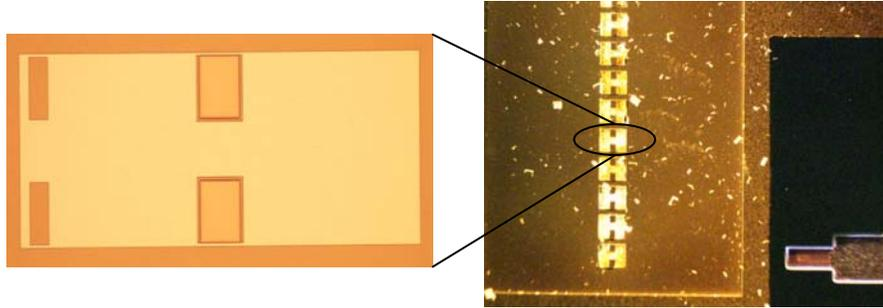
Figure 7.12. Fabricated patch array substrate
