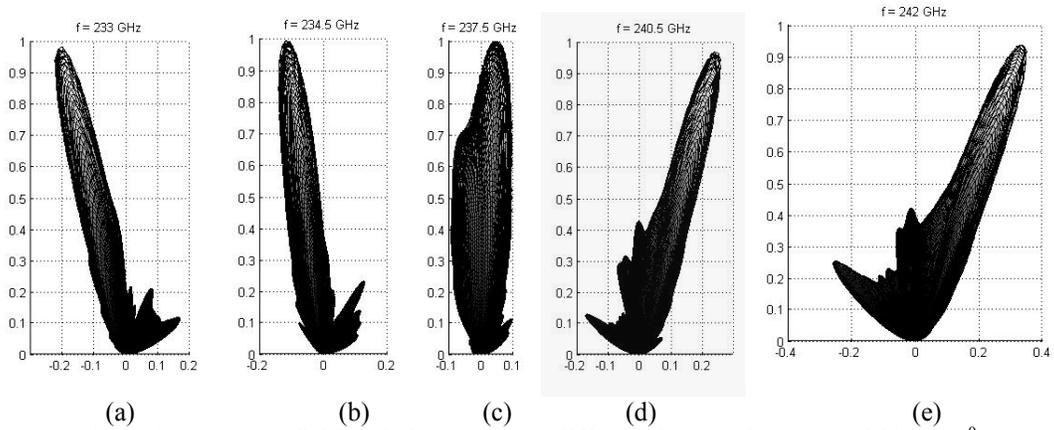
Figure 8.18. (a) Far-field radiation pattern at different frequencies, beamwidth =  $8.5^\circ$ .
