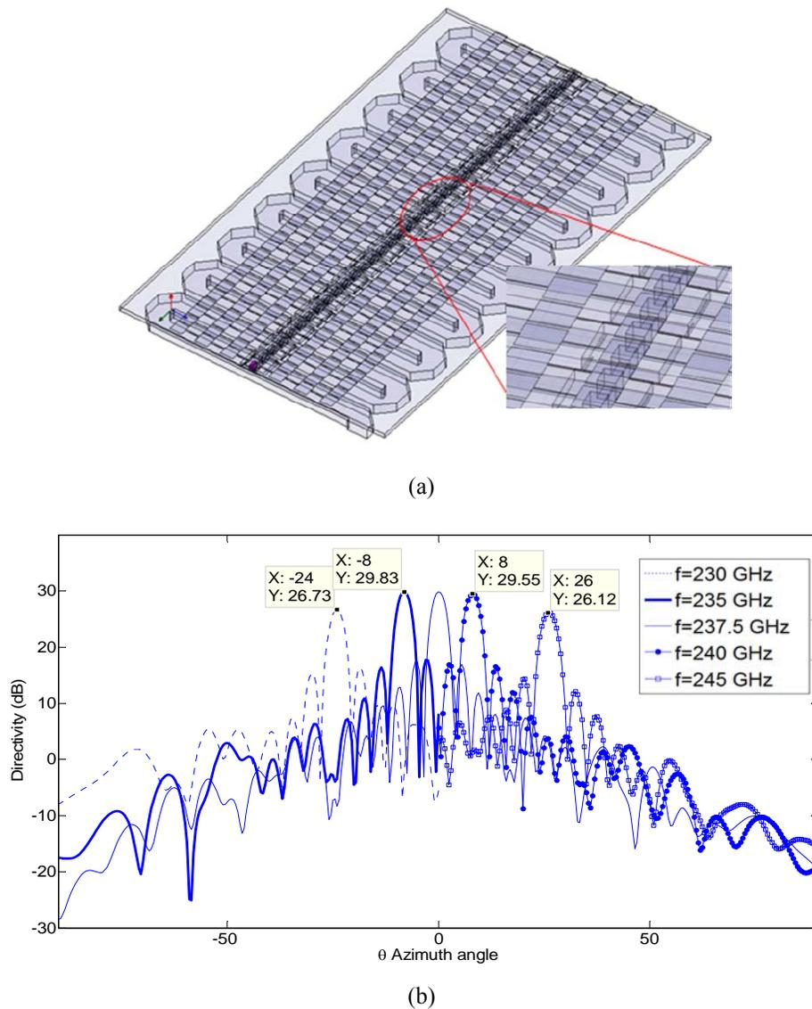
Figure 5.17. (a) The final structure (b) the radiation pattern in azimuth direction to verify the frequency scanning.
