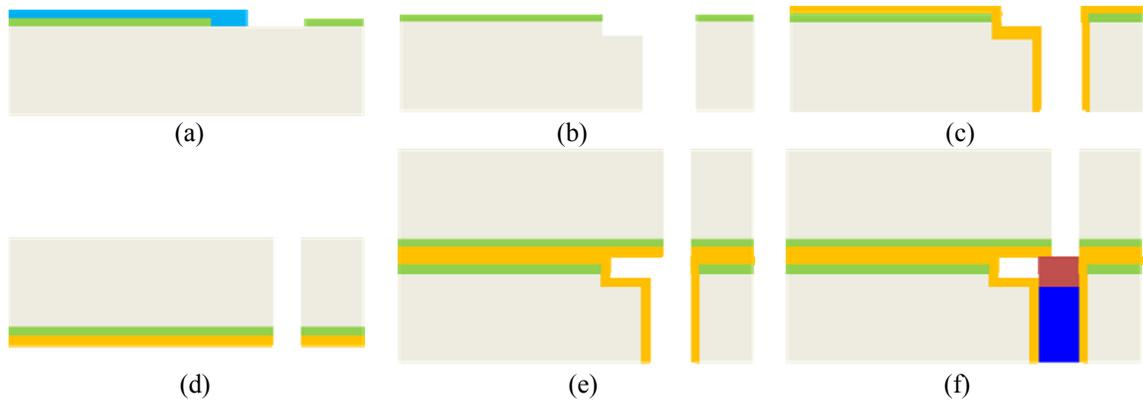
Figure 7.17 Fabrication process of the transition between the chip and the CBCPW. (a) two-step patterning (b) two step etching (c) gold sputtering for the first wafer. (d) top wafer (membrane, line patterns and etching the open areas). (e) top-bottom wafers gold bonding. (f) inserting the chip inside.
