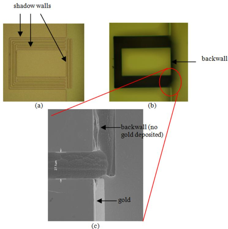
Figure 7.4. The grooved CPW (a) before (b) after removing the shadow walls. (c) SEM photo of the backwall (tilted  $200^\circ$ ) which verifies that the shadow walls prevented gold deposition effectively.
