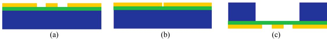
Figure 7.6. Second wafer fabrication process. A stacked layer of LPCVD SiO<sub>2</sub>/Si<sub>3</sub>N<sub>4</sub>/SiO<sub>2</sub> (ONO) as a membrane followed by gold is deposited. Then gold is patterned with the mask of (a) CPW and CBCPW lines. (b) the slots. (c) The wafer is flipped over and the backside is etched from the top of the areas around CBCPW and slots.
