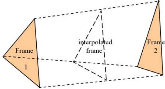
Figure 2.5. Linear interpolation is performed between each two adjacent facets from each frame in order to estimate the “in-between” frames.
