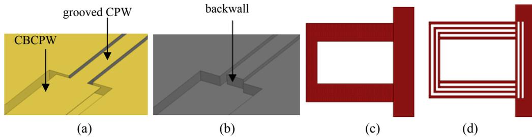
Figure 7.3. (a) The schematic of the transition from grooved CPW to the CBCPW (b) Bottom substrate with top layer removed. The backwall shown in (b) should not be covered with gold (c) Top view of very short section of grooved CPW (d) the proposed structure for fabrication to avoid gold deposition on the sidewalls.
