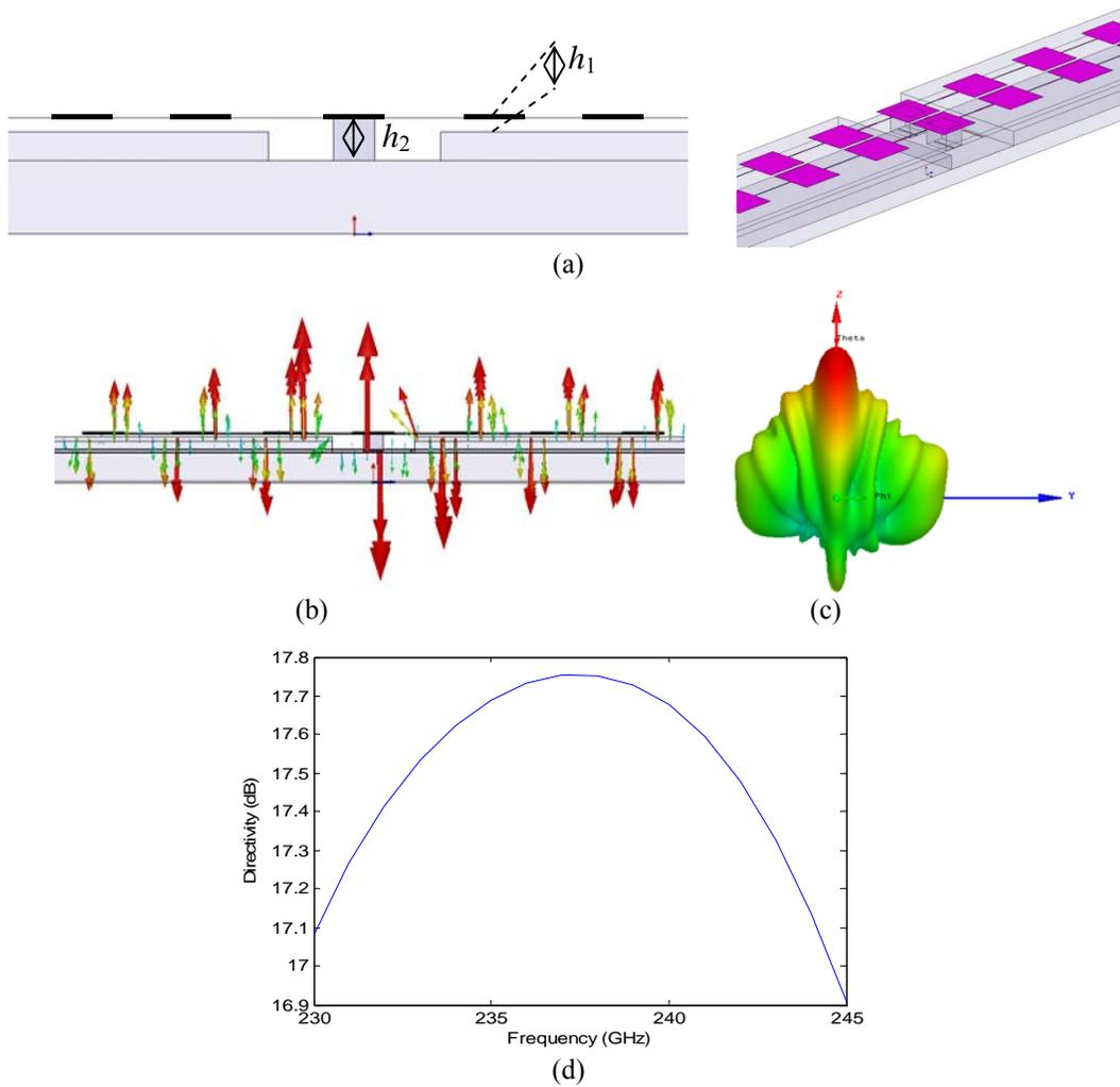
Figure 5.14. (a) The proposed hybrid-coupled patch array with silicon block to enhance slot-patch coupling. (b) The electric field distribution (c) the radiation pattern at the center frequency 237.5 GHz and (d) the directivity over the frequency band.
