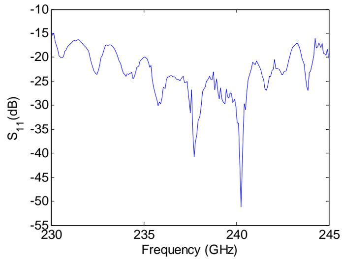
Figure 8.14. The reflection loss of the waveguide slot array.
