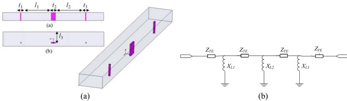
Figure 6.19. (a) The structure of E-plane two-pole filter. (b) The equivalent circuit model.
