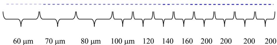
Figure 5.22. The slot width for each four/two turns so that eight different widths are used for the 28 turn waveguide. The length of the slots is  $400 \mu\text{m}$ .
