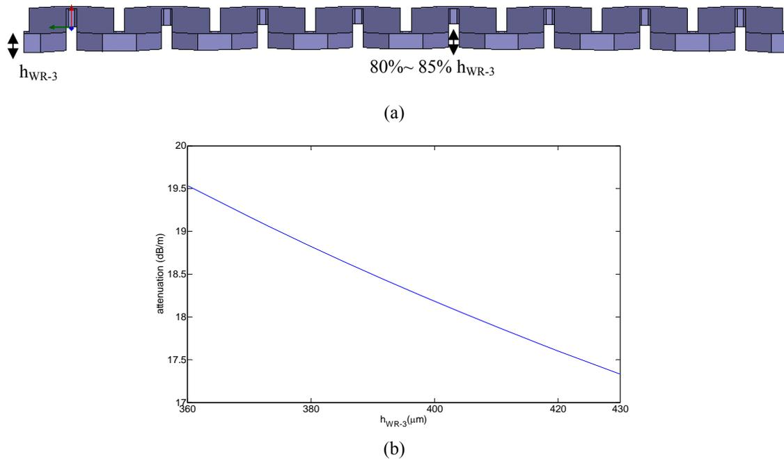
Figure 5.18. (a) Non-uniformity in the etched surfaces caused by DRIE. (b) Waveguide loss versus height. It is shown that by decreasing the height, loss increases.
