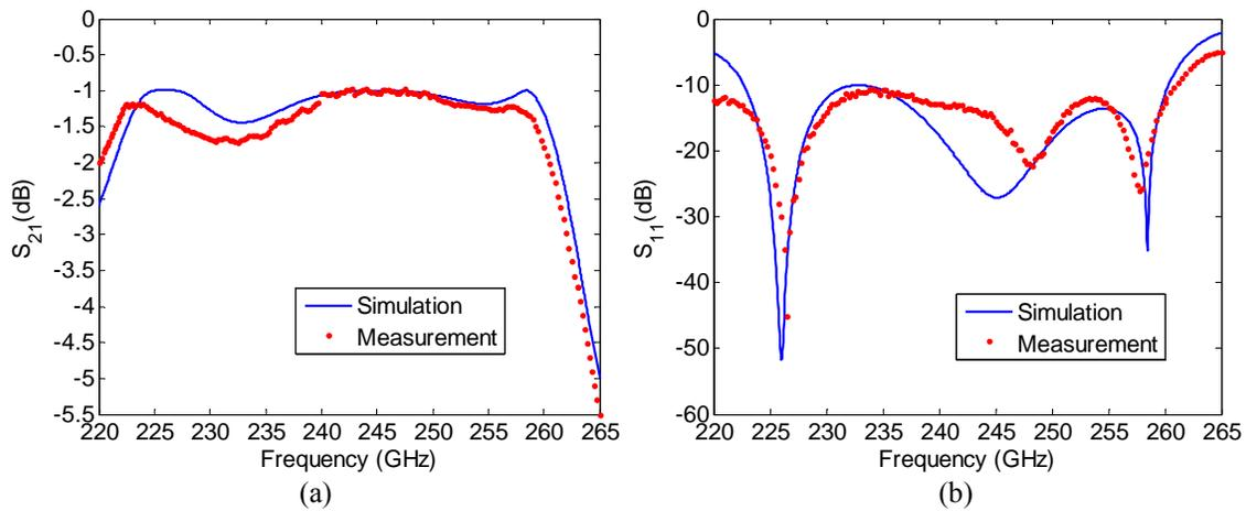
Figure 8.3. The measured transmission and reflection coefficients of the back-to-back transition structure of Figure 6.4. The results are in good agreement with the simulation. The transmission coefficient is below -1.5 dB for the two series transitions and the waveguide section in between.
