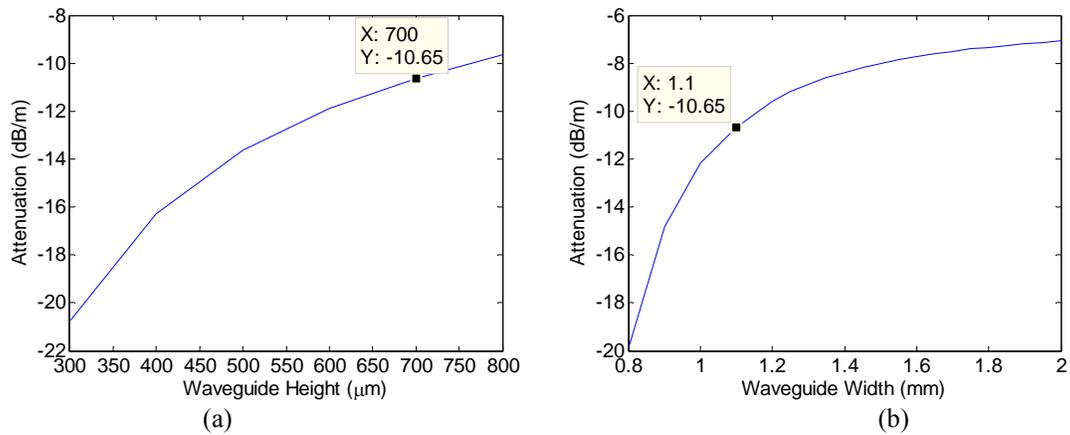
Figure 5.20. Waveguide loss (a) versus waveguide height for width =  $1100 \mu\text{m}$  (b) versus waveguide width for height =  $700 \mu\text{m}$
