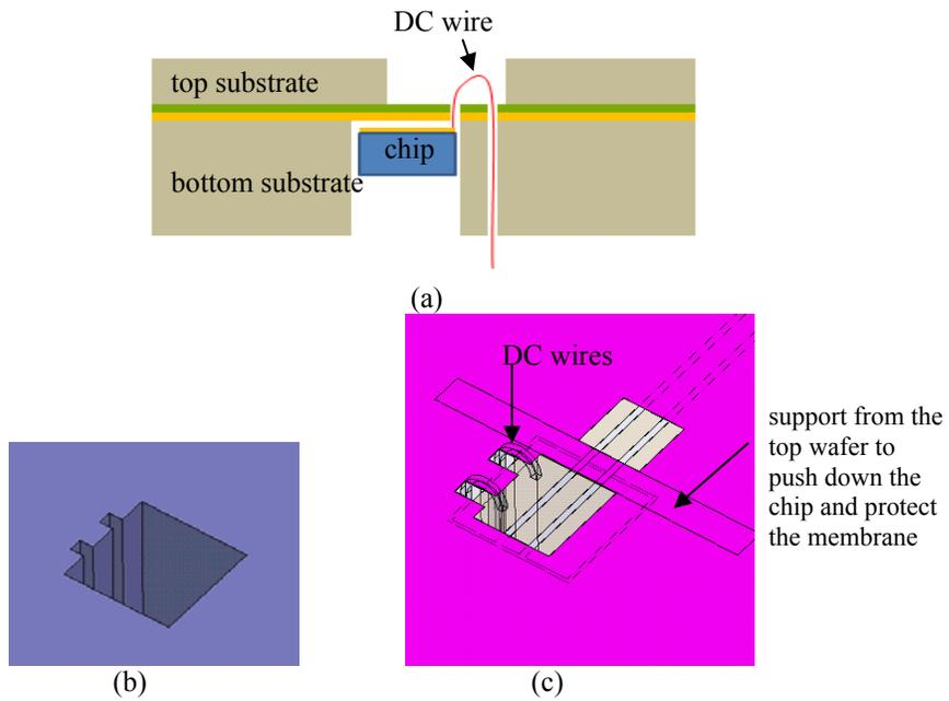
Figure 6.15. (a) Schematic of the thru-wafer transition for chip packaging. (b) a hole is etched on the bottom wafer for the chip and for the DC line transfer. (c) The structure of the packaging after bonding and embedding the external chip.
