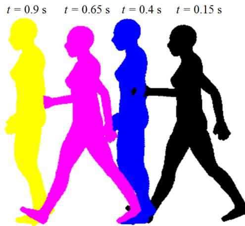
Figure 3.11. The position of human body during walking at different time frames (approaching the radar). It is observable that around  $t = 0.15$  s and  $t = 0.65$  s where the legs and arms are spread out, the RCS of legs and arms are lower as shown by Figure 3.10. Similarly, around  $t = 0.4$  s and  $t = 0.9$  s when the legs and arms are aligned with the body, the response is higher.
