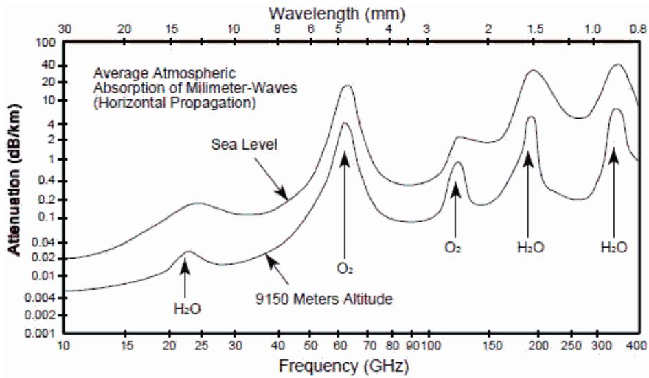
Figure 1. 1. Atmospheric absorption of millimeter wave [2]. Principal windows exist at 35, 94, 140 and 220 GHz with extremely large available bandwidths around each.
