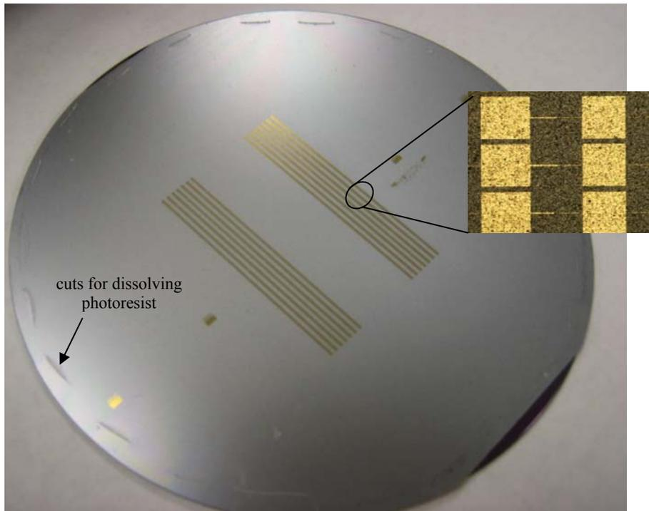
Figure 7.14. Fabricated third wafer after dissolving the photoresist release layer.
