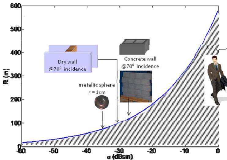
Figure 4.3. Radar range versus RCS is represented for some sample targets. Target that fall under the curve are detectable
