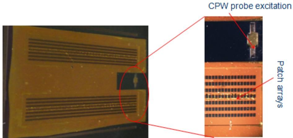
Figure 7.16. Final fabricated structure.
