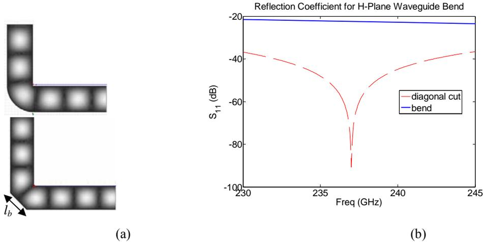
Figure 5.4. (a) Electric field distribution inside the waveguide for curved and diagonal cut bends. (b) Reflection coefficient from the bends. The diagonal cut bend is  $45^\circ$  and  $l_b = 0.85$  mm.
