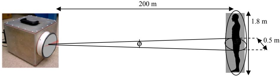
Figure 3.20. The required antenna beamwidth to provide footprints commensurate to human body width.
