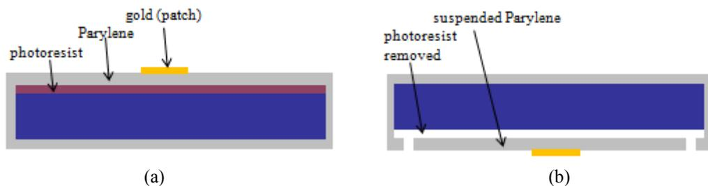
Figure 7.13. Third wafer fabrication process. (a) photoresist, Parylene and patterned gold are deposited on a silicon wafer. (b) photoresist is dissolved by soaking the wafer in acetone and IPA.
