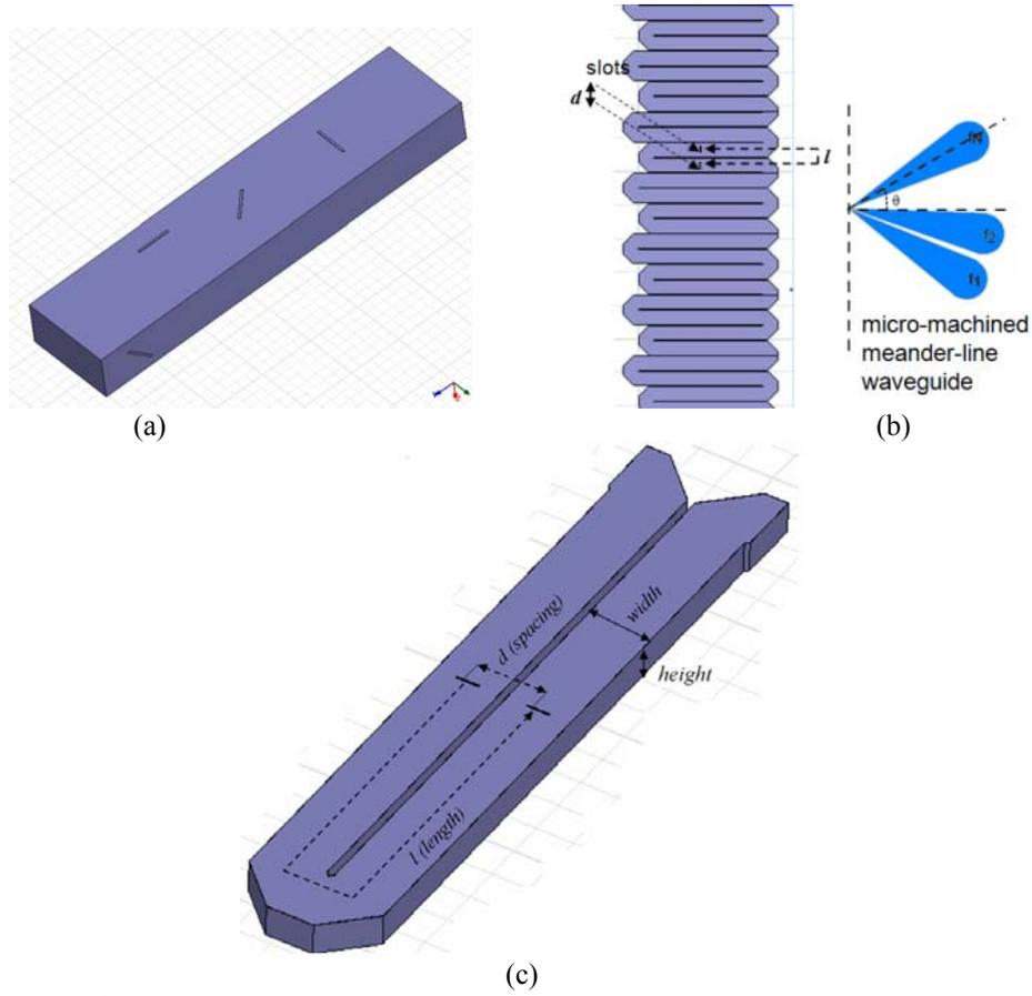
Figure 5.2. (a) Different configuration of slots cut on the walls of a rectangular waveguide. (b) Planer meander-line waveguide slot antenna (d) unit cell of the proposed structure.
