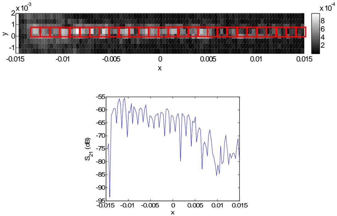
Figure 8.21. (a)  $S_{21}$  intensity measured over the slot openings of the reduced-loss design with the diffusion barrier layer. (b)  $S_{21}$  intensity over the cells shown in part (a).
