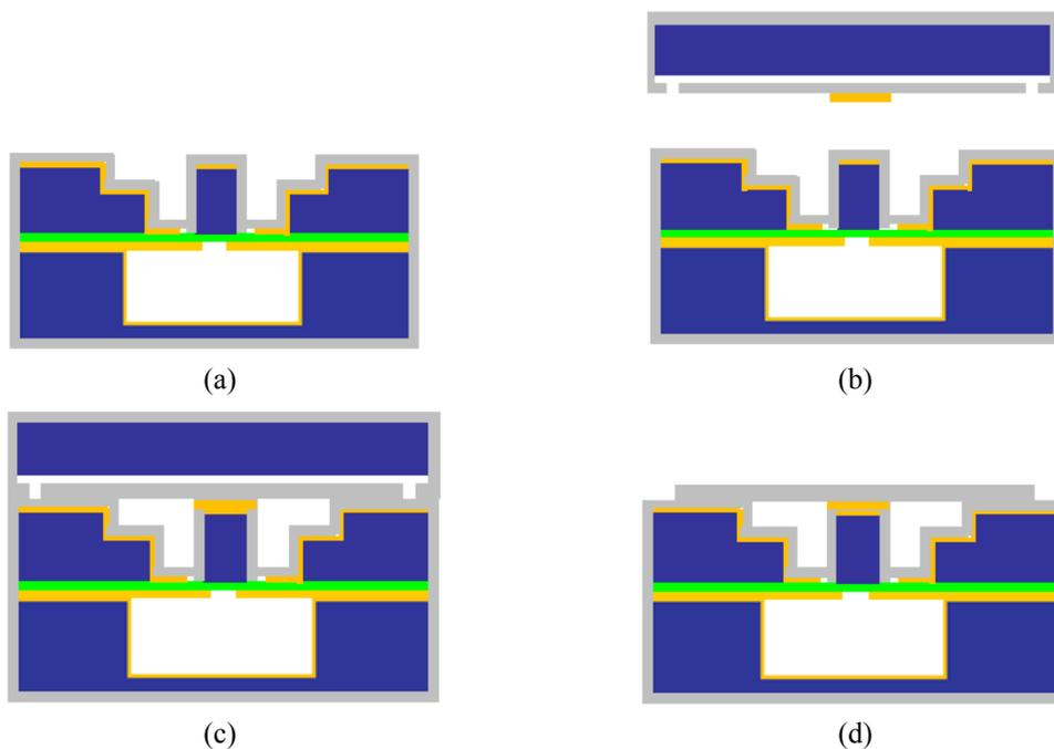
Figure 7.15. Last step of the fabrication process. (a) The gold-bonded pair is Parylene-coated. (b) The wafers are aligned and (c) bonded. (d) The third wafer is de-bonded with a razor blade through the edges.
