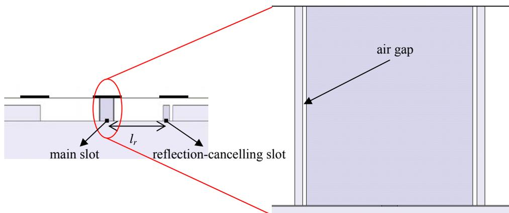
Figure 5.15. A developed version of hybrid-coupled patch array compatible with microfabrication.
