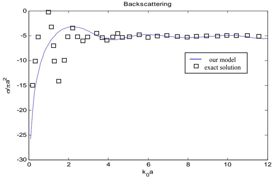
Figure 2.8. Normalized back scattering RCS of a lossy sphere with  $\epsilon_r = 5 + j10$  versus normalized frequency  $k_0 a$  compared with exact solution (Figure 3.20 in [29]). It is obvious that by increasing the normalized frequency, the PO approach tends to the exact solution.
