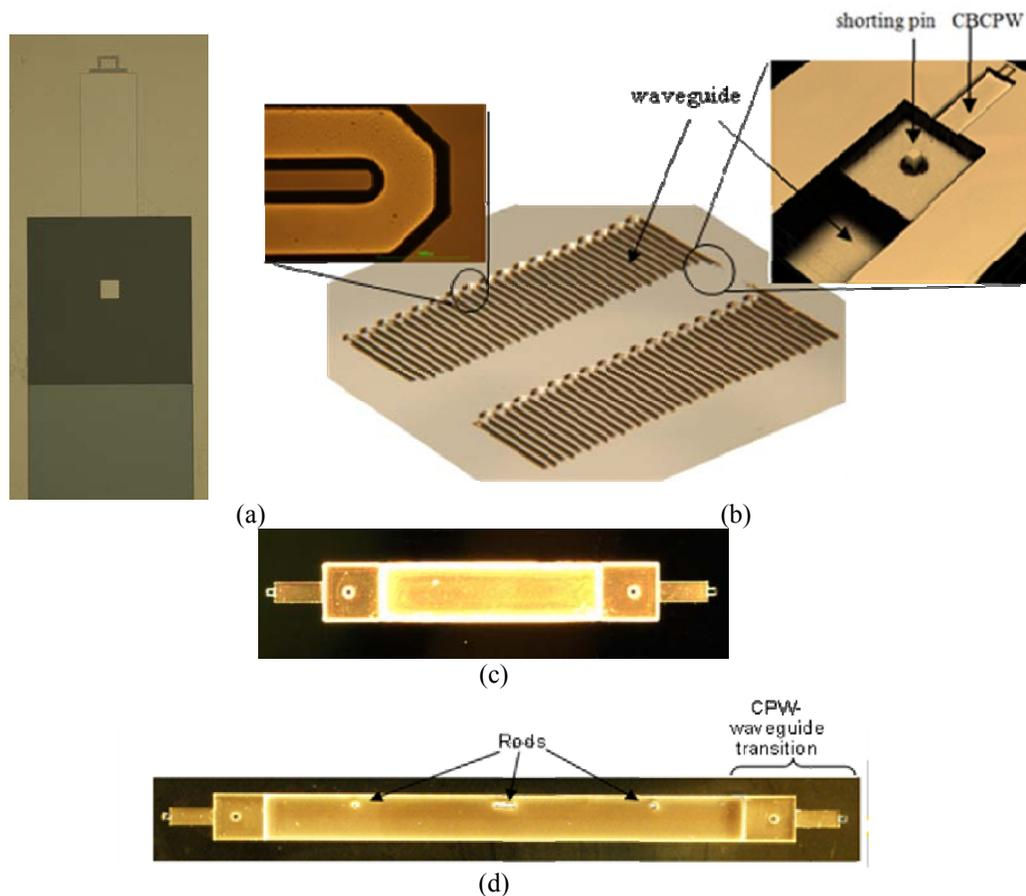
Figure 7.5. (a) Three-step patterning the waveguide. (b) Meander-line waveguide. (c) back-to-back CBCPW to waveguide transition. (d) waveguide filter with the transition
