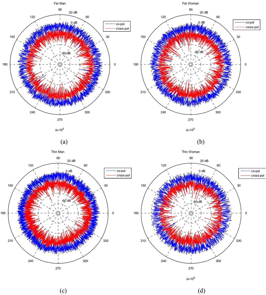
Figure 2.24. The IPO responses for (a) oversize man (b) oversize woman (c) thin man and (d) thin woman targets at  $\theta = 10^\circ$  incident angle. Different amplitude level can be observed for different sizes and genders.
