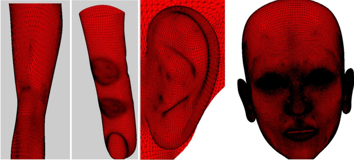
Figure 2.3. Facet distribution in the ear, thigh, finger and face. The non-uniform discretization involves the smaller parts have finer facets (fingers and ears) while larger parts have larger facets (thighs).
