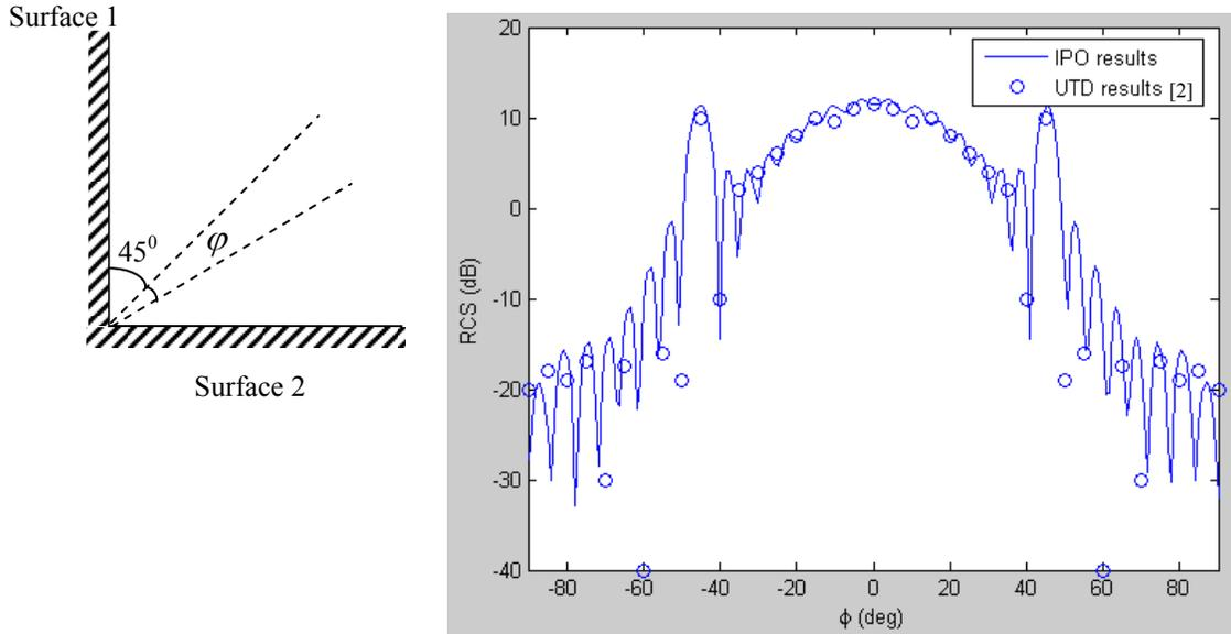
Figure 2.12. RCS of  $90^\circ$  PEC dihedral corner reflector with dimensions  $5.6988\lambda \times 5.6988\lambda$  at 9.4 GHz in [31] compared to IPO results.
