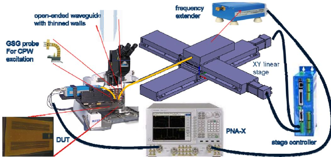
Figure 8.5. The proposed setup to measure the antenna near-field.
