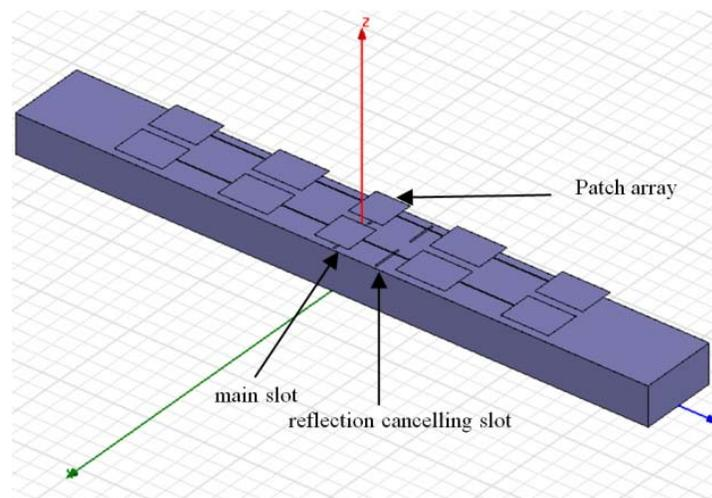
Figure 5.9. Hybrid-coupled patch array fed by the main slot
