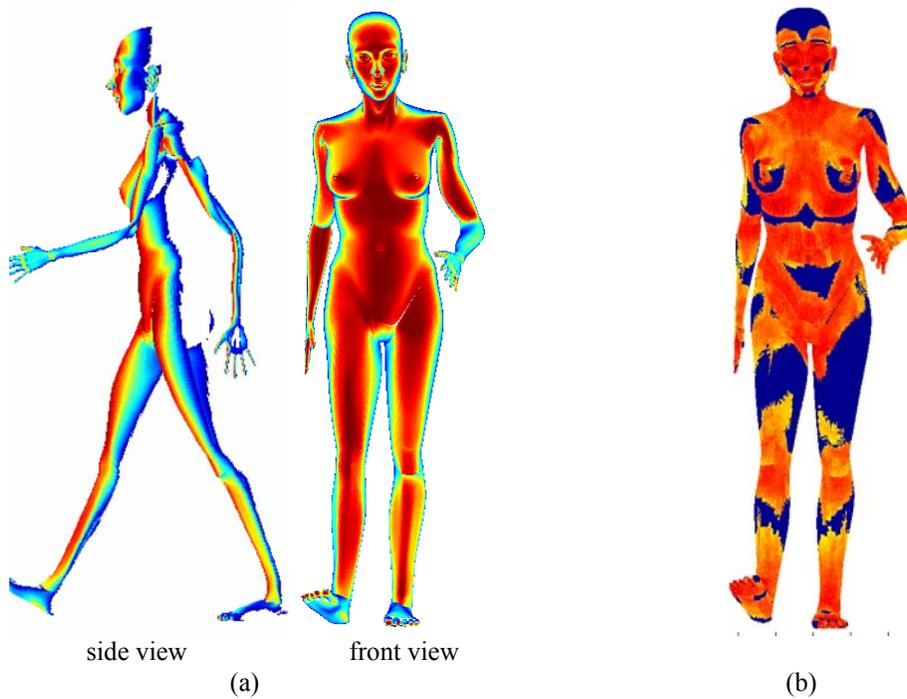
Figure 2.14. (a) First and (b) second order electric current distribution on human body when it is illuminated from the front side. The second order distribution is represented in log-scale.
