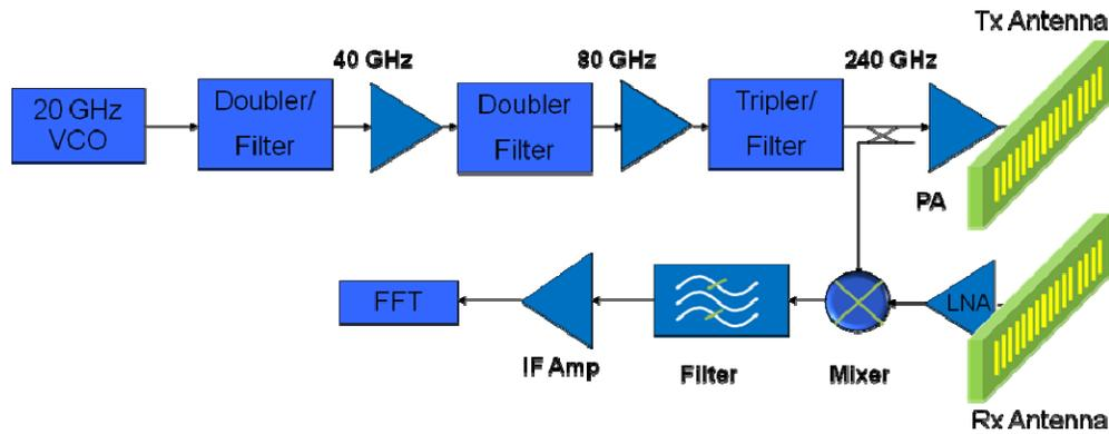
Figure 4.1. Block diagram of the Y-band FMCW radar.
