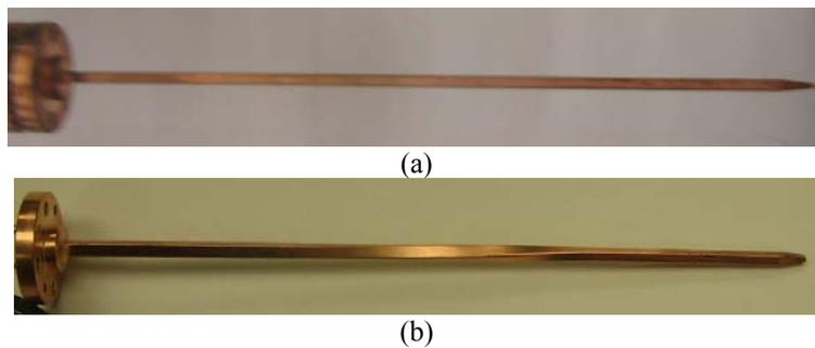
Figure 8.6. (a) Straight and (b) twisted waveguide probes to measure co- and cross-polarized field components.
