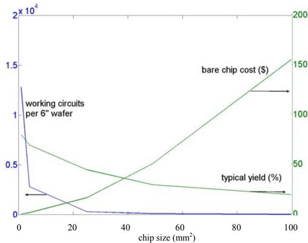
Figure 1. 4. MMIC chip sizes versus cost, yield and packing density for a high-yield MESFET process using ion-implantation. It shows as the chip size increases less chips are obtained from the wafer and hence lower yield and high cost are resulted.
