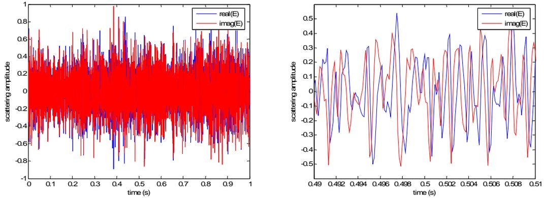
Figure 3.2 Time domain variations of scattering amplitude of the walking human body of Figure 3.1.
