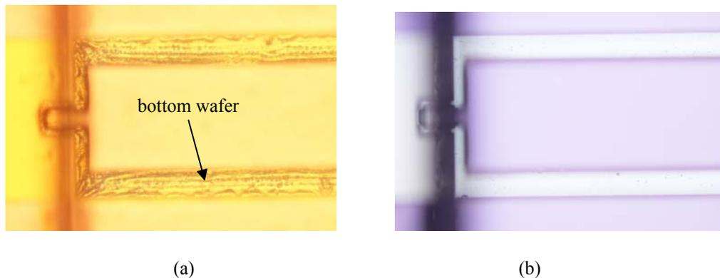
Figure 8.20. Gold quality on the bottom wafer after bonding (a) without and (b) with a diffusion barrier layer.
