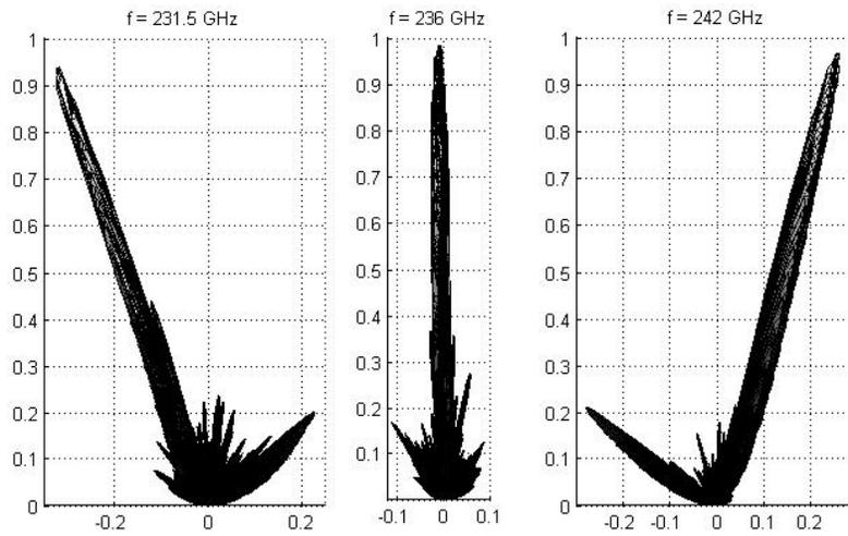
Figure 8.22. Far-field radiation pattern of the reduced-loss design with the diffusion barrier layer at different frequencies, beamwidth =  $3.5^\circ$ .
