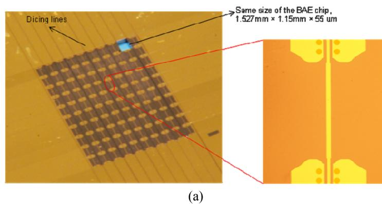
Figure 7.19. (a) the chip is fabricated on a silicon wafer with a simple CPW to microstrip transition optimized for maximum insertion.
