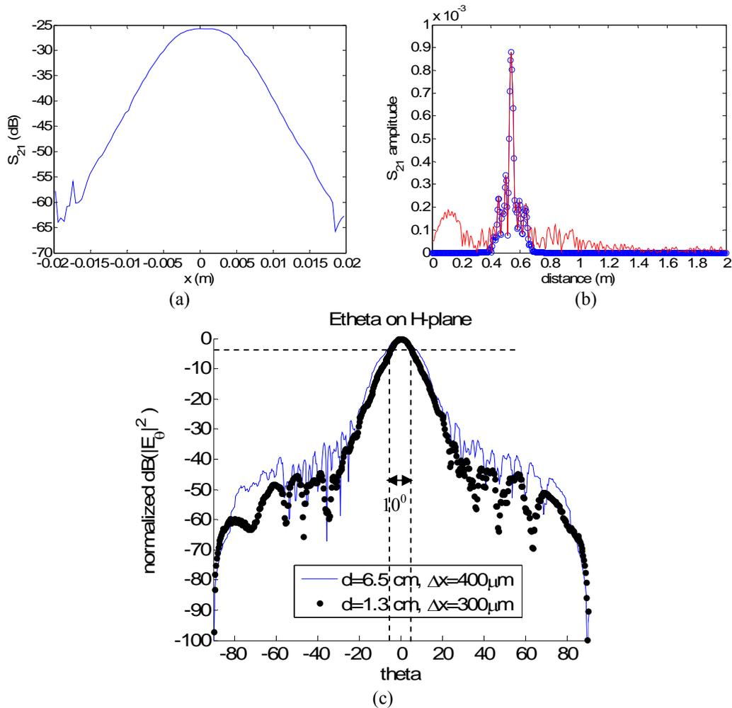
Figure 8.9. (a)  $S_{21}$  magnitude versus the scanned area at  $f = 237.5$  GHz. (b) The time-domain and the gated response with Kaiser filter for the received signal at  $x = 0$ . (c) The normalized far-field radiation pattern verifies  $10^0$  HPBW.
