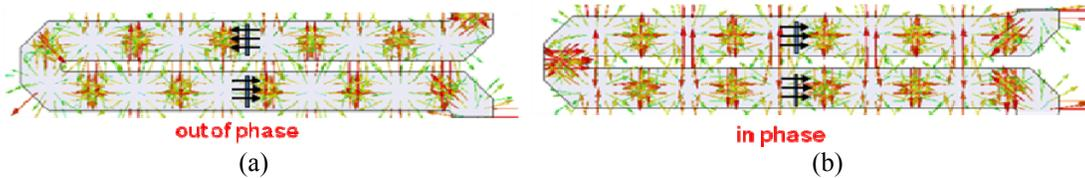
Figure 5.3. The current distribution on the broad wall of the rectangular waveguide. (a) For  $l = n \lambda_{g0}$  it is noticeable that the direction of the electric field on the slot is reversed. (b) The reverse is compensated by adding adding a  $\lambda_{g0}/2$  waveguide segment.
