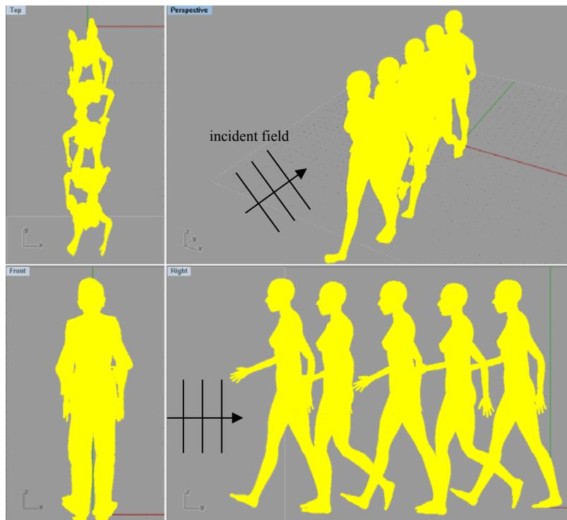
Figure 3.1. Moving human body is illuminated by a monostatic radar in the same direction as walking.
