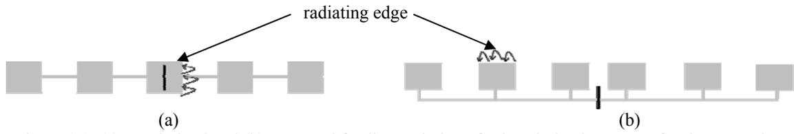
Figure 9.3. (a) v-polarized and (b) proposed feeding technique for h-polarized antennas for the same slot.
