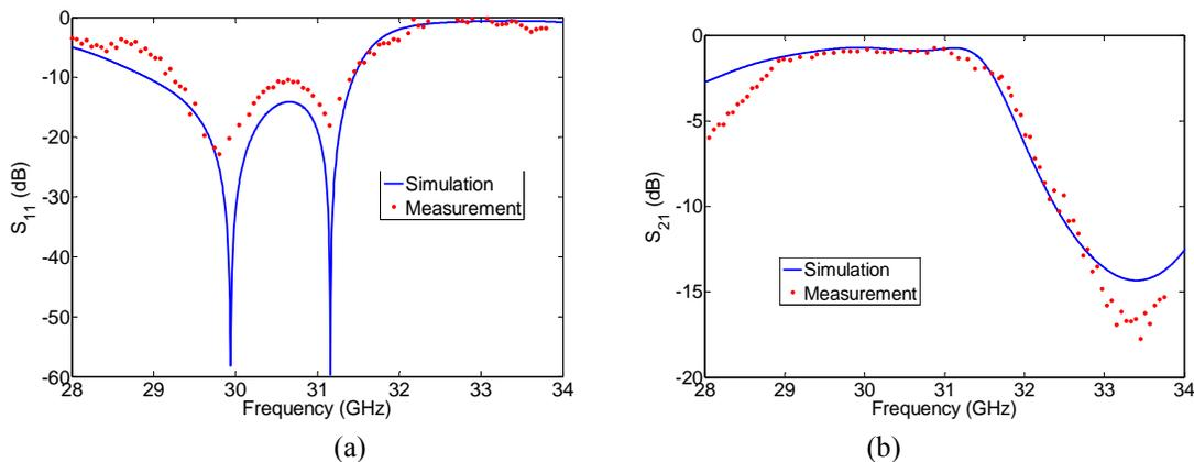
Figure 6.10. Simulation compared to measurement results for reflection and transmission coefficients which show a good agreement with the simulation. The observed deviations from the simulation are attributed to misalignment, especially near the pin positions and possible air gaps between the substrate and the brass unit
