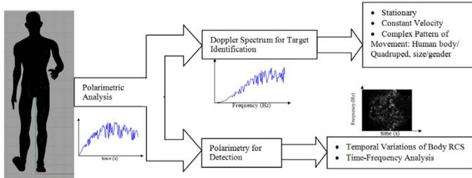
Figure 1. 6. Procedures used for target discrimination and detection. The time domain polarimetric response of the walking body undergoes processes such as Fourier transform and time-frequency analysis to derive a means for identifying human body and detecting concealed objects.
