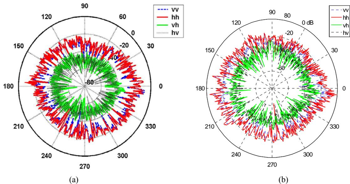
Figure 3.18. Polarimetric response of torso is measured using a 95 GHz radar (a) without and (b) with a handgun. It is observable that the presence of the firearm increases the cross-polarized response
