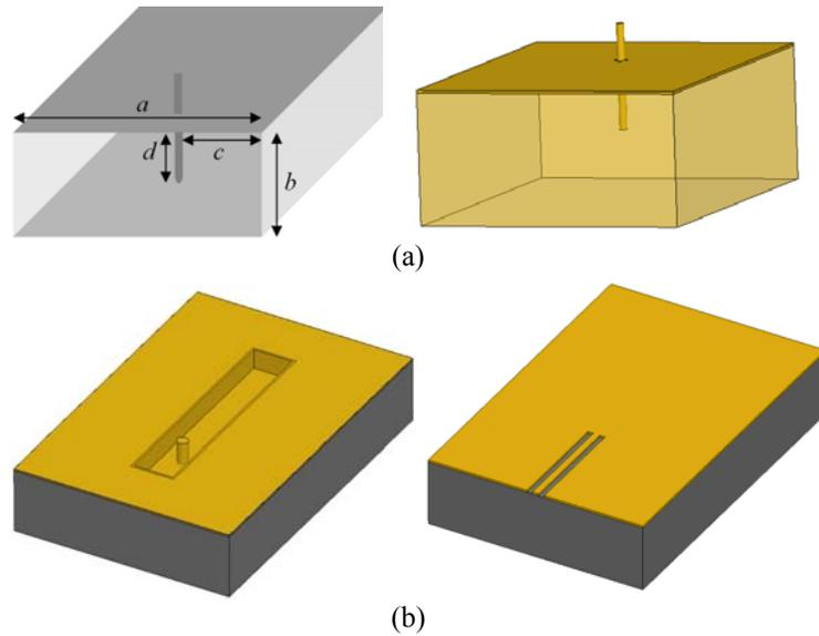
Figure 6.2. (a) Suspended E-plane probe excitation. (b) Microfabrication of short-circuited probe for in-plane CPW is performed on two wafers: one for waveguide trench and the probe, the other for CPW line. The two wafers are bonded to form the transition.
