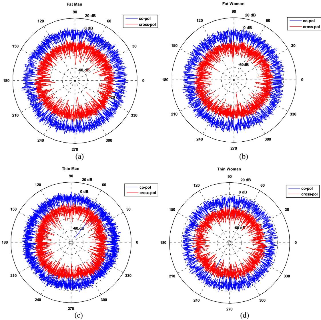
Figure 2.22. The IPO responses for (a) oversize man (b) oversize woman (c) thin man and (d) thin woman targets at  $\theta = 0^\circ$  incident angle. Different amplitude level can be observed for different sizes and genders
