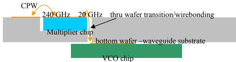
Figure 6.14. The proposed configuration for integration of the multiplier and VCO
