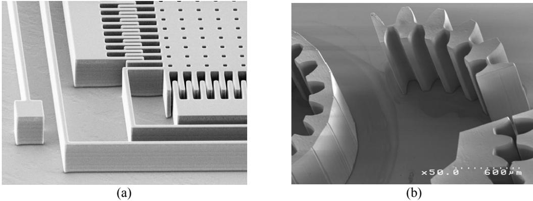
Figure 4.4. (a) Bulk micromachining: the microstructure is fabricated by DRIE etching of silicon substrate [61]. (b) Surface micromachining: the microstructure is fabricated using lithography of a thick SU-8 photoresist layer [62].
