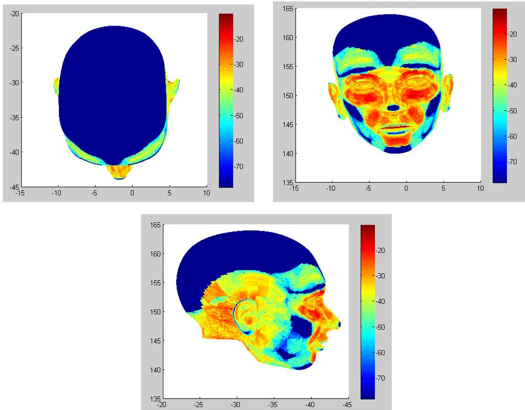
Figure 2.16. Second order electric current distribution in log-scale. It is observable that current is zero in convex areas like head, and is concentrated in irregular areas like around nose, eyes, ears, and upper chin. Convex areas in face like cheeks, chin, forehead and eyebrows have also zero induced currents.
