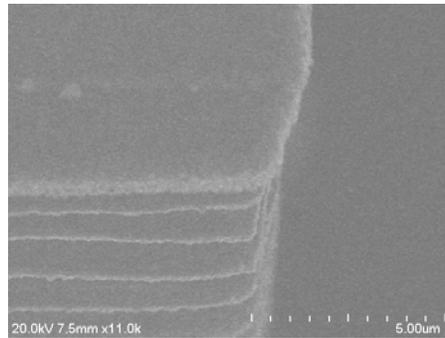
Figure 4.5. Sidewall scalloping of DRIE process
