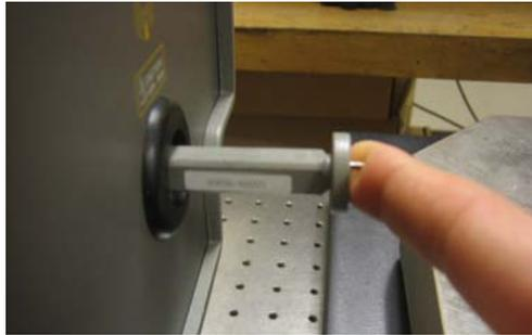
Figure 2.1. The setup for in-vivo measurement of the skin dielectric constant.
