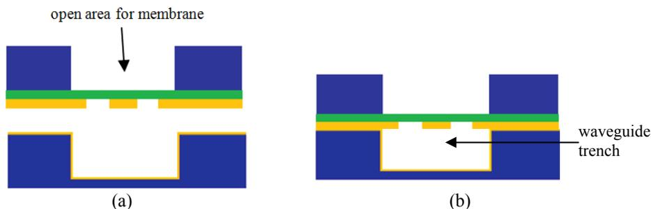
Figure 7.8. First and second wafers. (a) before gold-gold thermocompression bonding (b) after bonding
