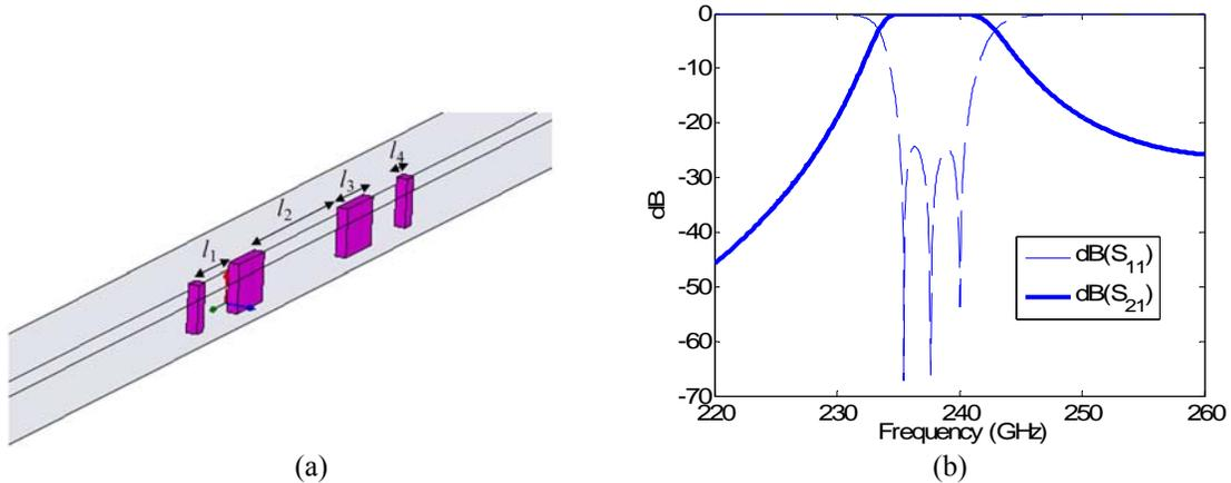
Figure 6.21. (a) The structure of the three-pole filter. (b) The response of the filter for with  $t_1=117 \mu\text{m}$ ,  $l_1=636 \mu\text{m}$ ,  $t_2=466 \mu\text{m}$ ,  $l_2=1.562 \text{ mm}$ ,  $t_3=t_1$ ,  $t_4=t_2$ ,  $l_3=l_1$ ,  $l_4=l_2$
