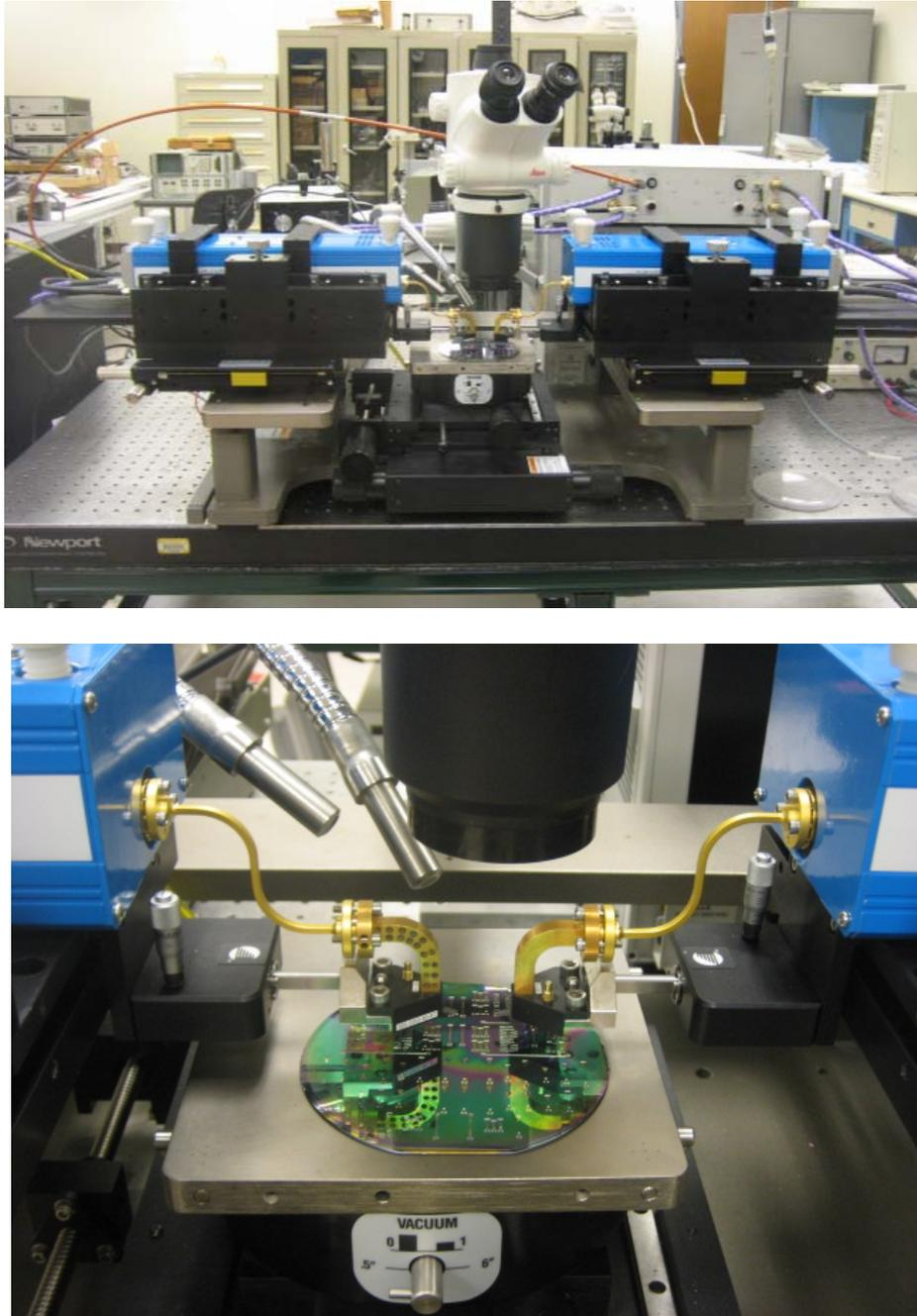
Figure 8.1. WR-3 (220-325 GHz) measurement setup.
