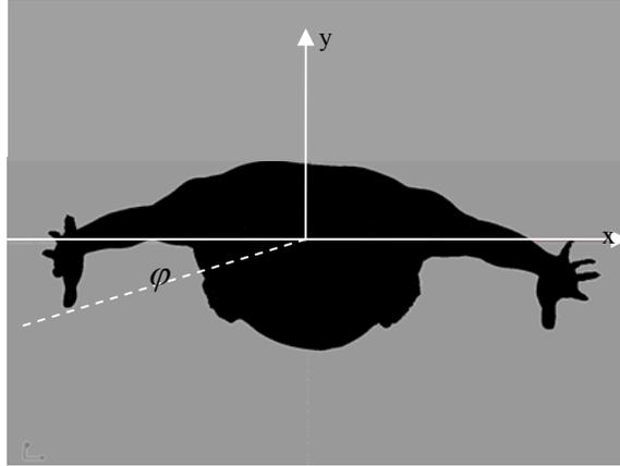
Figure 2.13. Human body is illuminated in different orientation. For each orientation the scattered field and radar cross section are calculated.
