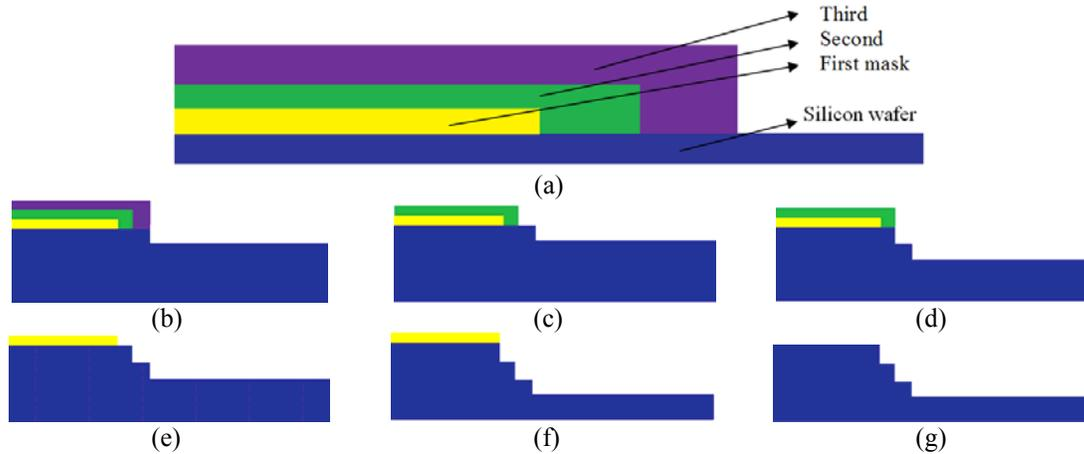
Figure 7.2. Multi-step etching process for the First wafer. (a) Three different mask layers are deposited and patterned. (b) The wafer is etched with the last mask layer down to the desired thickness. (c) The mask layer is removed. (d) The wafer is etched with the next mask layer. (e) The mask layer is removed. (f) The wafer is etched with the final mask layer. (g) The mask layer is removed. The process can be carried on for more number of steps as long as the appropriate mask layer is chosen.
