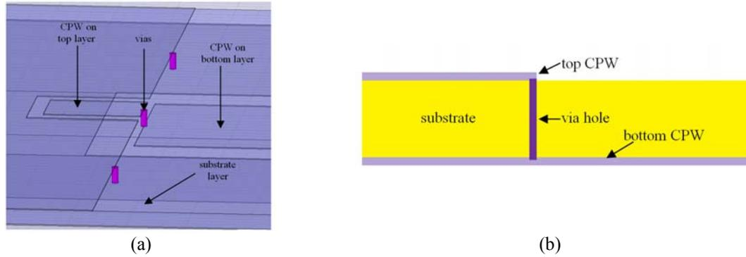
Figure 6.8. A transition from a 50 ohm CPW line patterned on top of the substrate to the CBCPW line patterned on the bottom layer. The lines are connected through electroplated via holes. (b) side view.
