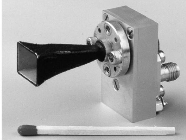
Figure 1. 5. 94-GHz FMCW radar using a horn antenna and microstrip hexaferrite circulator [15].
