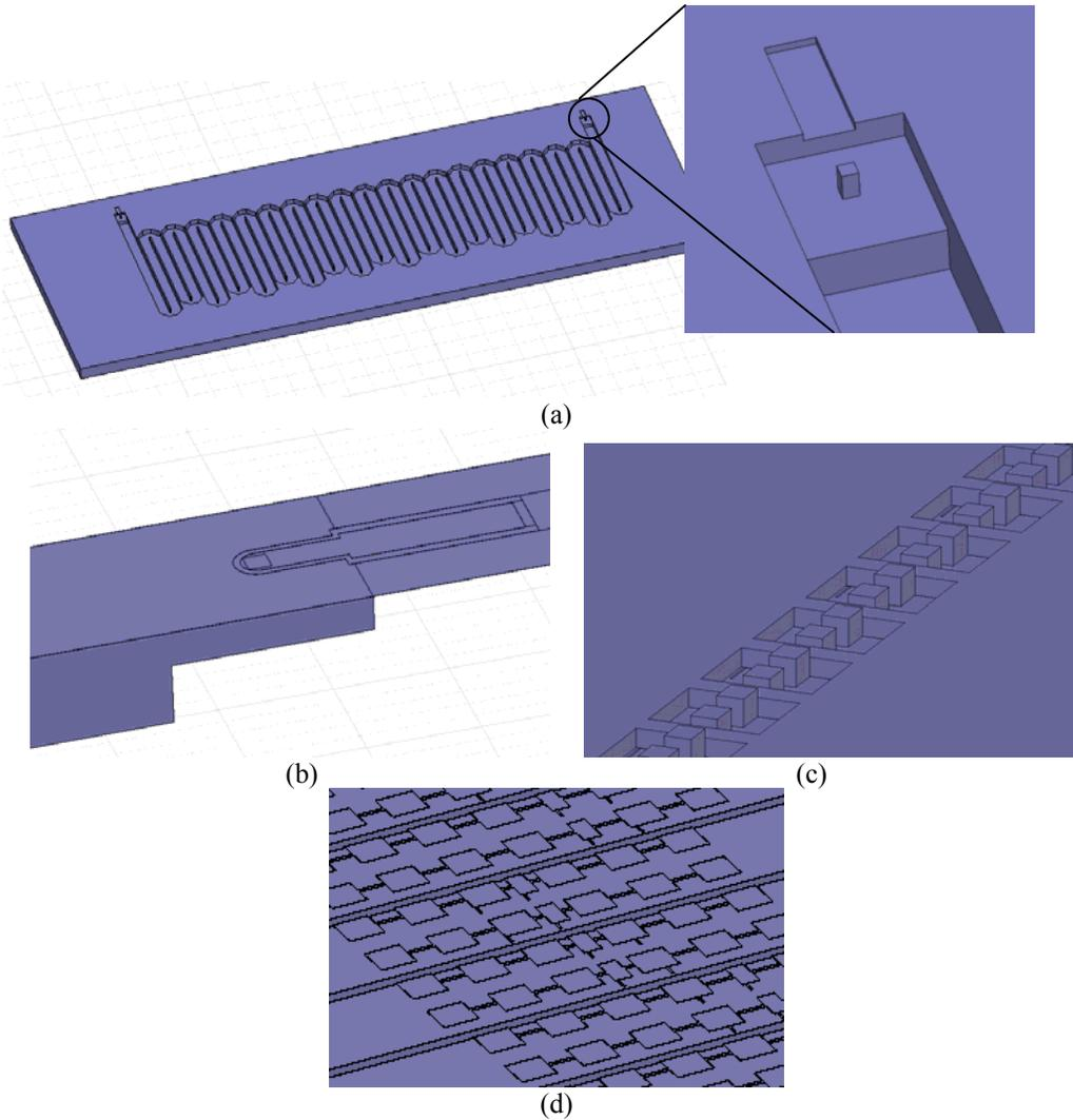
Figure 7.1. The radar structure fabrication steps. (a) First wafer includes waveguide trench and multi-step structure of the waveguide transition (b) Second wafer includes slots and CPW line patterns with the patch substrate on the other side (c) Third wafer includes the patch arrays. The wafers are connected using wafer bonding processes.
