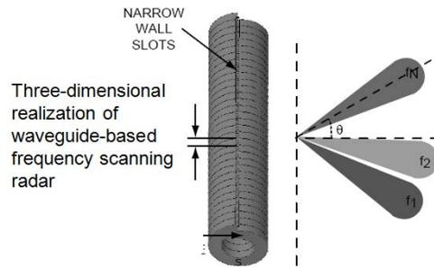
Figure 1. 8. Waveguide-based helical slot antenna.
