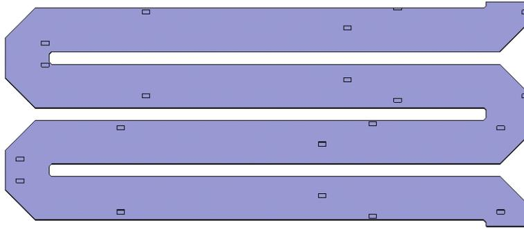
Figure 5.19. Two cells of the antenna structure are simulated with randomly-distributed defects with 20  $\mu\text{m}$  height and 50  $\mu\text{m} \times 100 \mu\text{m}$  area (corresponding to the largest bump experimentally measured)
