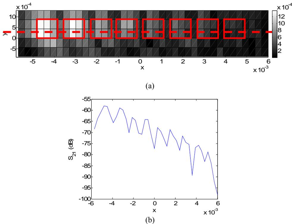
Figure 8.16. (a)  $S_{21}$  intensity measured over the slot openings of the reduced-loss design. (b)  $S_{21}$  intensity over the cells shown in part (a).
