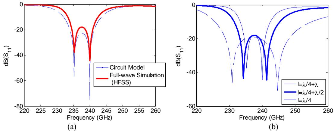
Figure 6.20. (a) The reflection coefficient of the filter presented in Figure 1 with  $t_1=75\ \mu\text{m}$ ,  $l_1=2.344\ \text{mm}$ ,  $t_2=365\ \mu\text{m}$ ,  $l_2=l_1$ ,  $t_3=638.6\ \mu\text{m}$ . (b) The response of the same filter with various values for  $l = l_2 = l_1$  maintaining  $\lambda/4$  difference.
