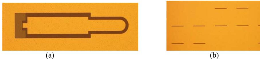
Figure 7.7. Fabricated second wafer. (a) top side- CPW/CBCPW lines (b) top side - slots
