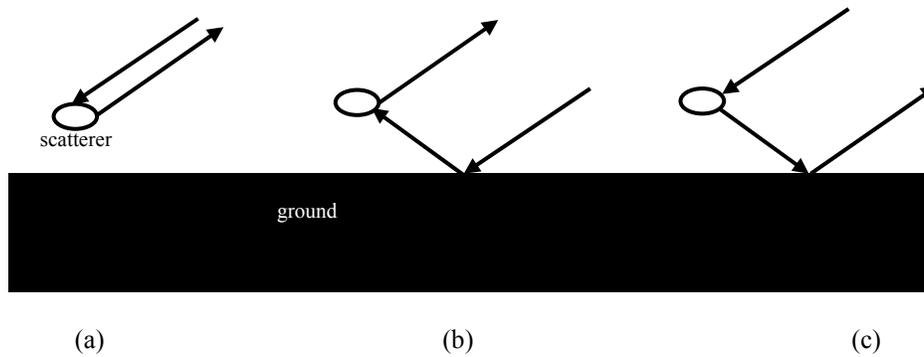
Figure 2.23. backscattering response of the target in the present of the ground plane includes: (a) the backscattering response of the target (b) the response of the target when the incident field is the reflected wave from the ground plane (c) the scattered field of the target is reflected by the ground plane and makes a backscattering response.
