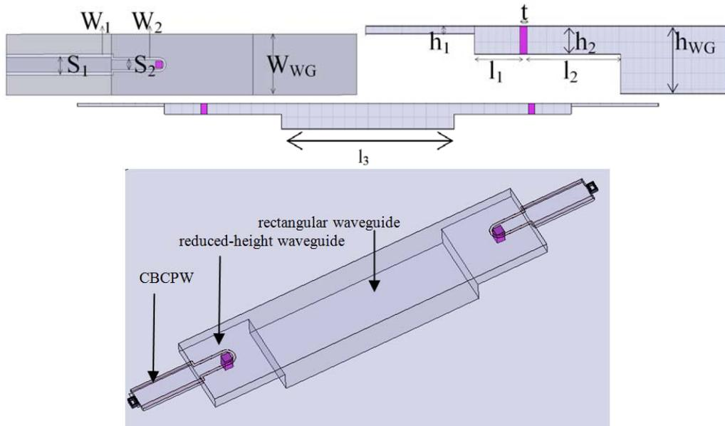
Figure 6.4. CBCPW to rectangular waveguide transition, top view, side view and the perspective of a back-to-back configuration which includes a transition from CBCPW to CPW, CPW to reduced-height waveguide and reduced-height waveguide to the standard WR-3 rectangular waveguide.
