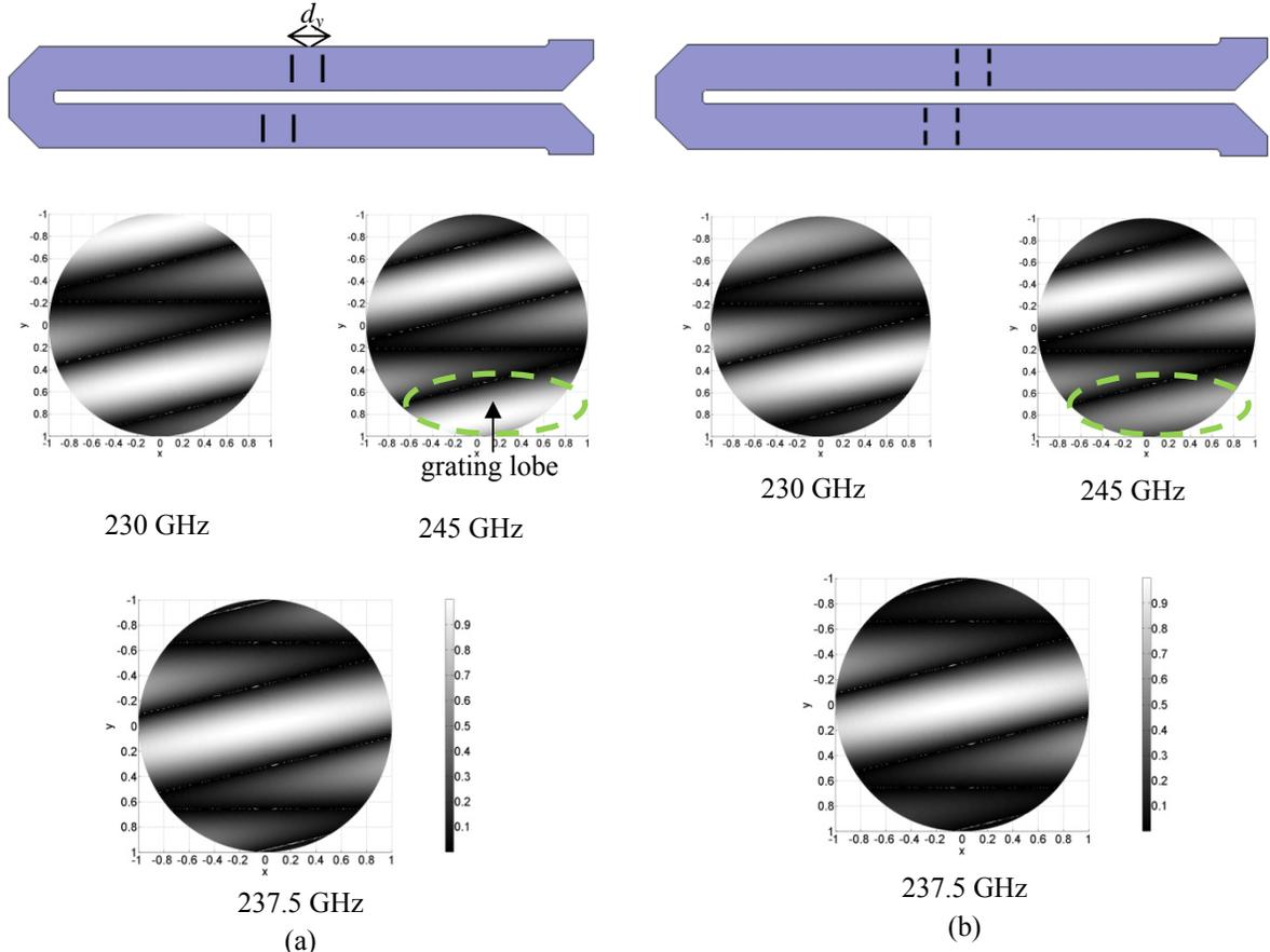
Figure 5.6. (a) Unit cell with reflection cancelling slot and the analytical far-field pattern of the array at the beginning, center and end of the band. (b). The final proposed structure with additional slot across the broad wall of the waveguide and the analytical far-field pattern of the array at the beginning, center and end of the band. It is observable that the grating lobe is around -8 dB lower.
