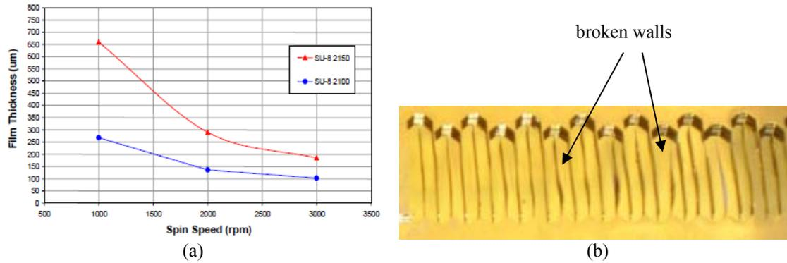
Figure 4.7. (a) Thickness versus spin speed of SU-8 series 2100. (b) meander-line structure fabricated by spinning SU-8 2100 in two steps. The structure is gold-sputtered after developing and hard-bake.
