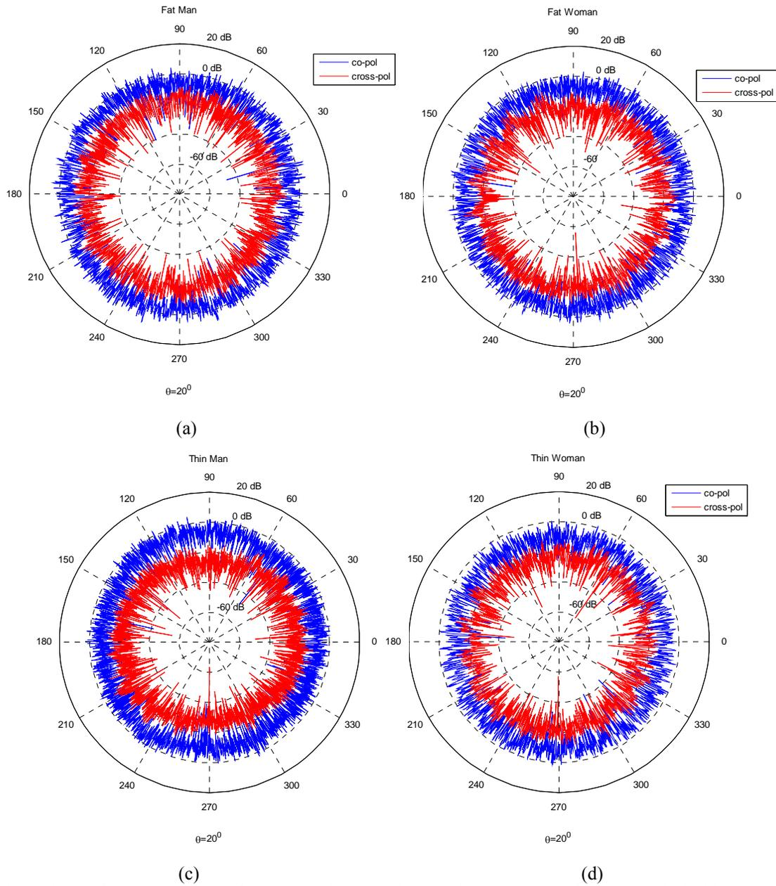
Figure 2.25. The IPO responses for (a) oversize man (b) oversize woman (c) thin man and (d) thin woman targets at  $\theta = 20^\circ$  incident angle. Different amplitude level can be observed for different sizes and genders
