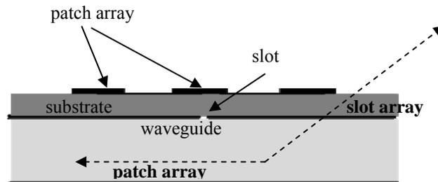
Figure 5.1. The two-dimensional structure of the antenna
