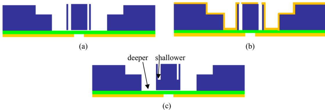
Figure 7.10. (a) multi-step etching for the patch array substrate. Thin shadow walls are also formed to protect the sidewalls of the silicon block from gold-deposition. (b) gold-coating the substrate. (c) the realistic version of the structure.
