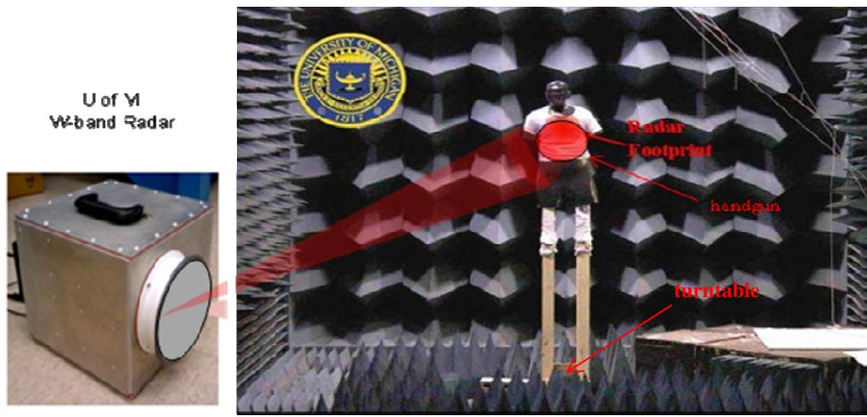
Figure 3.17. W-band RCS measurement setup for human body. It is mounted on top of a turntable.
