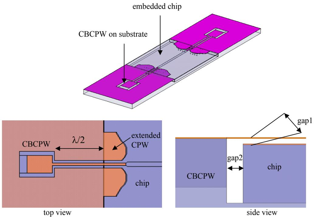
Figure 6.16. The transition between the chip and CBCPW. It includes an intermediate step of narrow transmission line with  $\lambda/2$  length
