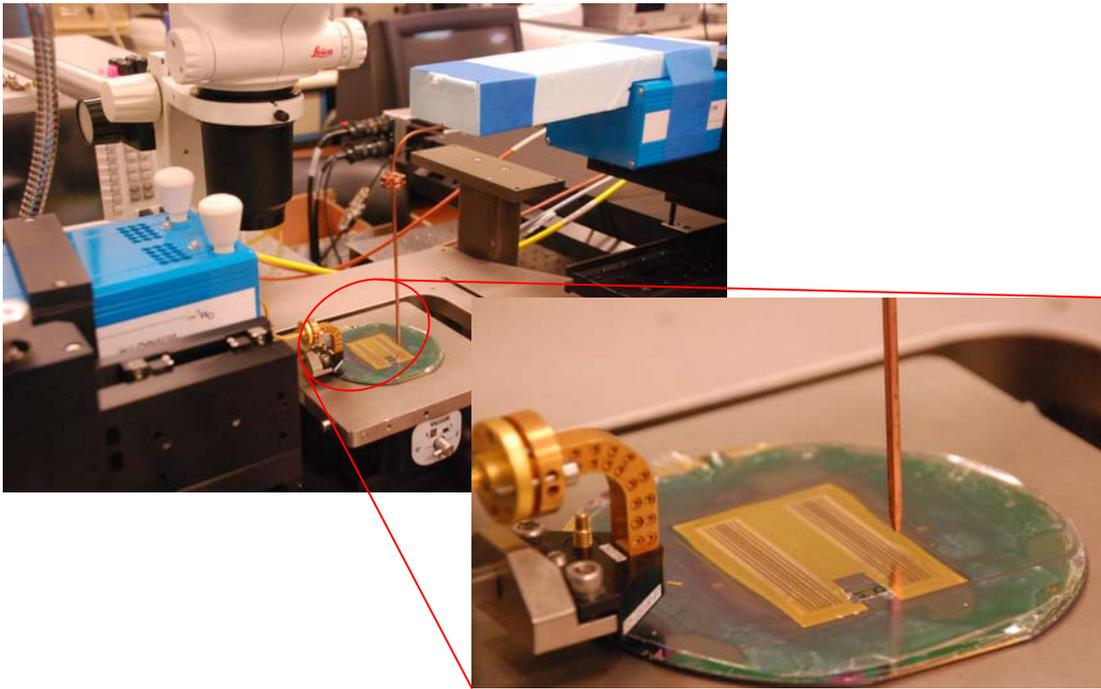
Figure 8.10. The setup proposed for the antenna measurement. The antenna is excited through the GSG probes and the radiated power is measured with a waveguide probe. The waveguide probe is connected to the frequency extender through a waveguide bend and its position is controlled by the XY stage.
