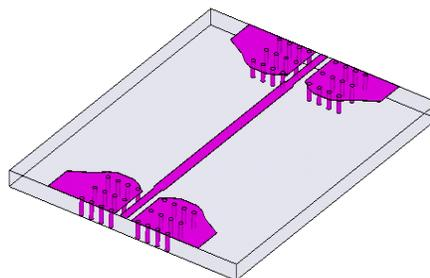
Figure 6.18. The transmission line chip designed to test the packaging.
