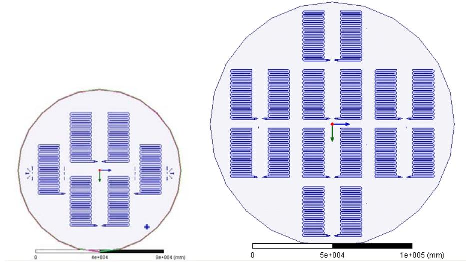
Figure 7.21. Yield of the radar structure with 4 inch and 6 inch wafers. It can be observed that while only two radars (including one transmitter and one receiver antennas) can be fabricated on a 4 inch wafer, eight radars (one pair of antennas) can be fabricated on a 6 inch wafer.
