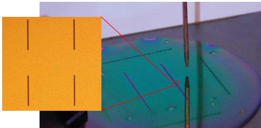
Figure 8.11. The waveguide probe moving on top of the slot openings.
