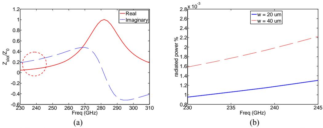
Figure 5.7. (a) Normalized slot impedance versus frequency. A resonance happened at 282 GHz. (b) The total power associated with a non-resonant slot for two different widths.
