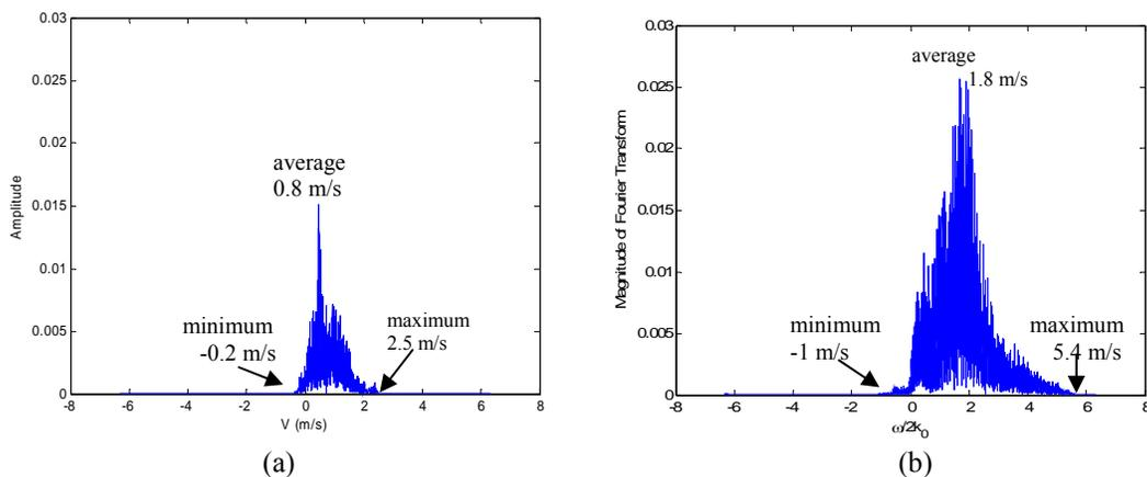
Figure 3.8. (a) Doppler spectrum of scattering amplitude of a walking dog versus velocity  $v/(2k_0)$ . It can be seen that it has peaks around its average velocity ( $v=0.8$  m/s) and the maximum and minimum velocities are 2.5 m/s and 0.2 m/s (b) Doppler Spectrum of human body presented in the previous report.
