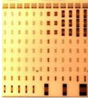
Figure 8.2. GGB CS-15 calibration substrate with line, thru, matched load, short and open.
