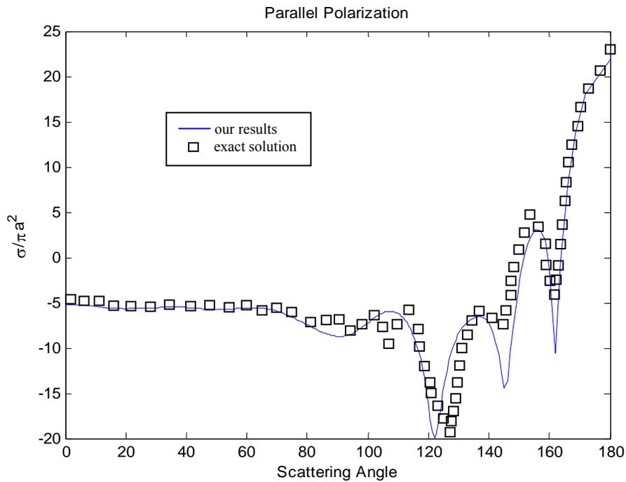
Figure 2.10. Normalized RCS of a lossy sphere with  $\epsilon_r = 5 + j10$  and  $a = 2\lambda$  for parallel polarized incident wave compared with exact solution (Figure 3.22 in [29]).
