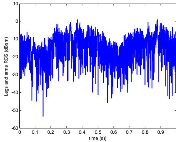
Figure 3.10. Backscattering response of the legs and arms during walking for different walking positions. It is lower when they are spread out ( $t = 0.15$  s,  $t = 0.65$  s) and higher when they are aligned with the body ( $t = 0.4$  s,  $t = 0.9$  s).
