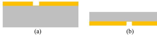
Figure 7.18. Fabrication process of a test chip (a) patterning gold on a silicon wafer (b) etching the backside of the wafer to thin down to the desired chip thickness.
