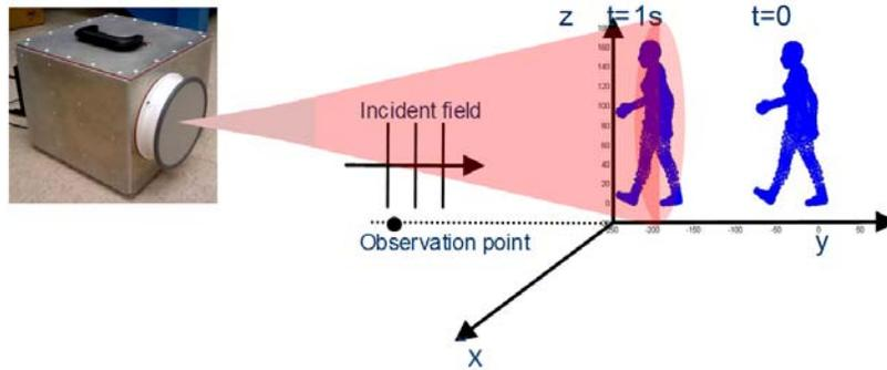
Figure 1. 7. The University of Michigan W-band polarimetric radar is used for human body RCS measurement.
