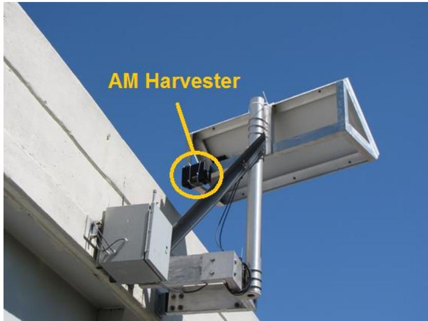
Figure 3.15. The harvester being tested on a highway bridge in Detroit, Michigan
