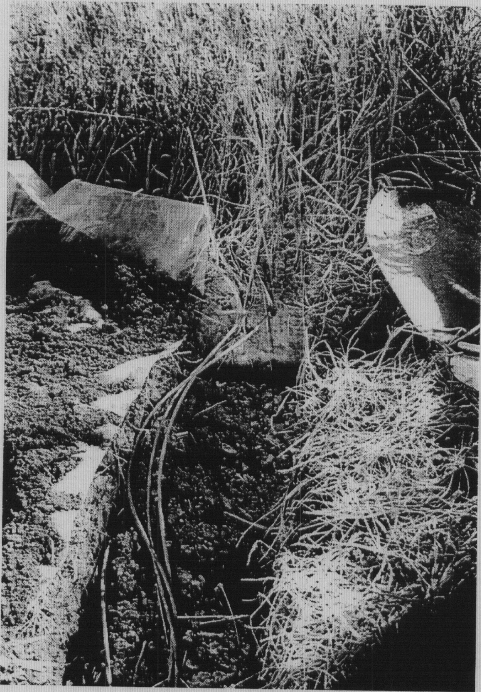
Figure 5.9: Insertion of the soil temperature probes. At the time of this picture, I had already inserted the probes in the side of the trench and refilled it, burying the 64, 32, and 16 cm probe cables. Cables leading to the 2, 4, and 8 cm deep probes protrude from the side of the trench.
