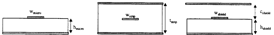
Fig. 4.3: Transmission lines used in RF input/output interconnects: microstrip, stripline, and shielded microstrip.
