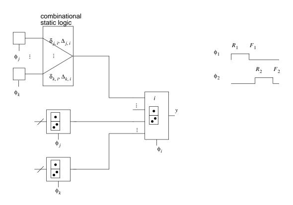
Figure 4: Timing checks for dynamic gates: circuit fragment
