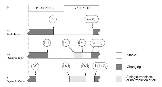
Figure 3: I/O Waveforms of a Domino gate
