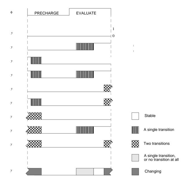
Figure 2: Waveforms of the output of a domino gate
