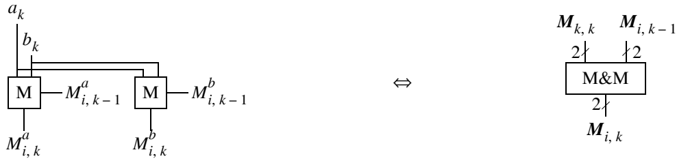
Figure 3-1: Double majority cell for computing a pair of M signals. Note that M_{k,k} = \langle a_k, b_k \rangle
