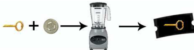
Fig. 1. The server key share and disable token are encrypted under the server’s public key to create the client ticket. The plaintext server key share is then erased.
