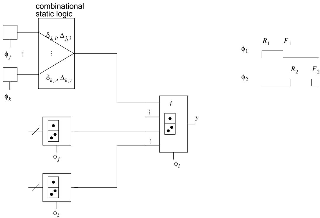
Figure 4: Timing checks for dynamic gates: circuit fragment
