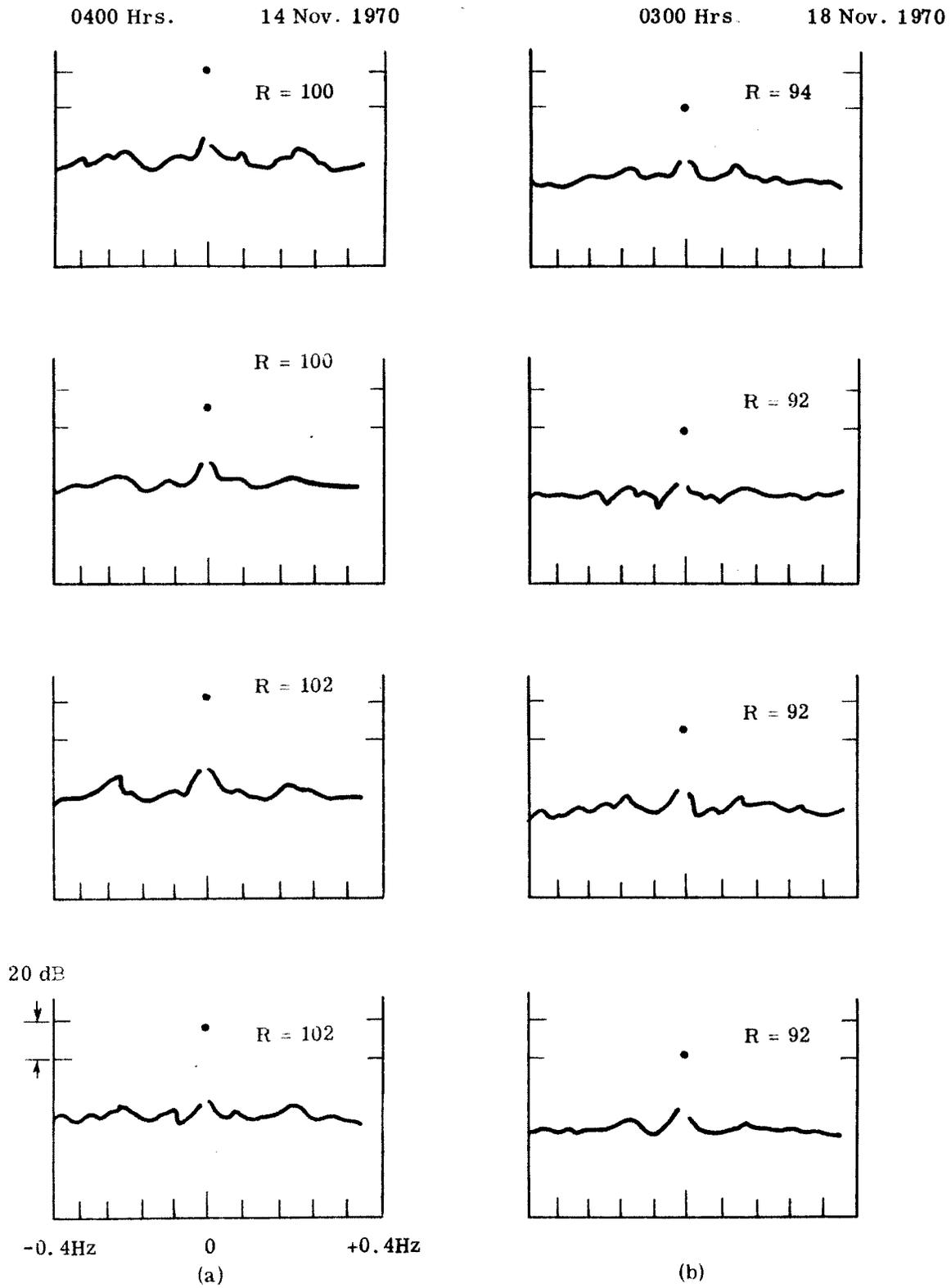
Fig. 25. Reverb spectra displays: Fowey Rocks to Bimini
