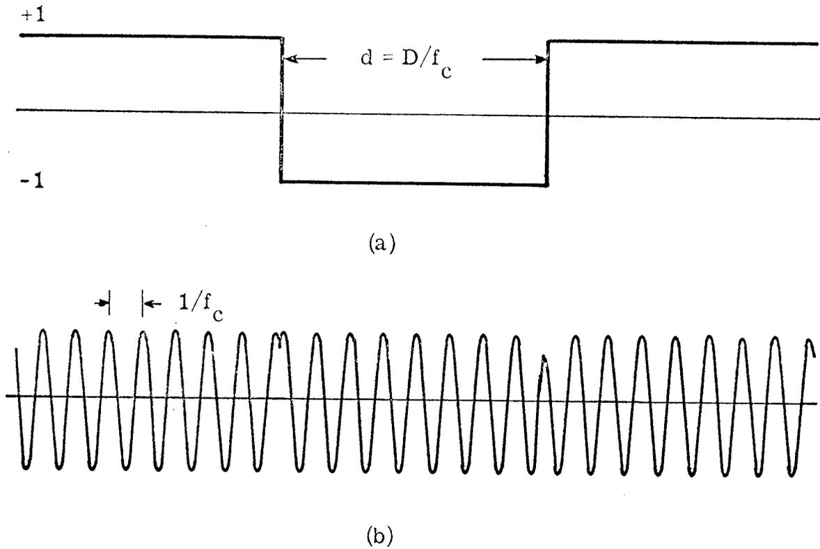
Fig. 4. A complement-phase modulated signal
