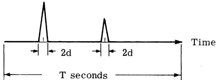
Fig. 7. A multipath display for two transmission paths
