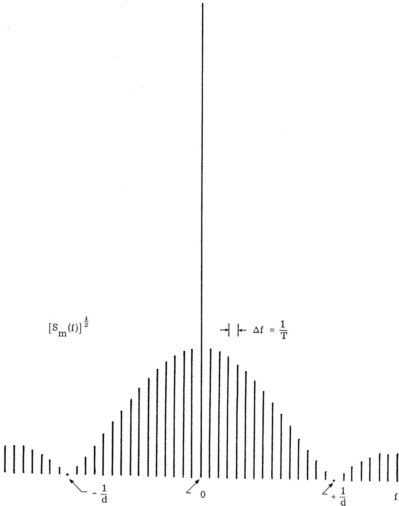
Fig. 5. The RMS spectrum of a complement-phase modulated signal for  $L = 15$  and  $D = 8$
