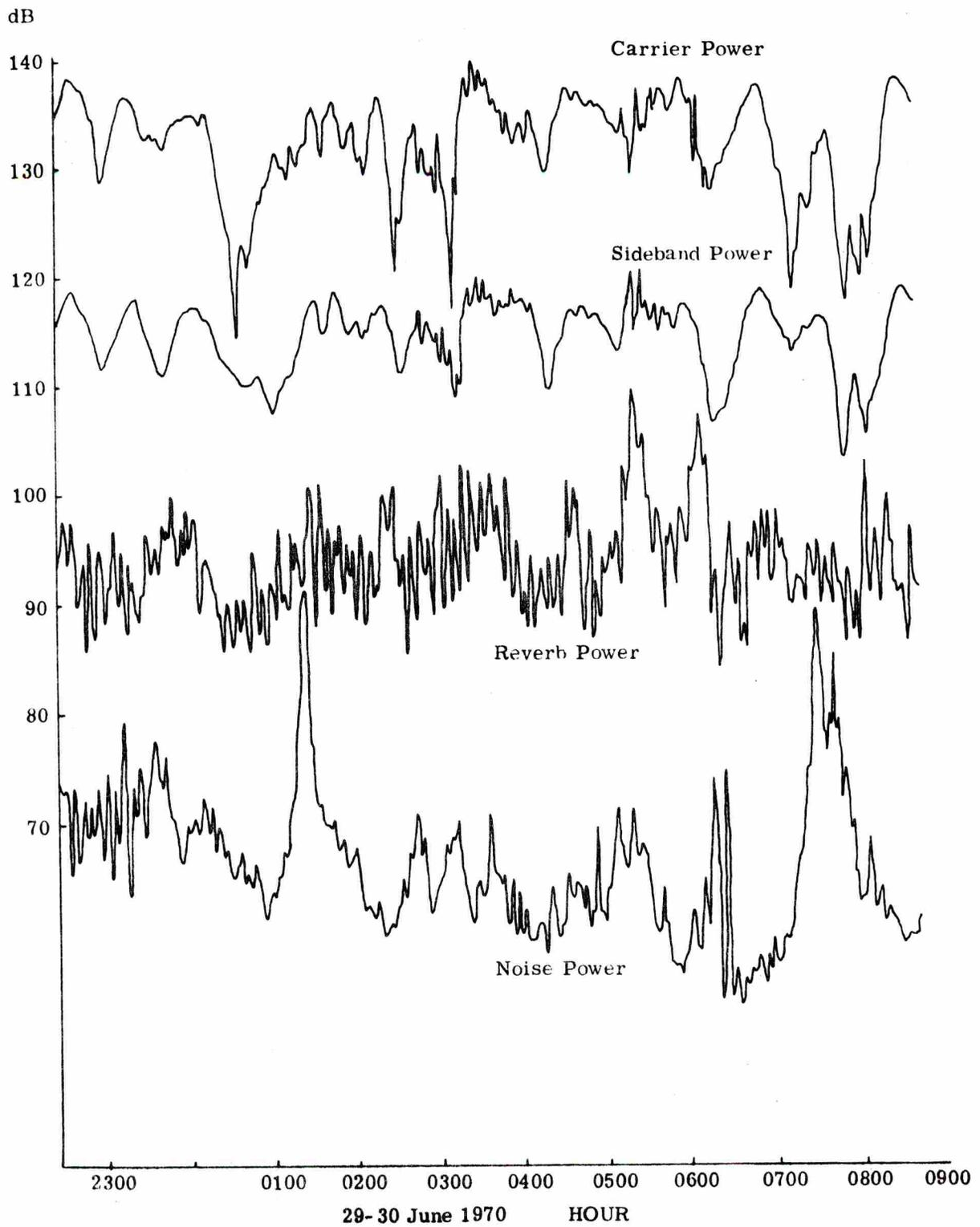
Fig. 12. Power measurements from the 7-mile hydrophone
