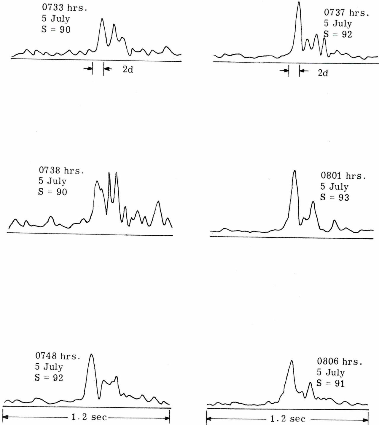
Fig. 17. Multipath displays from the Bimini hydrophone taken on 5 July 1970
