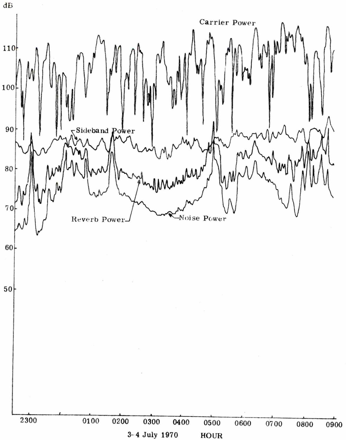
Fig. 11. Power measurements from the Bimini hydrophone
