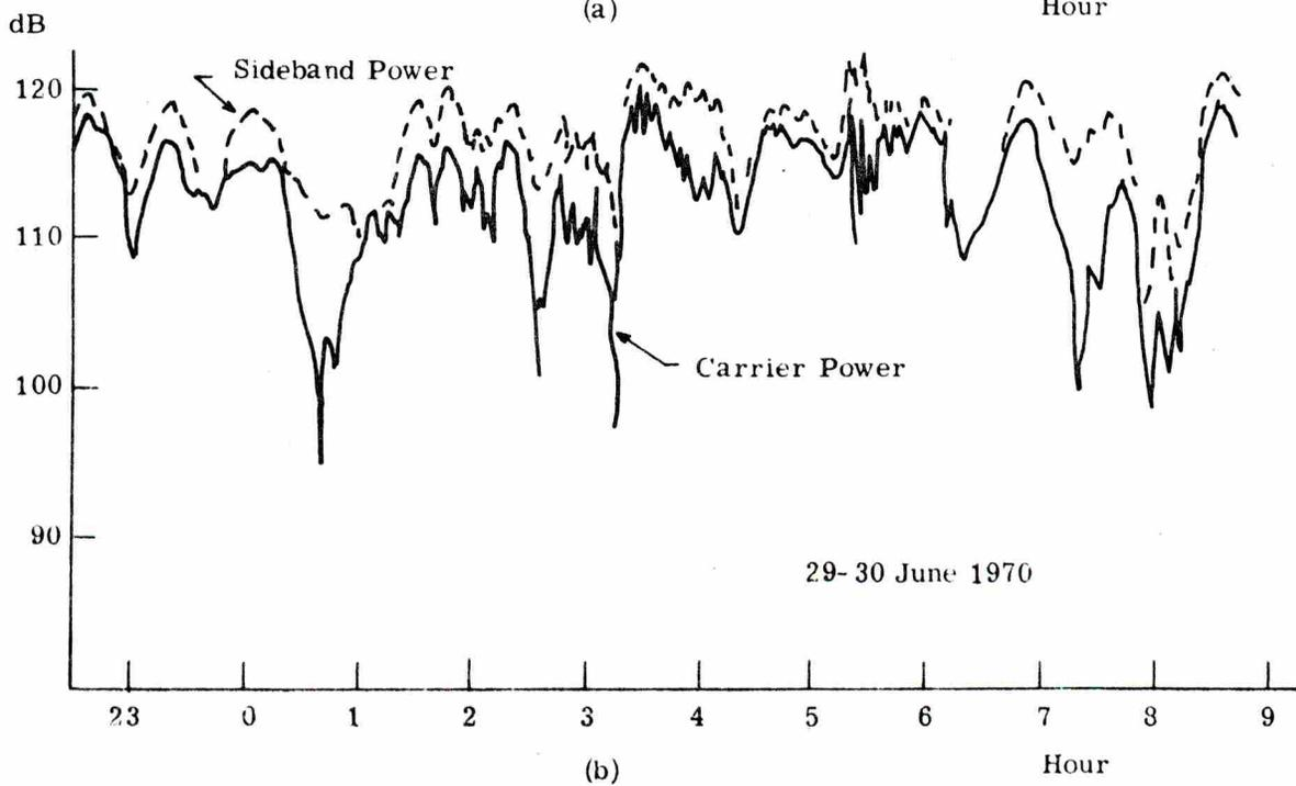
Fig. 13. Unity-gain plots of carrier power and sideband power
