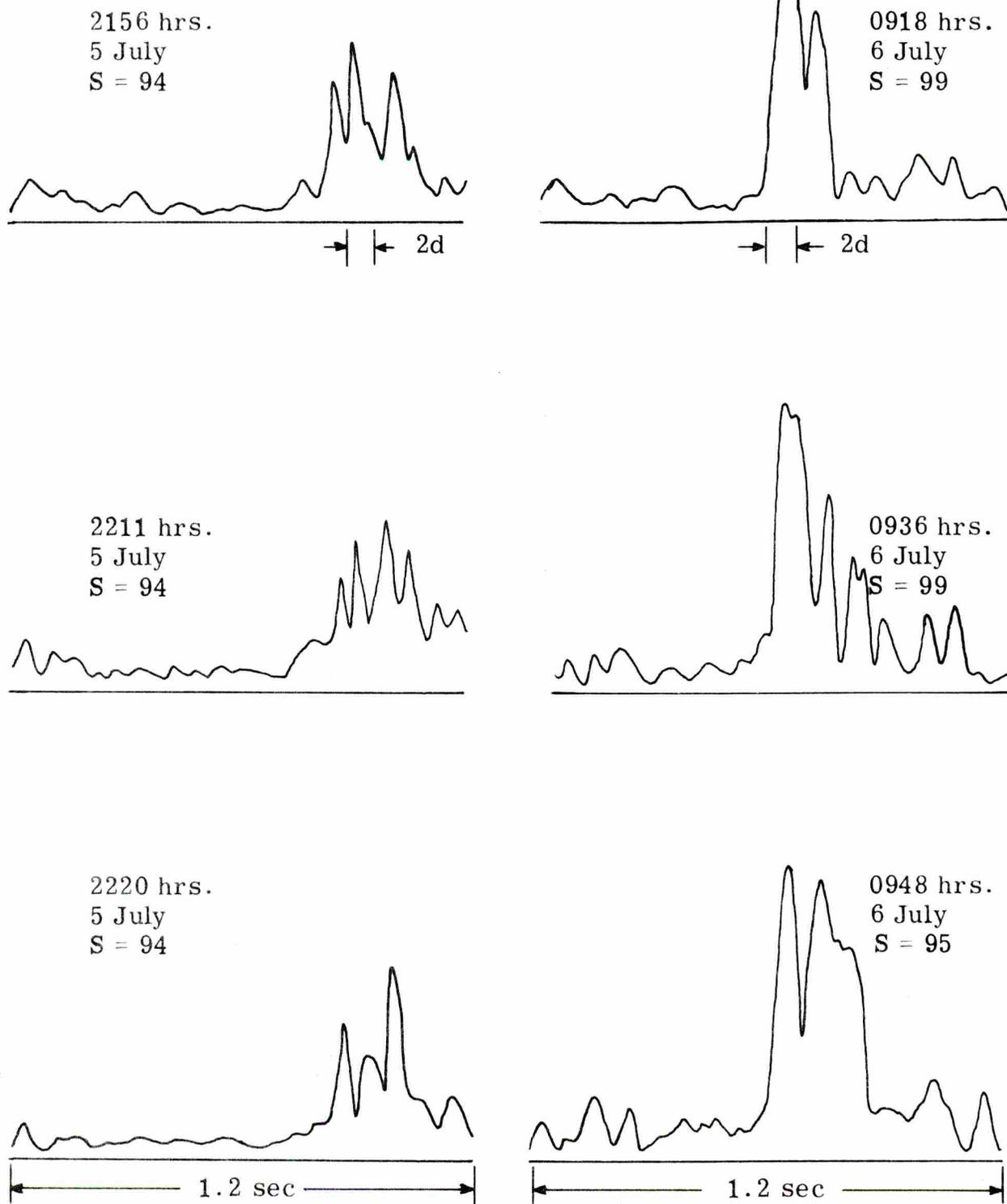
Fig. 18. Multipath displays from the Bimini hydrophone taken on 5-6 July 1970
