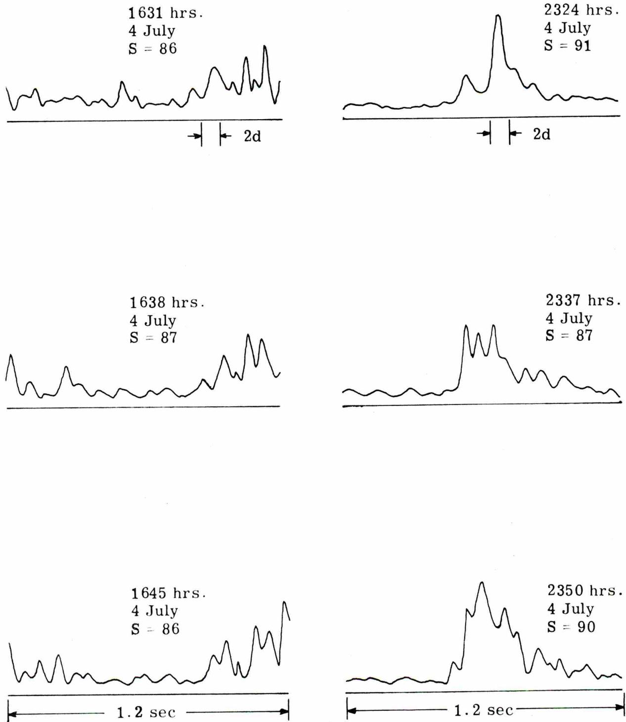
Fig. 16. Multipath displays from the Bimini hydrophone taken on 4 July 1970
