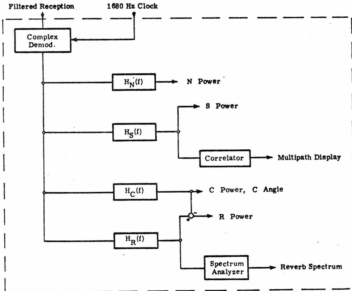
Fig. 10. Block diagram of the digital processing implementation
