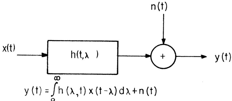
Fig. 2.5. The Linear, Quasi-Stationary UWAP Channel, An Impulse Response Representation
