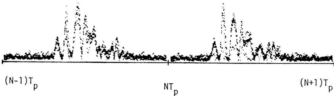
Fig. 2. 14. Typical Multipath (Or Delay Spread) Reception
