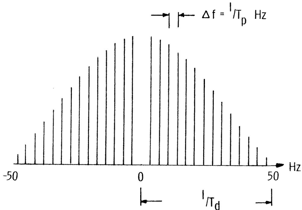
Fig. 2.11. The Multipath Measurement Signal Spectrum
