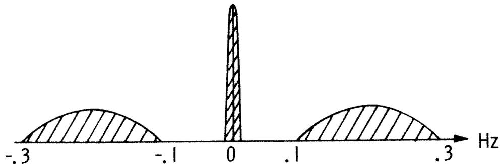
Fig. 2.6. Frequency Spreading of the UWAP Channel, Observed Using a CW Transmission
