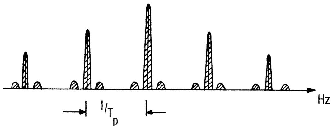
Fig. 2. 13. Received Frequency Spread Line Spectrum
