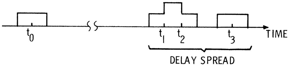
Fig. 2.7. Arrivals at  $t_1$ ,  $t_2$ , and  $t_3$  from a Single Pulse Transmission at  $t_0$  Illustrate the Multipath Structure (Delay Spread) of the Channel
