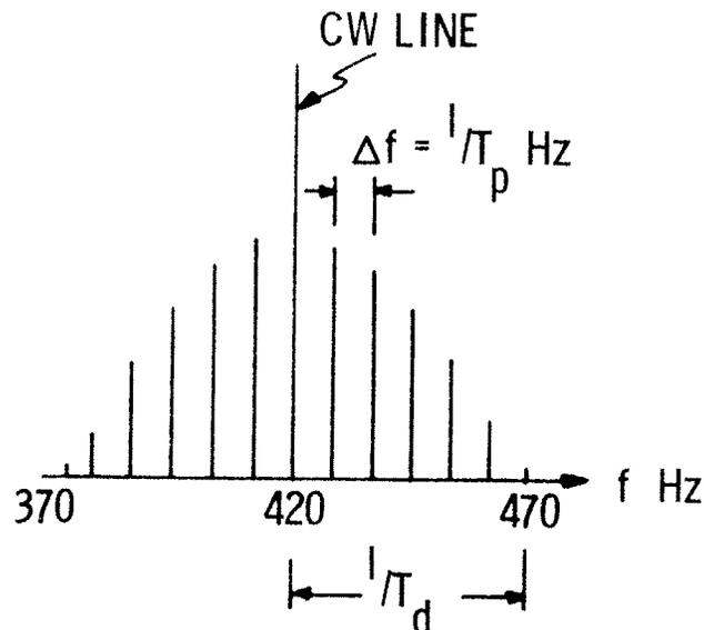
Fig. 2.4. Magnitude Spectrum of the MIMI CM Signal
