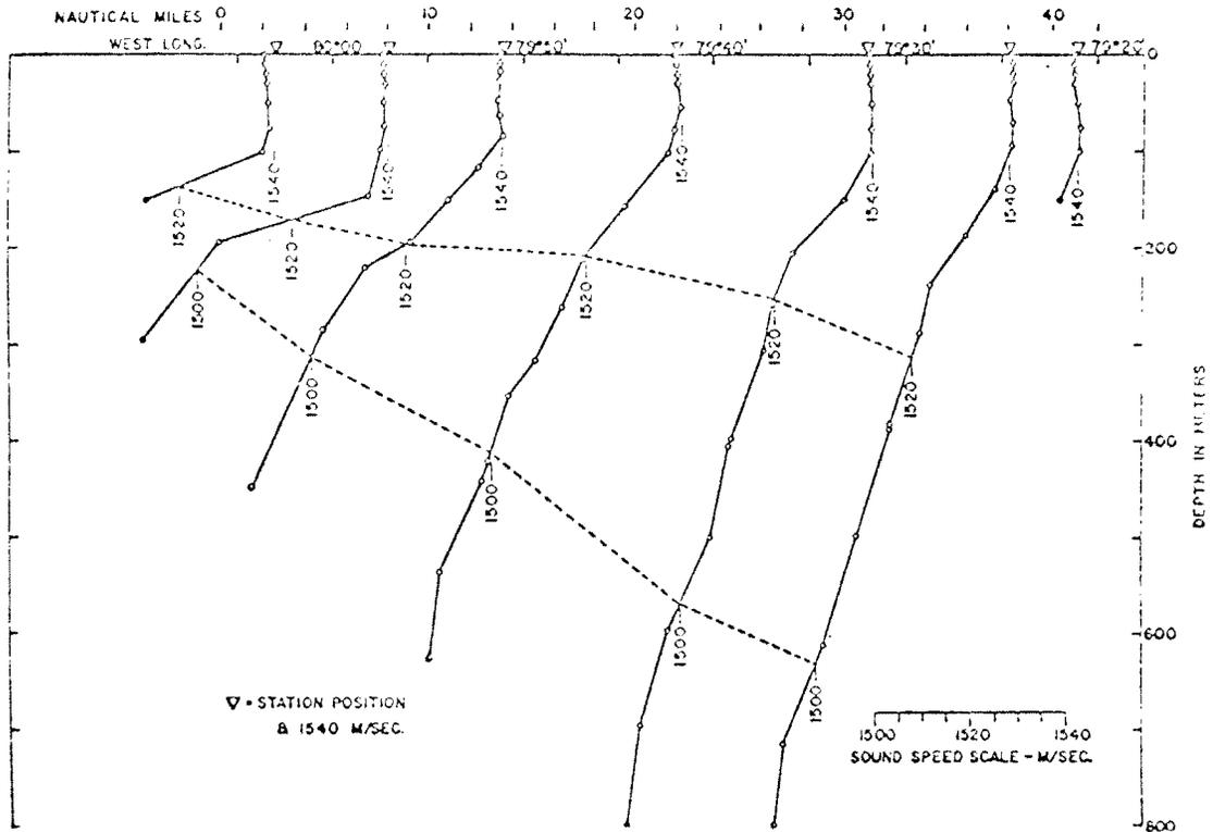
Fig. 2.2. Sound Speed vs. Depth
