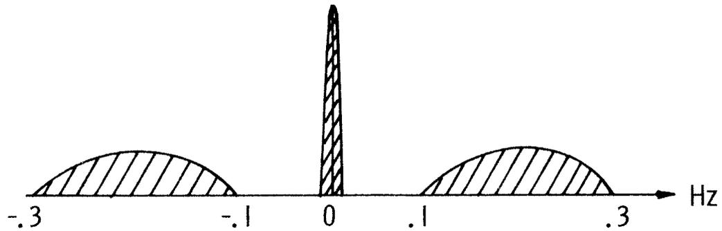
Fig. 2.10. CW Reception Magnitude Spectrum Demodulated
