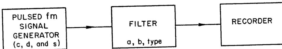
Fig. 4.1 Block diagram of differential analyzer.
