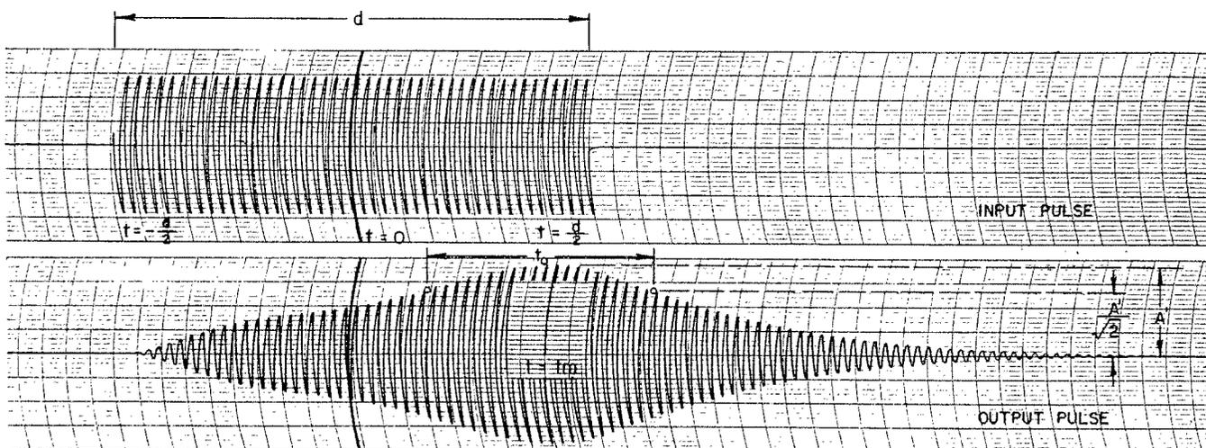
(a) INPUT AND OUTPUT PULSES FOR A TWO CIRCUIT FILTER
