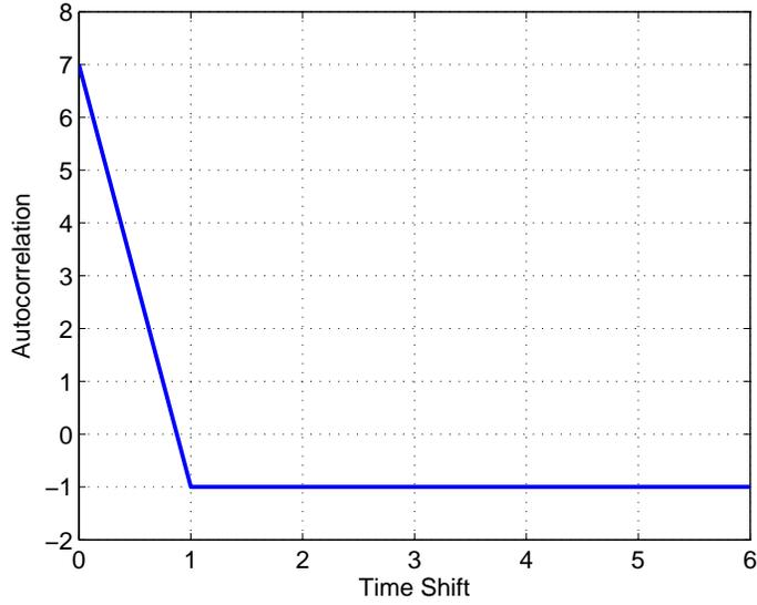
Figure 5.3: Autocorrelation function of modulation sequence
